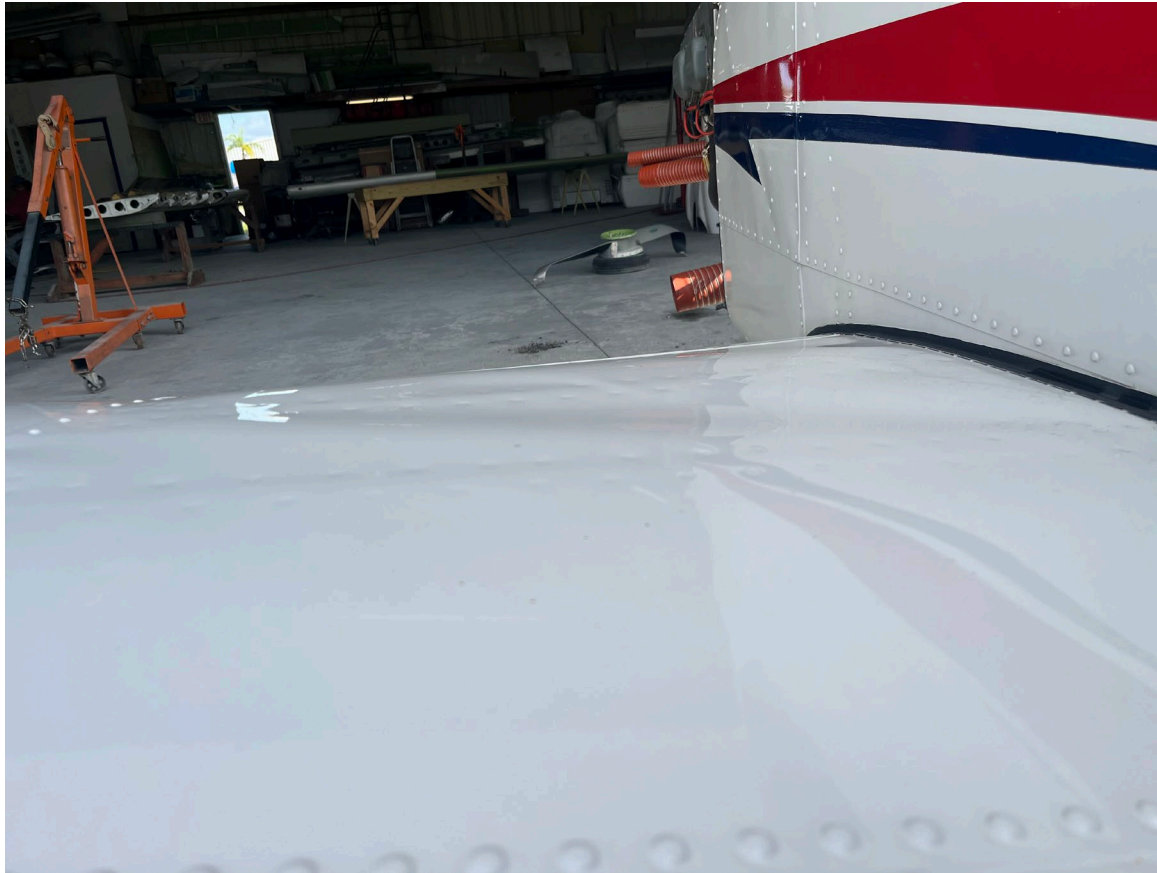
Photograph 3 - Left Wing Spar Damage (Courtesy of FAA)
