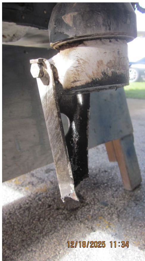
Photograph 4 - Nose Landing Gear Damage (Courtesy of FAA)
