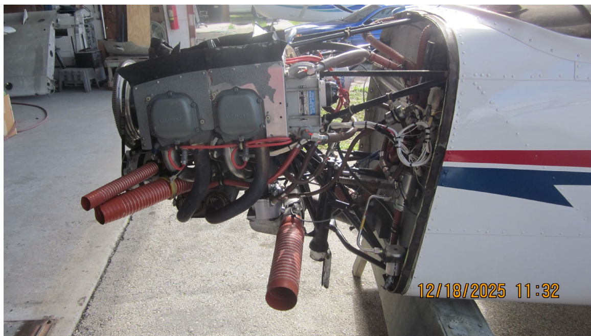
Photograph 2 - Engine Mount Damage (Courtesy of FAA)
