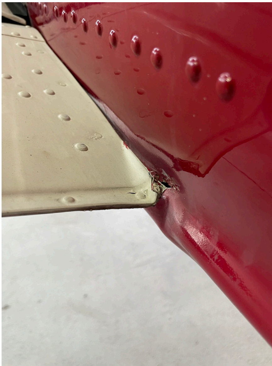
Photograph 3 - Left Wing Spar Damage (Courtesy of FAA)
