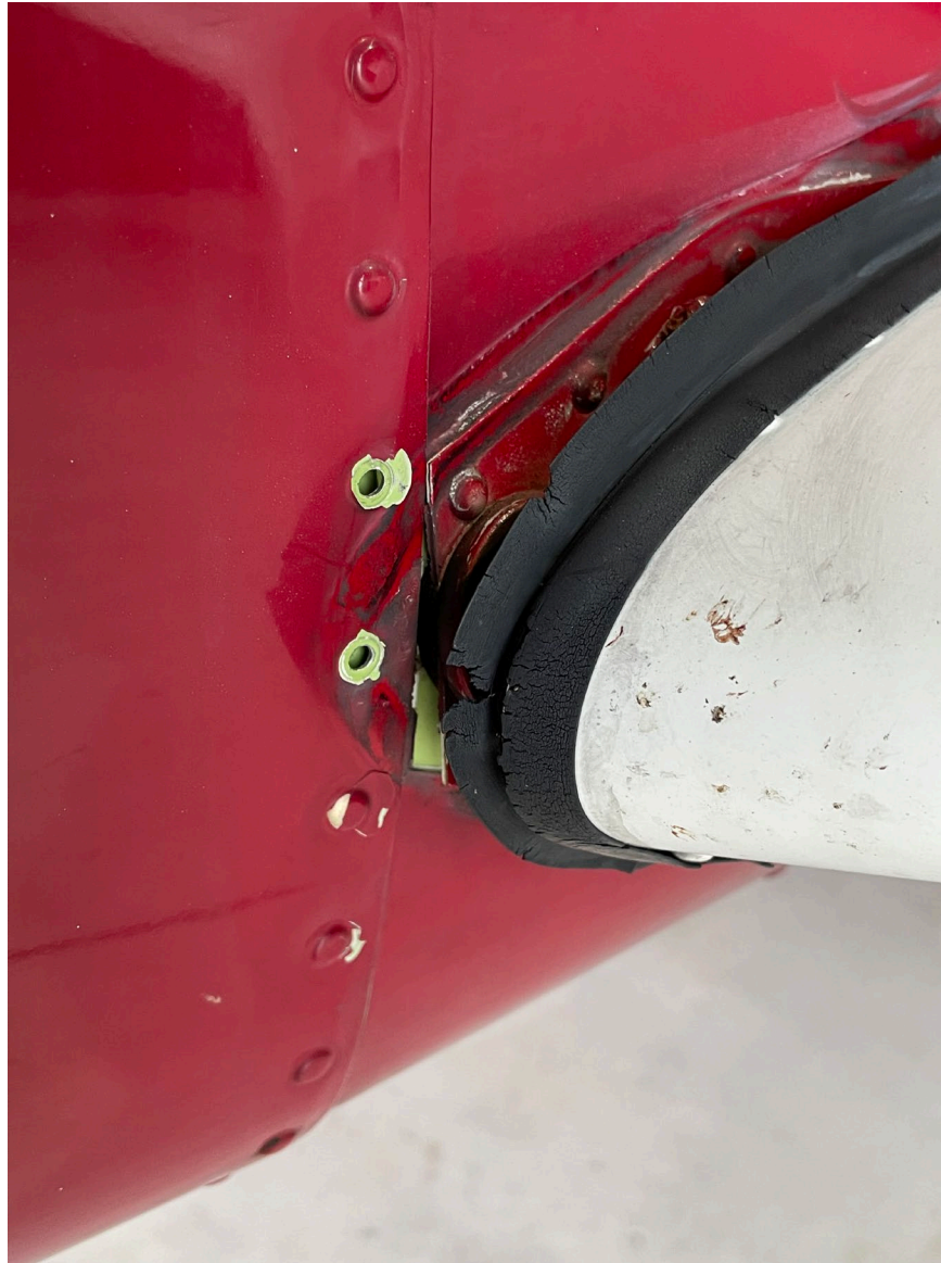
Photograph 1 - Left Wing Spar Damage (Courtesy of FAA)
