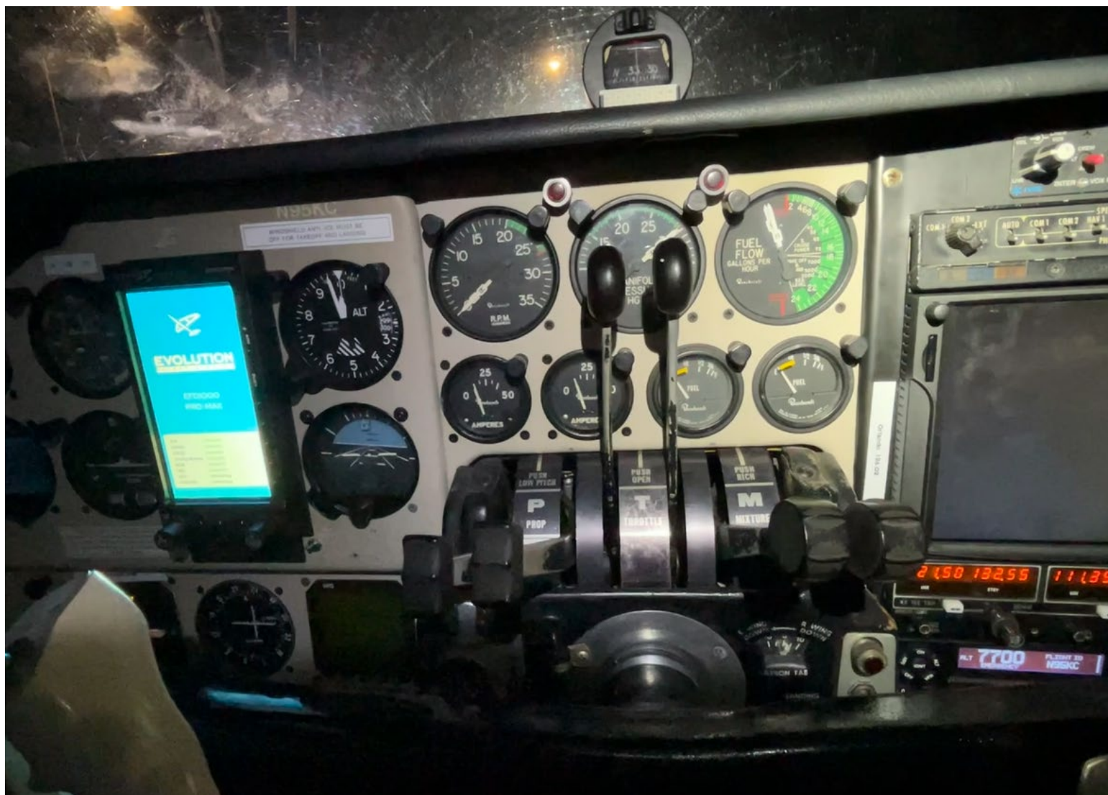
Photograph 2 - Fuel Needle Gauges with the Airplane Power On (Courtesy of FAA)
