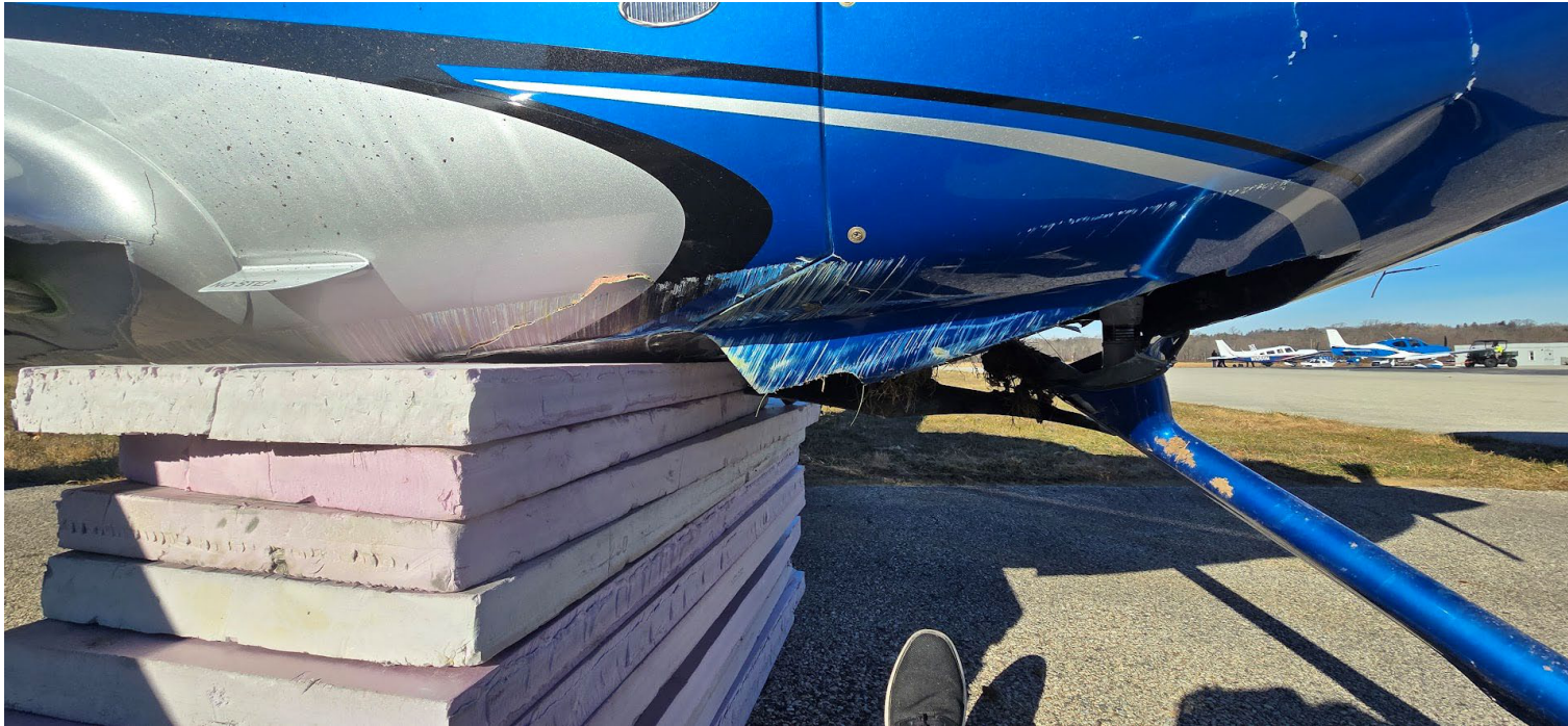
Photograph 2 - Lower fuselage Damage (Courtesy of FAA)
