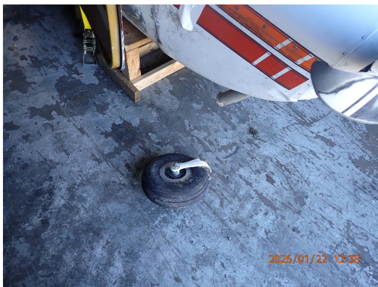
Photo 10: View of the nose landing gear that was impact separated.
