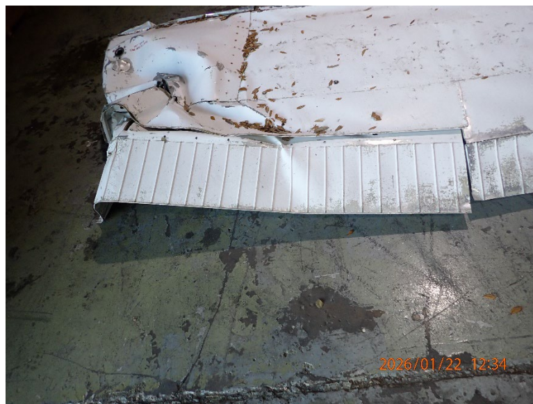
Photo 6: Damage to right wing root
