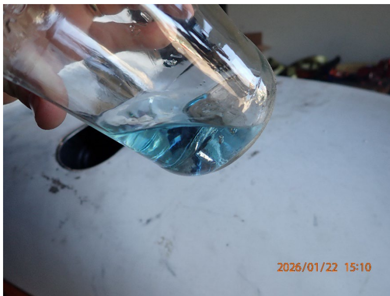
Photo 14: Fuel drained from strainer
