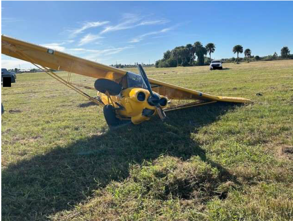
Photograph 2 - Right-hand front view showing damage to landing gear (Courtesy of Airport Authority)
