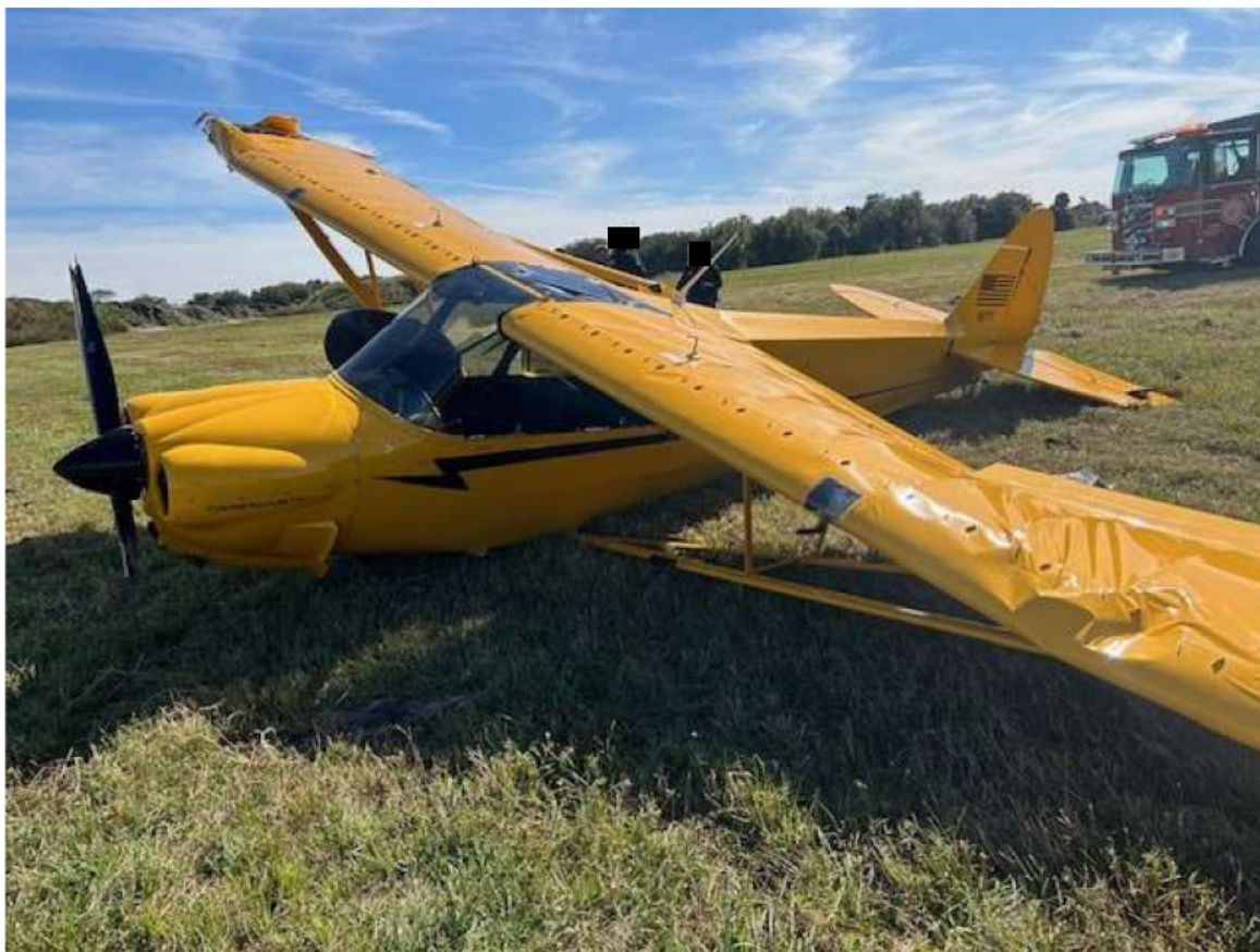
Photograph 1 - Left-hand front view showing damage to wings (Courtesy of Airport Authority)
