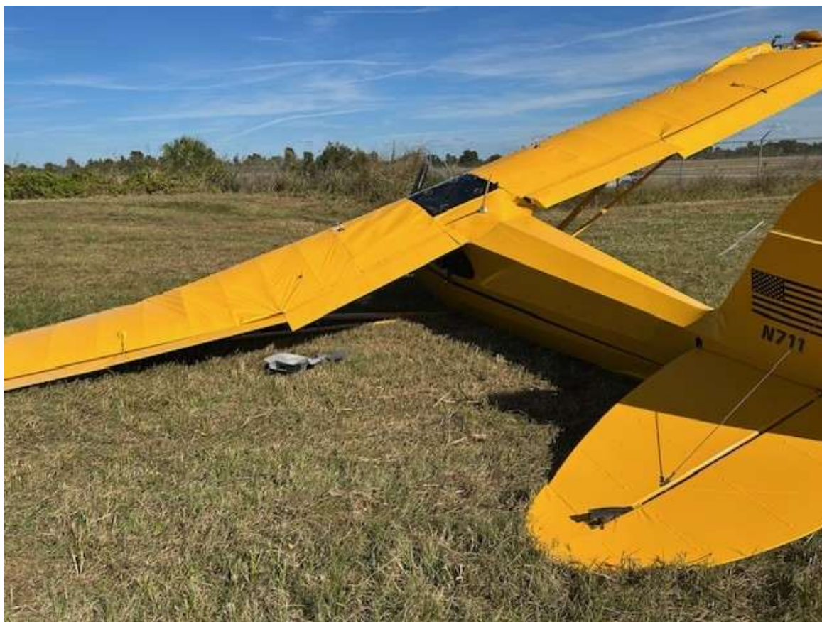
Photograph 4 - Left-hand rear view showing damage to wings (Courtesy of Airport Authority)
