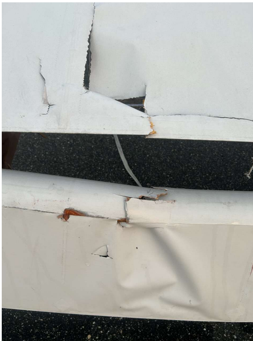
Photograph 2 - Closeup of damage to left wing and aileron (Courtesy of FAA)
