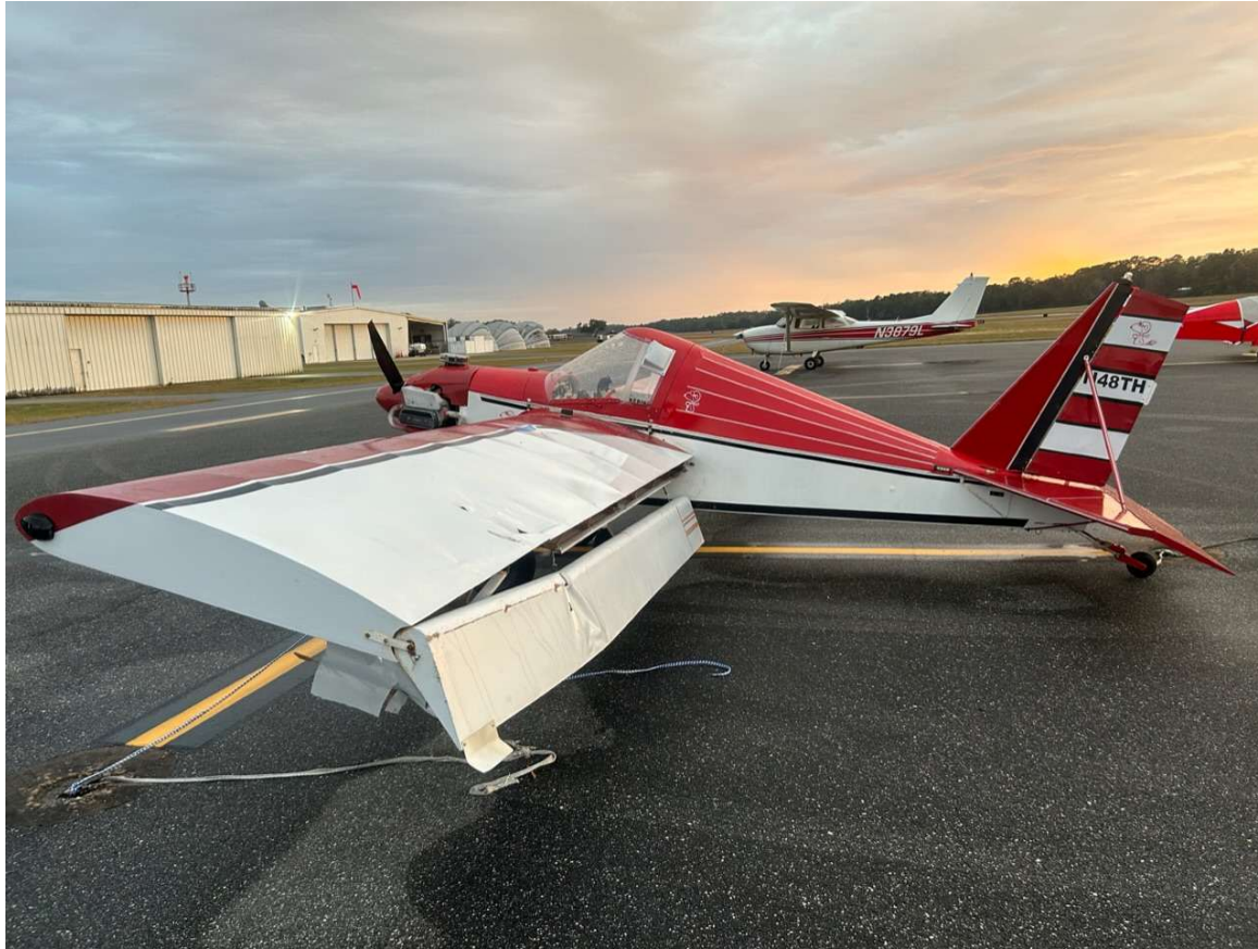
Photograph 1 - Left Side View showing damage to wing and aileron (Courtesy of FAA)
