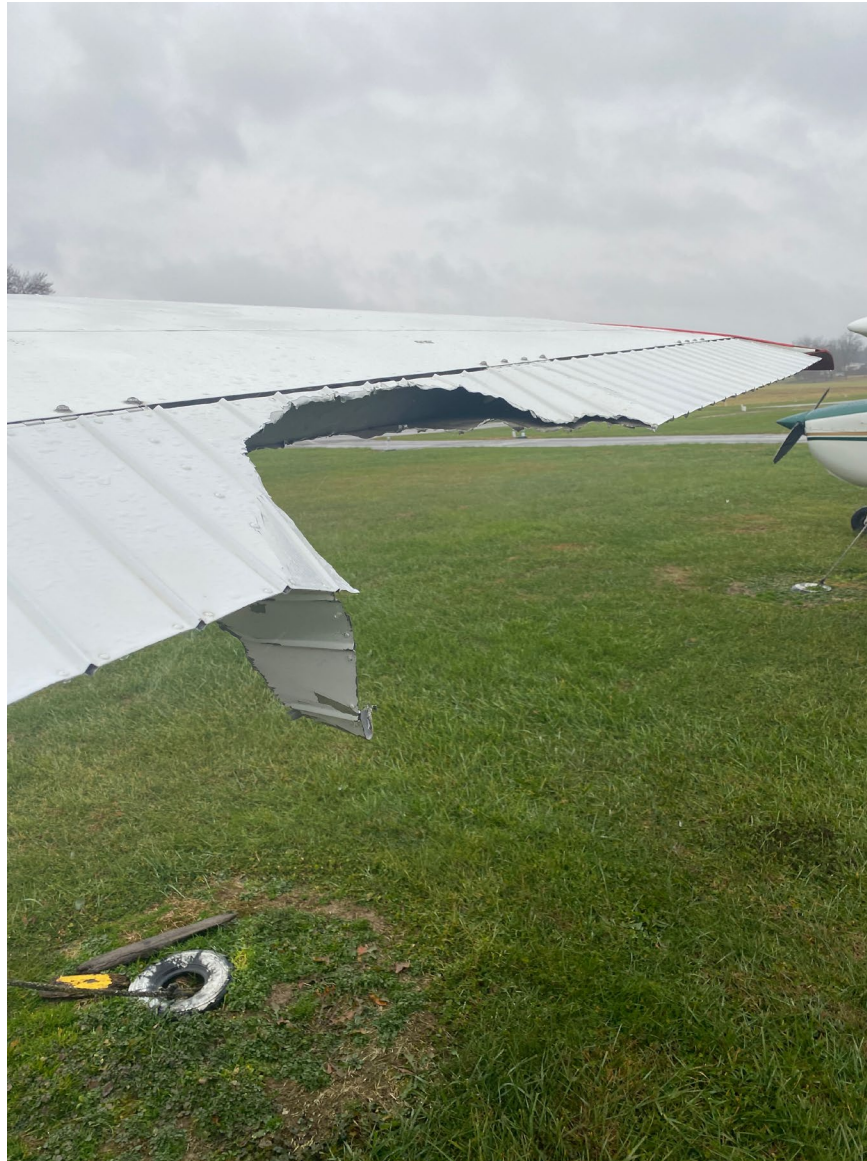
Photograph 2 - Right Aileron Damage (Courtesy of FAA)
