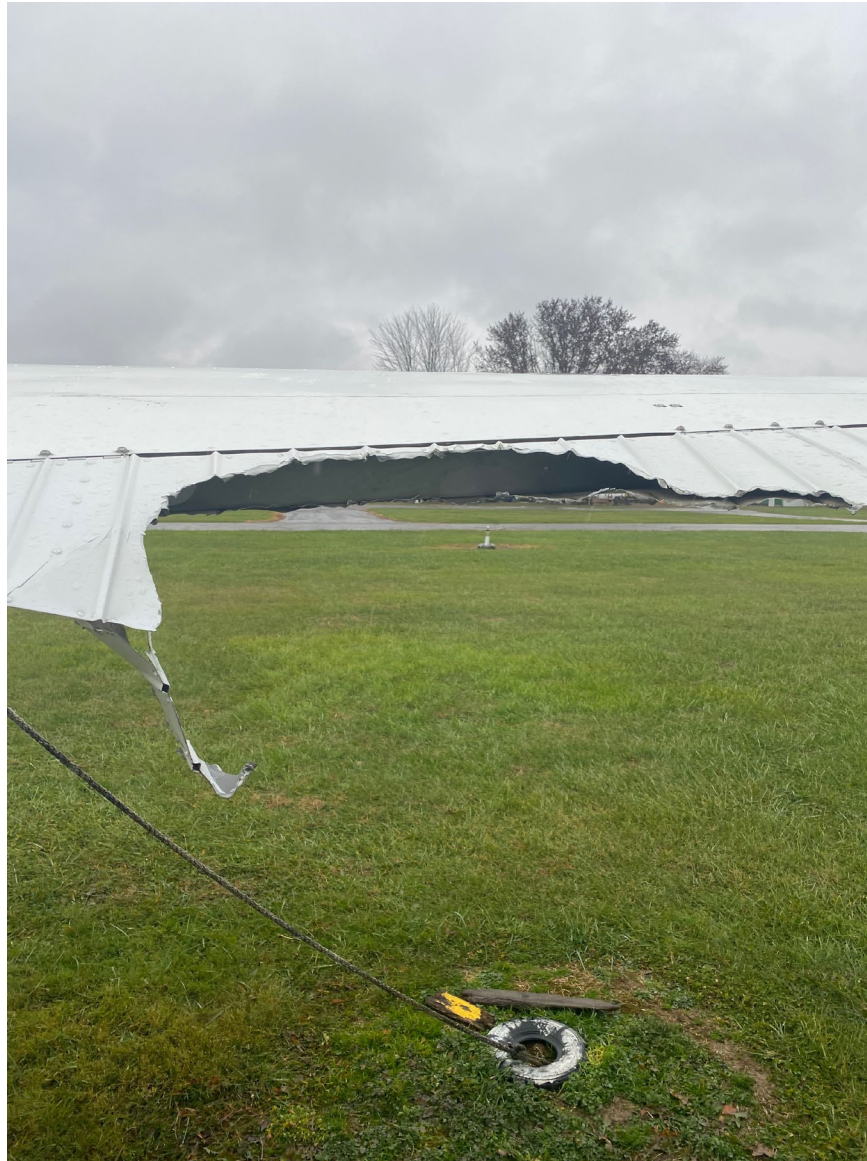
Photograph 3 - Right Aileron Damage (Courtesy of FAA)
