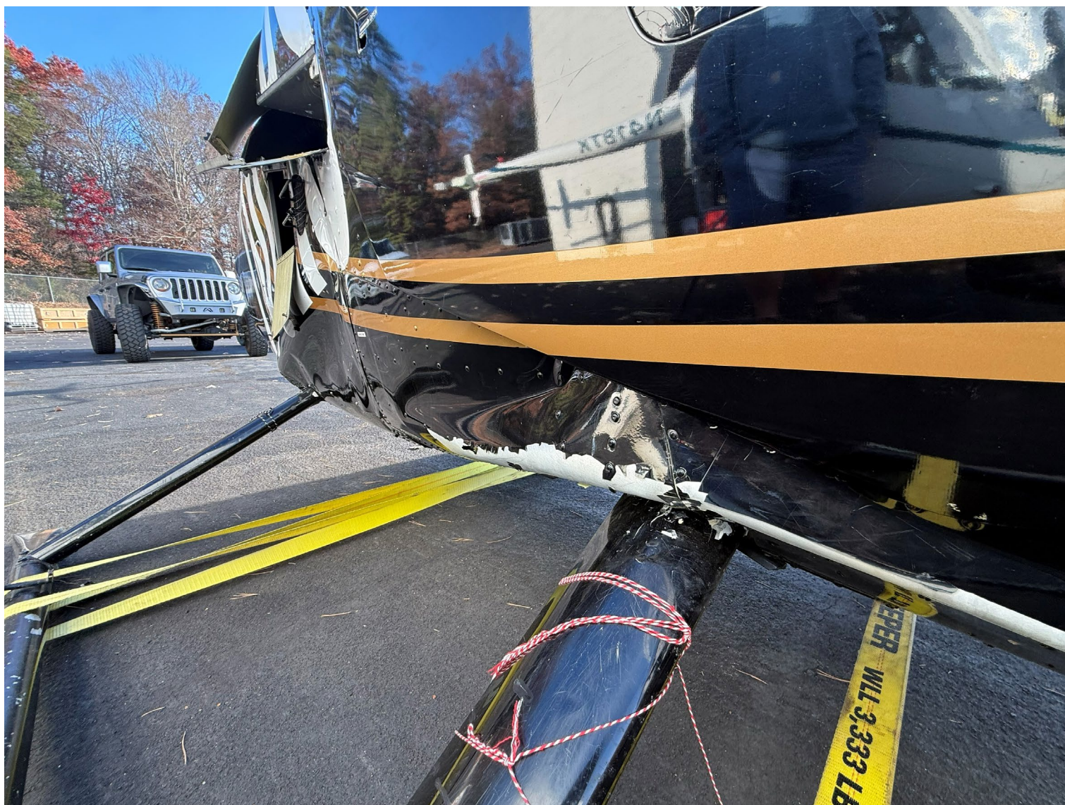
Photograph 2 - skid damage, fuselage damaged (Courtesy of FAA)
