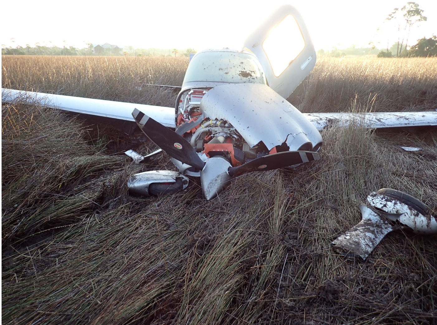
Photograph 2 - Airplane Forward Fuselage Damage and Broken Landing Gear (Courtesy of Cirrus Aircraft)
