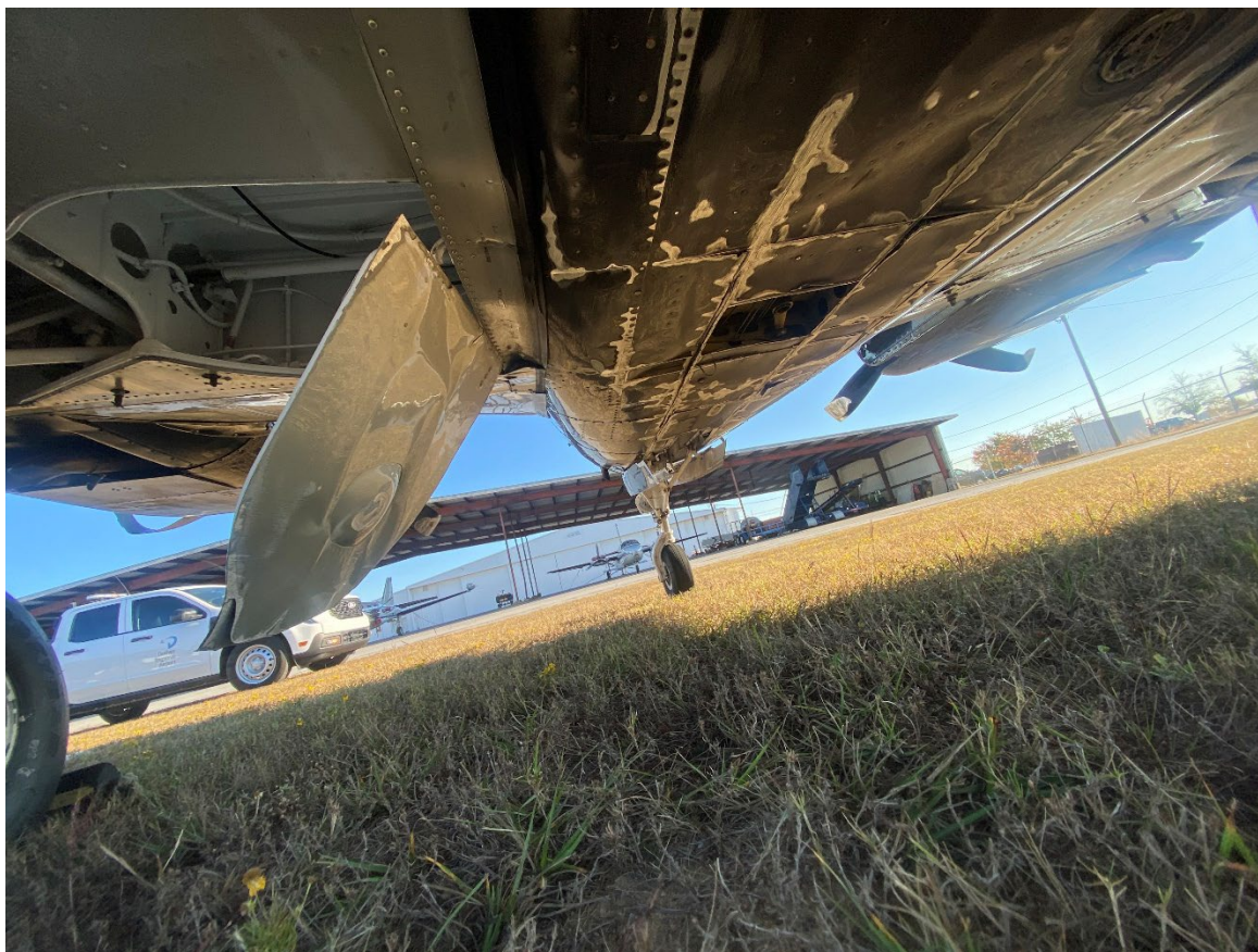
Photograph 3 - Abrasion Damage to Fuselage(Courtesy of Dothan Airport)
