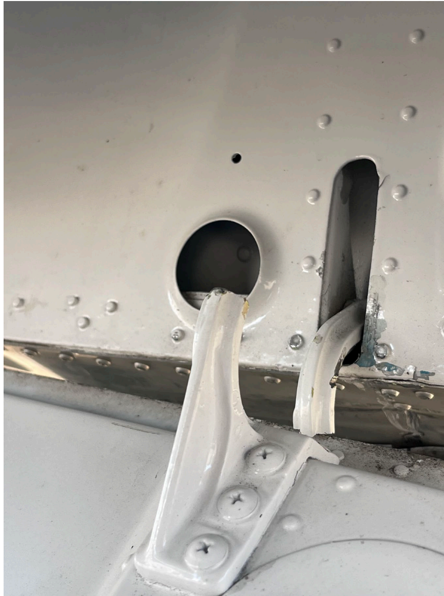
Photograph 5 - Failed Left Aft Inboard Door Hinge (Courtesy of Airplane Owner)
