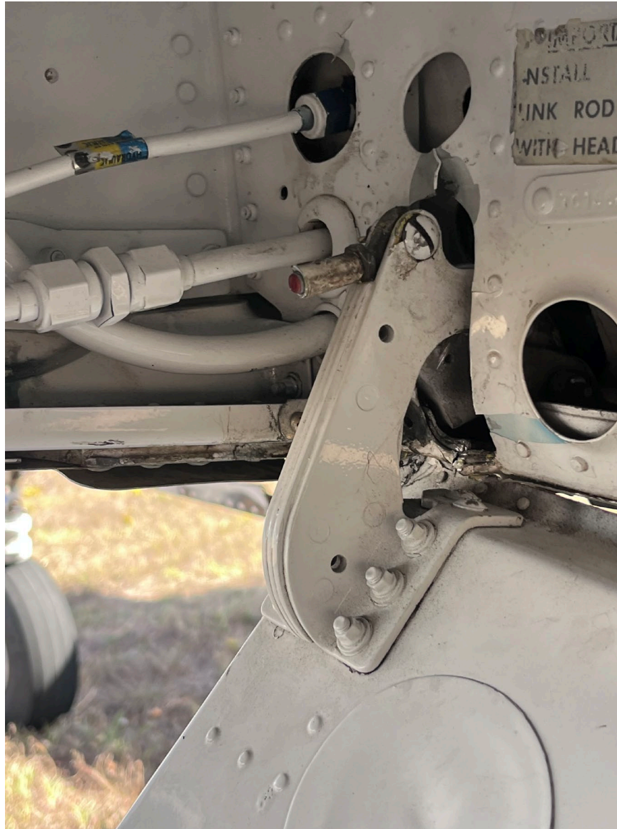
Photograph 4 - Failed Left Inboard Gear Door Link Assembly (Courtesy of Airplane Owner)
