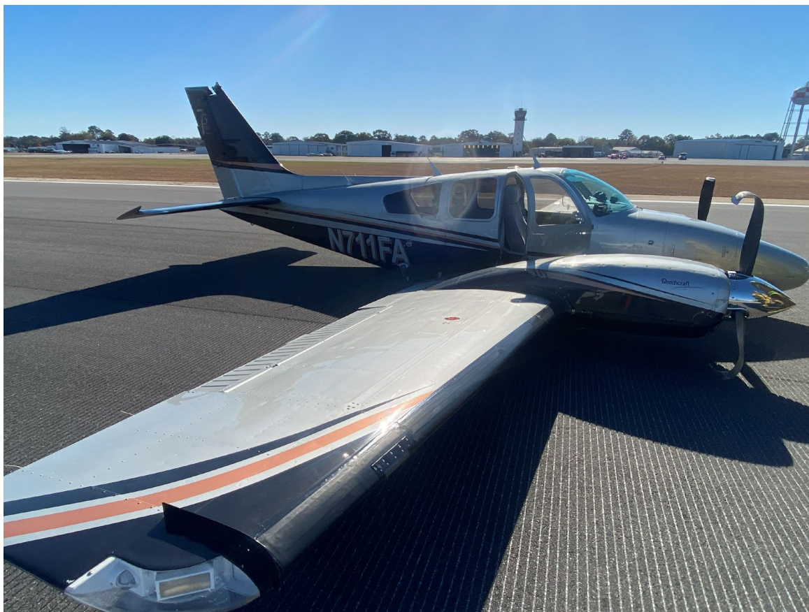
Photograph 1 - N711FA After Landing with Landing Gear Retracted (Courtesy of Dothan Airport)
