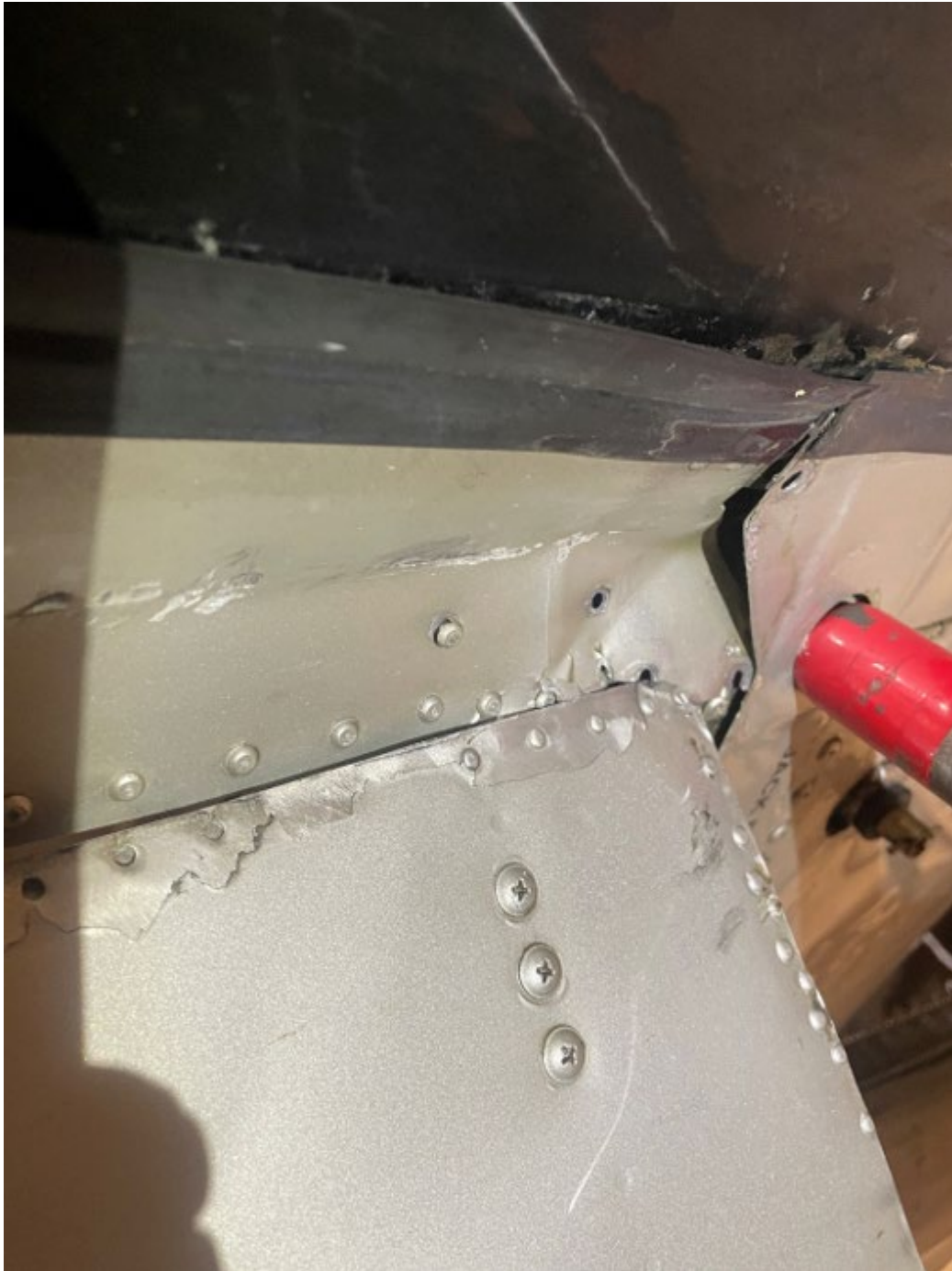
Figure 3: Abrasion Damage on Underside of Inboard Left Main Gear Door
