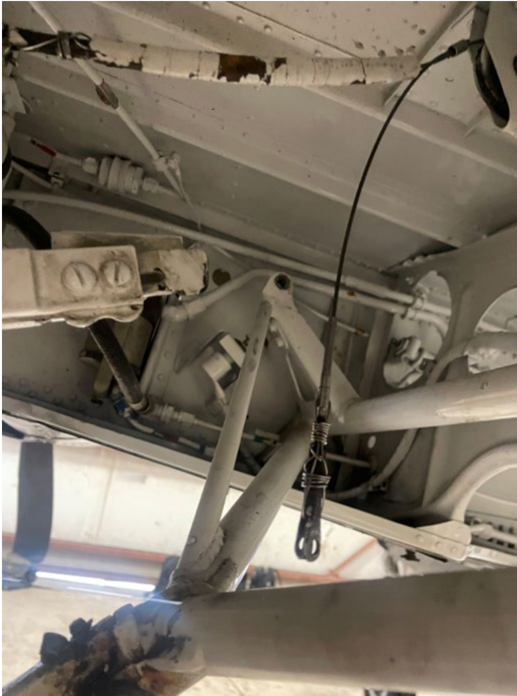
Figure 11: Left Main Gear Well, After Removal of Main Retraction Rod and Detachment of Downlock Cable
