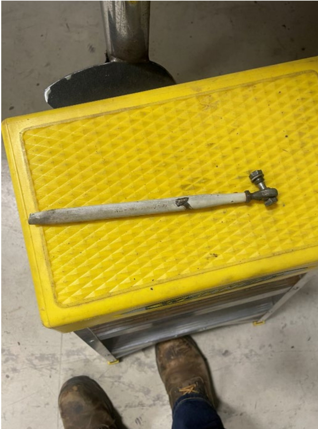
Figure 5: Rod Portion of Failed Left Main Gear Door Link Assembly
