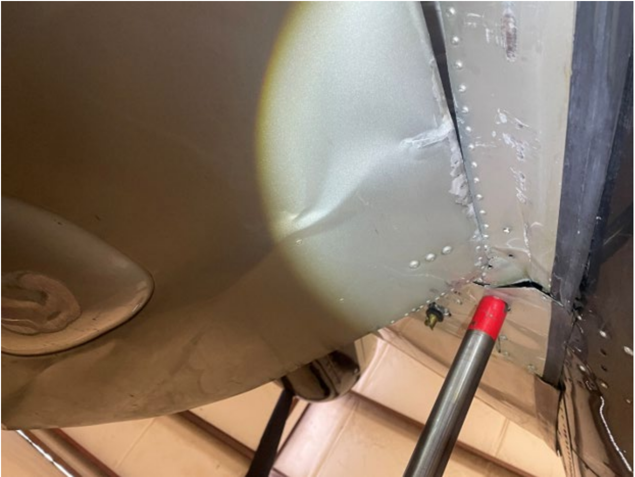
Figure 2: Underside of Inboard Left Main Gear Door
