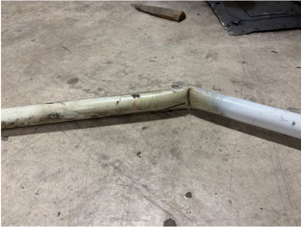
Figure 8: Buckled Main Gear Retraction Rod Assembly After Removal
