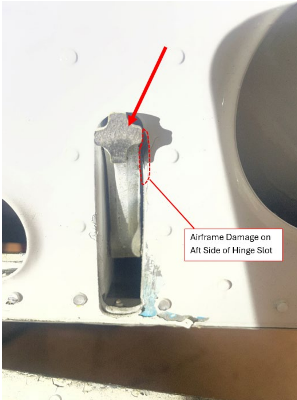
Figure 6: Failed Left Main Landing Gear Door Aft Inboard Hinge
