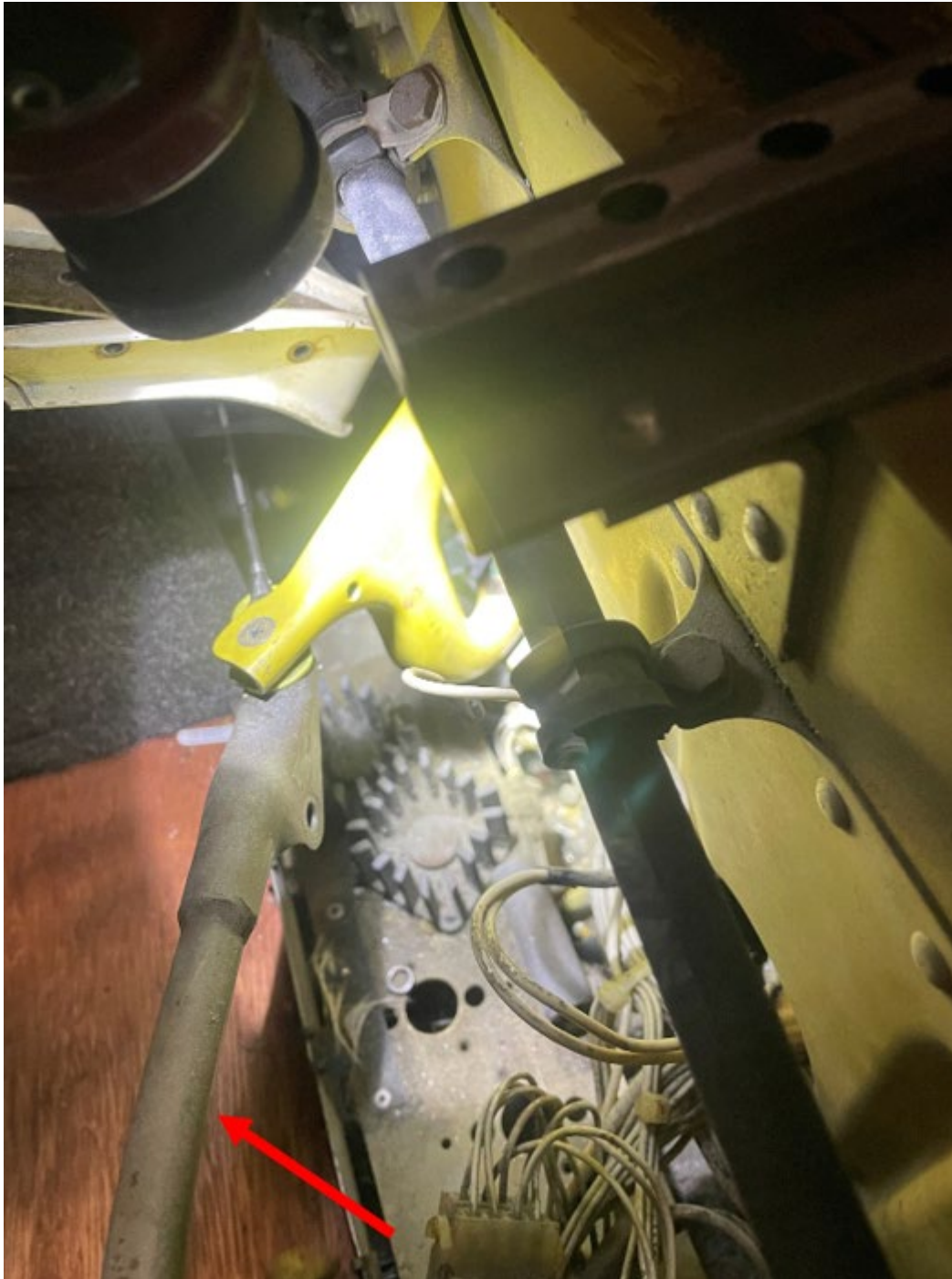
Figure 9: Bent Left Main Landing Gear Door Actuator Rod Assembly
