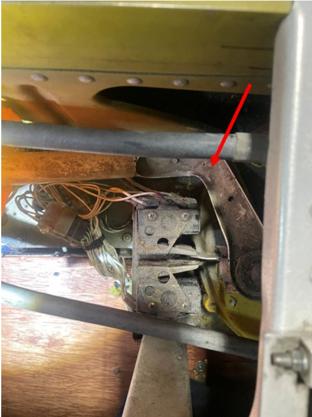
Figure 7: Bent Left Main Gear Retraction Rod Assembly
