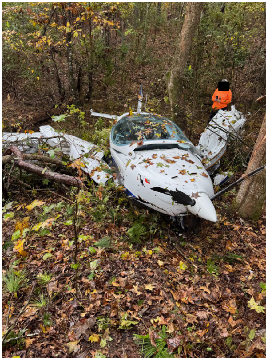
Photograph 2 - View from the Nose with Wing Damage (Courtesy of FAA)
