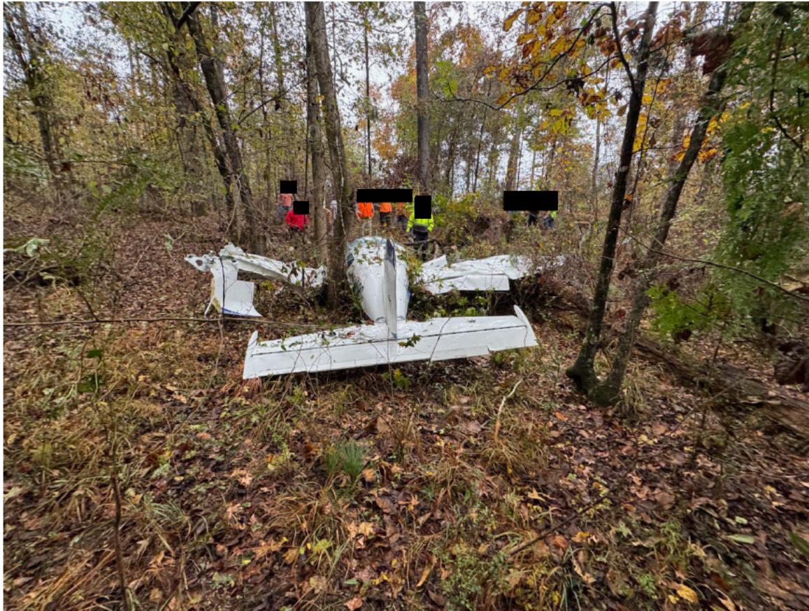
Photograph 3 - Aft View with Wing Damage (Courtesy of FAA)
