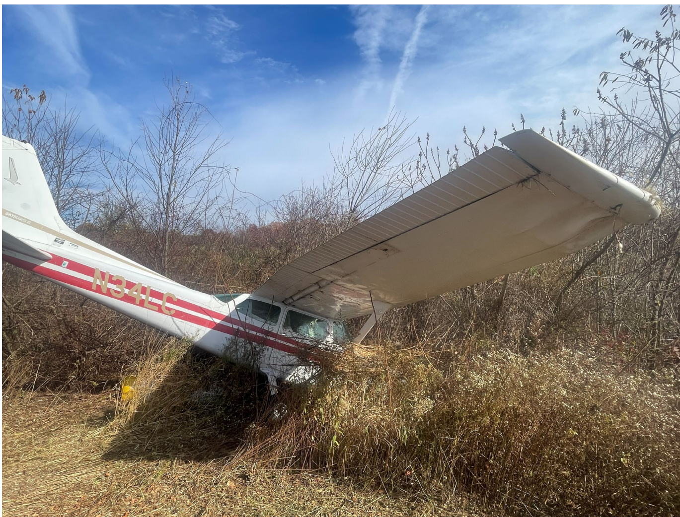
Photograph 2 - Outboard Right Wing Leading Edge Damage with Brush (Courtesy of FAA)
