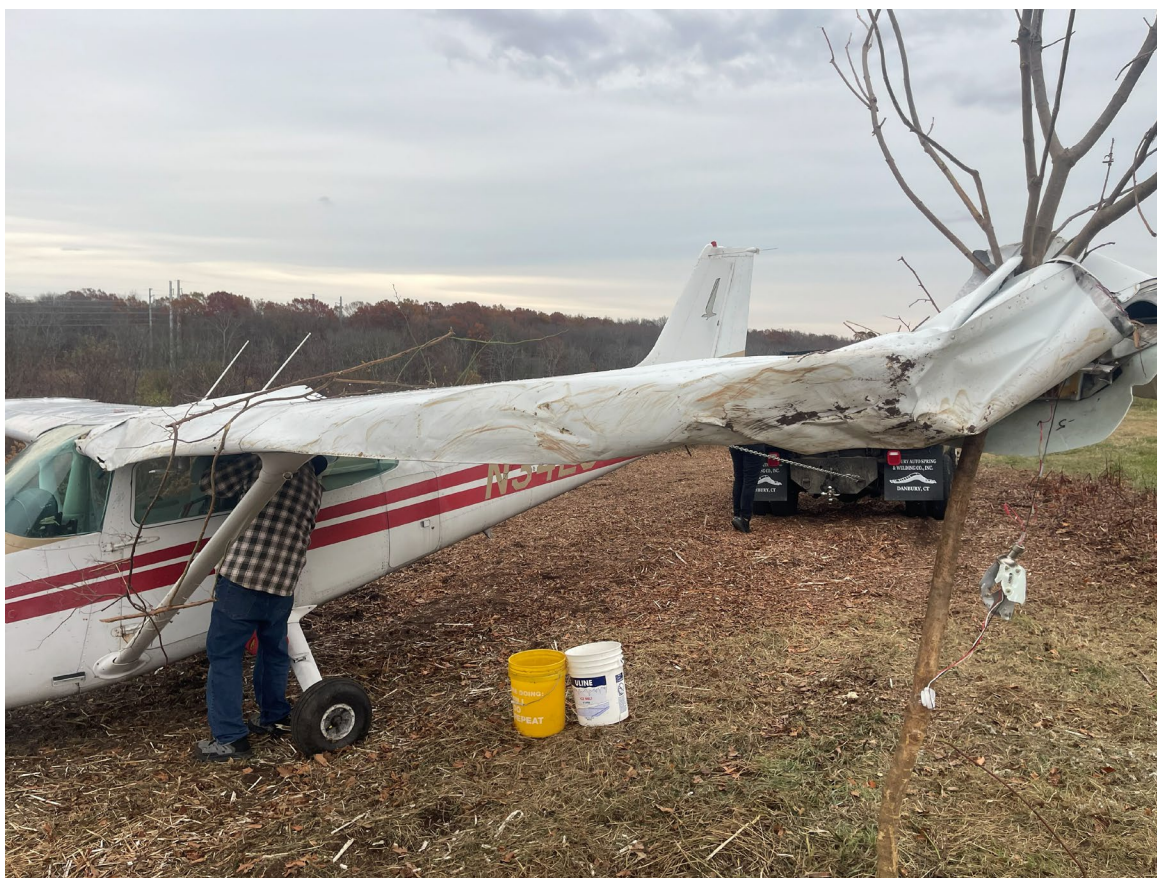
Photograph 3 - Left Wing Leading Edge Damage (Courtesy of FAA)
