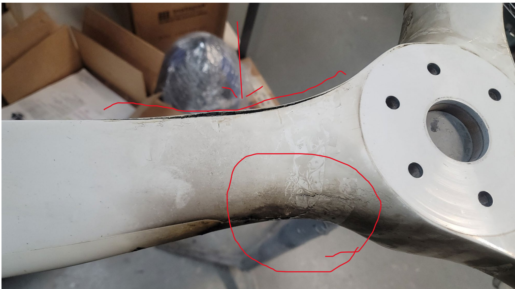
Photograph 4 - Photo of propeller after the accident showing delamination (Courtesy of Catto Propellers)
