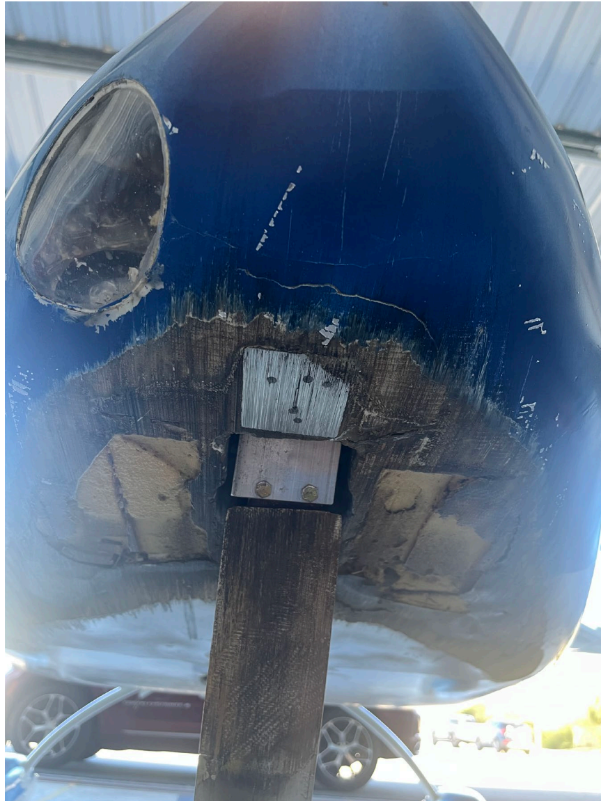
Photograph 2 - Photo showing substantial damage to the composite structure of the lower nose (Courtesy of owner)
