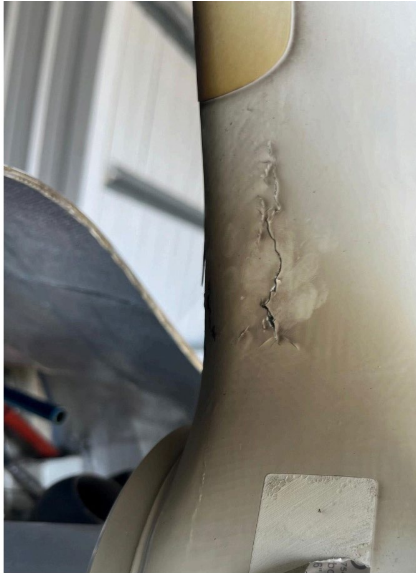
Photograph 5 - Photo of damage to propeller as reported to manufacturer May, 2025 (Courtesy of Catto Propellers)
