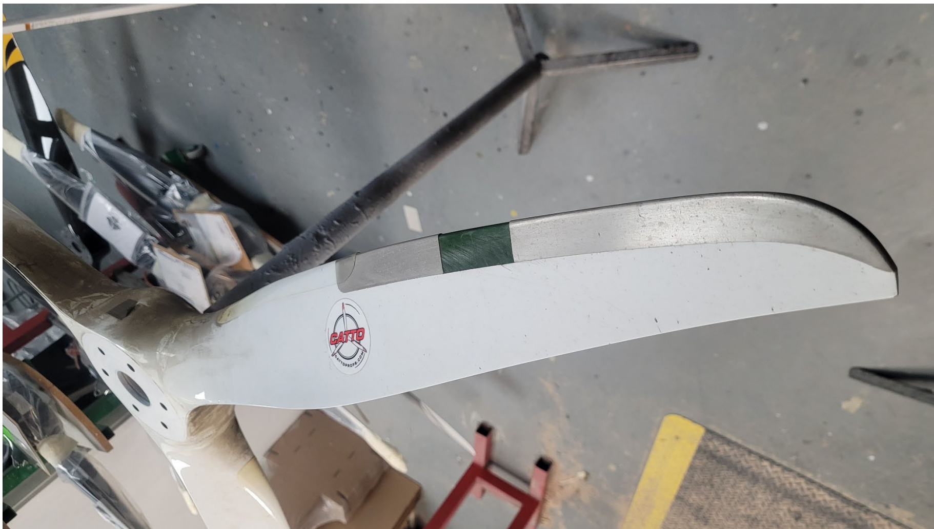
Photograph 3 - Photo of prop blade after accident with missing nickel leading edge (Courtesy of Catto Propellers)
