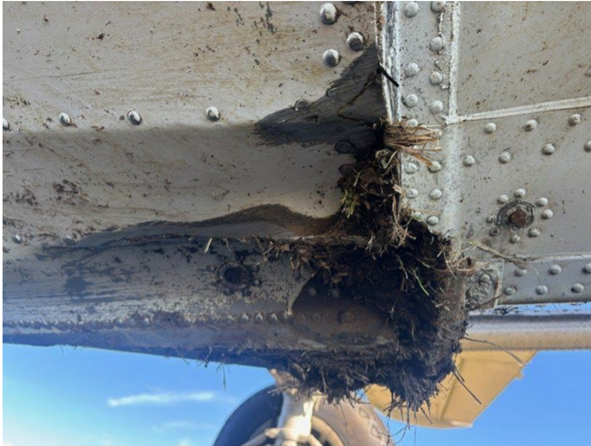
Photograph 5 - Center hull keel damage (Courtesy of Pilot)
