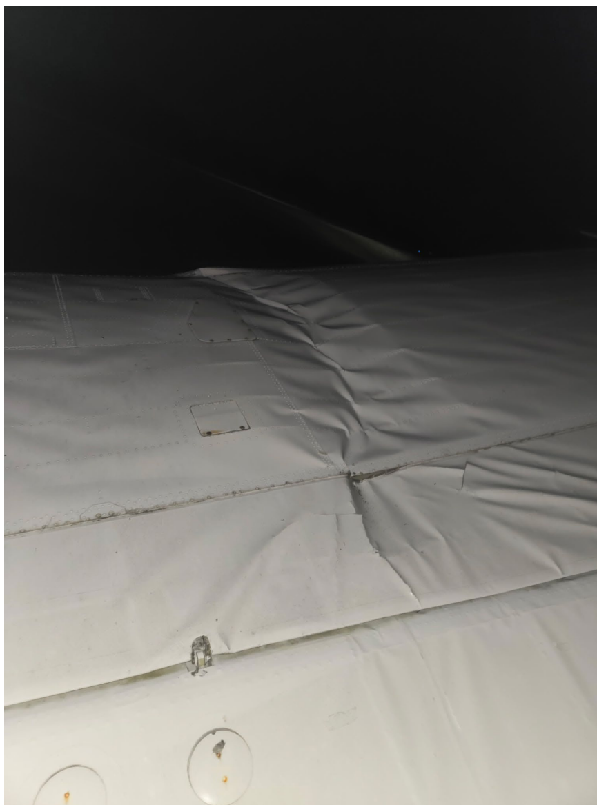
Photograph 2 - Left wing upper skin damage and spar buckling (Courtesy of FAA)
