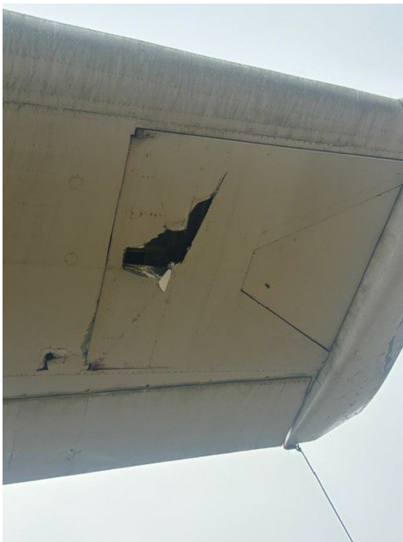
Photograph 4 - Left wing lower skin damage (Courtesy of Pilot)
