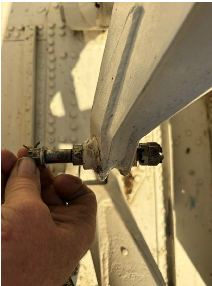
Photograph 6 - Left Main Landing gear sheared actuator bolt (Courtesy of Pilot)
