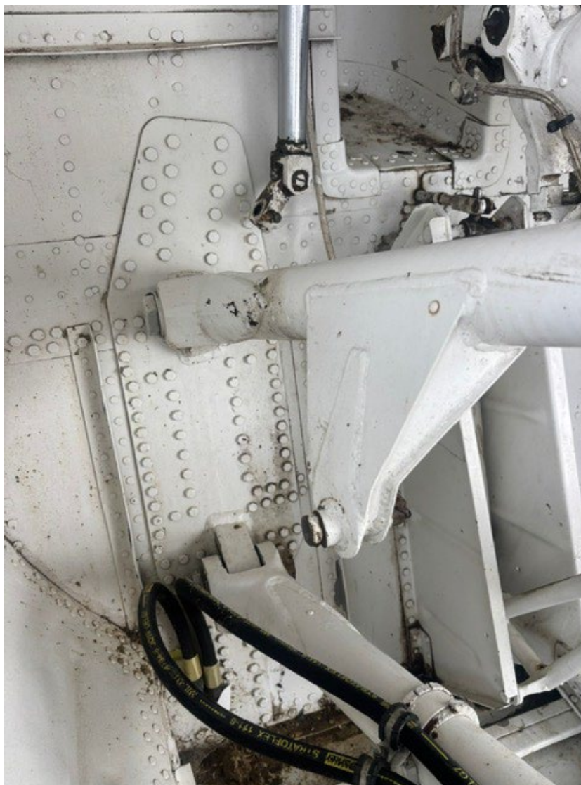
Photograph 7 - Left main landing gear actuator separated from the landing gear assembly. (Courtesy of Pilot)
