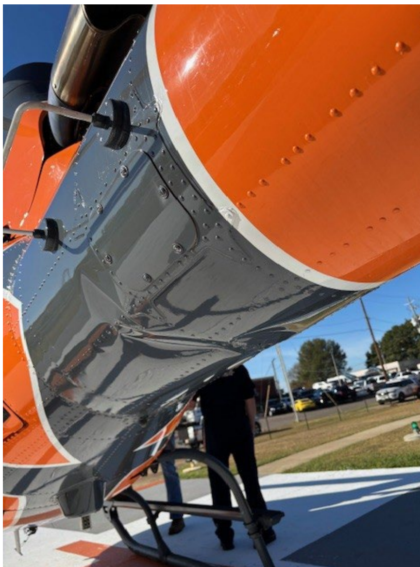
Photograph 1 - Damage to left side of Tail boom (Courtesy of Operator)
