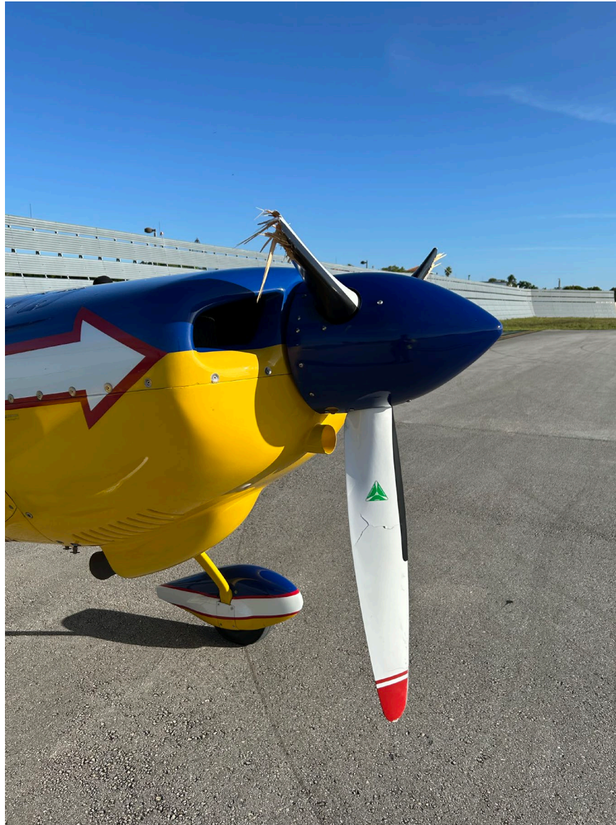
Photograph 5 - N202RD Propeller Damage (Courtesy of Boca Raton Airport)
