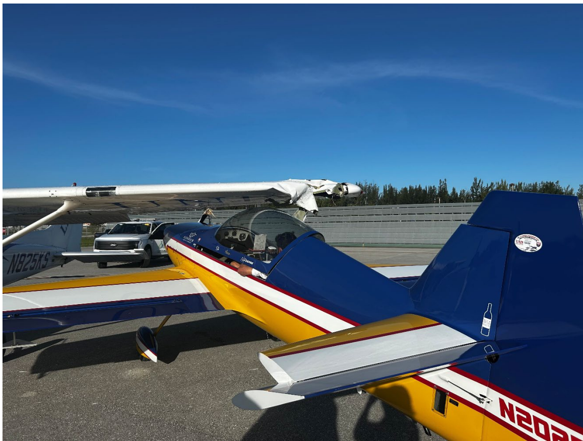
Photograph 2 - Low-Wing Airplane Beneath High-Wing (Courtesy of Boca Raton Airport)
