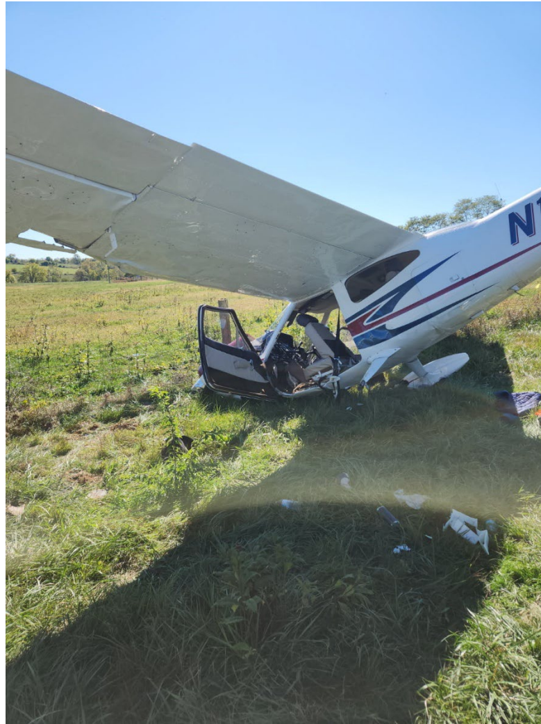
Photograph 1 - Left side view of airplane damage. (Courtesy of FAA)
