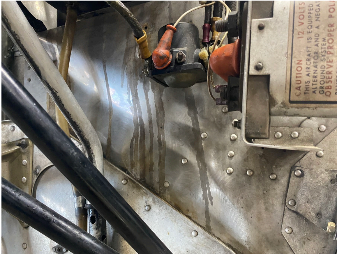
Photograph 2 - Firewall Wrinkling (Courtesy of FAA)
