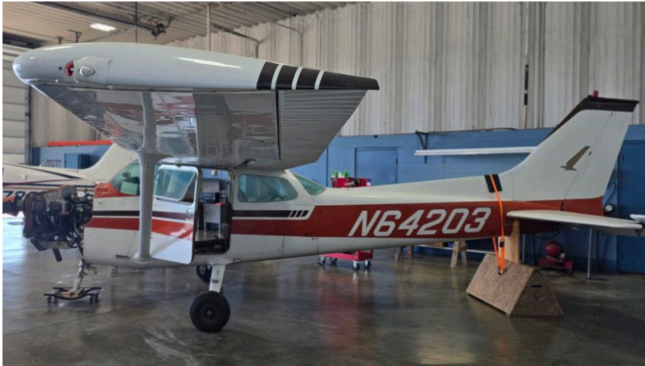
Photograph 1 - Front End Damage on Accident Aircraft (Courtesy of FAA)
