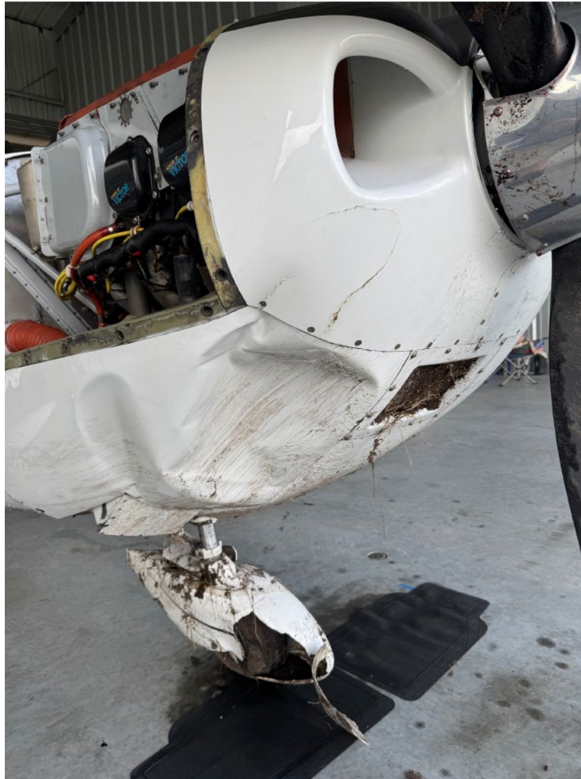
Photograph 1 - View of right-hand side of aircraft nose showing impact damage (Courtesy of Maintenance Facility)
