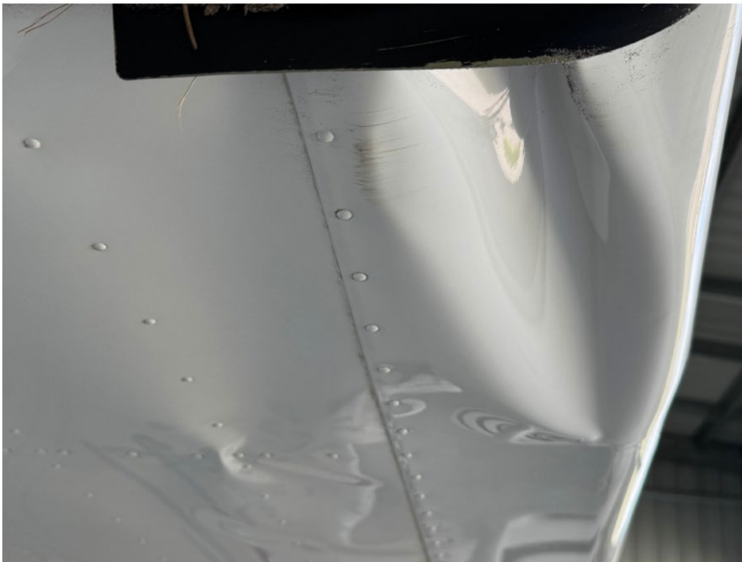
Photograph 4 - View of right-hand wing showing leading edge and spar damage (Courtesy of Maintenance Facility)
