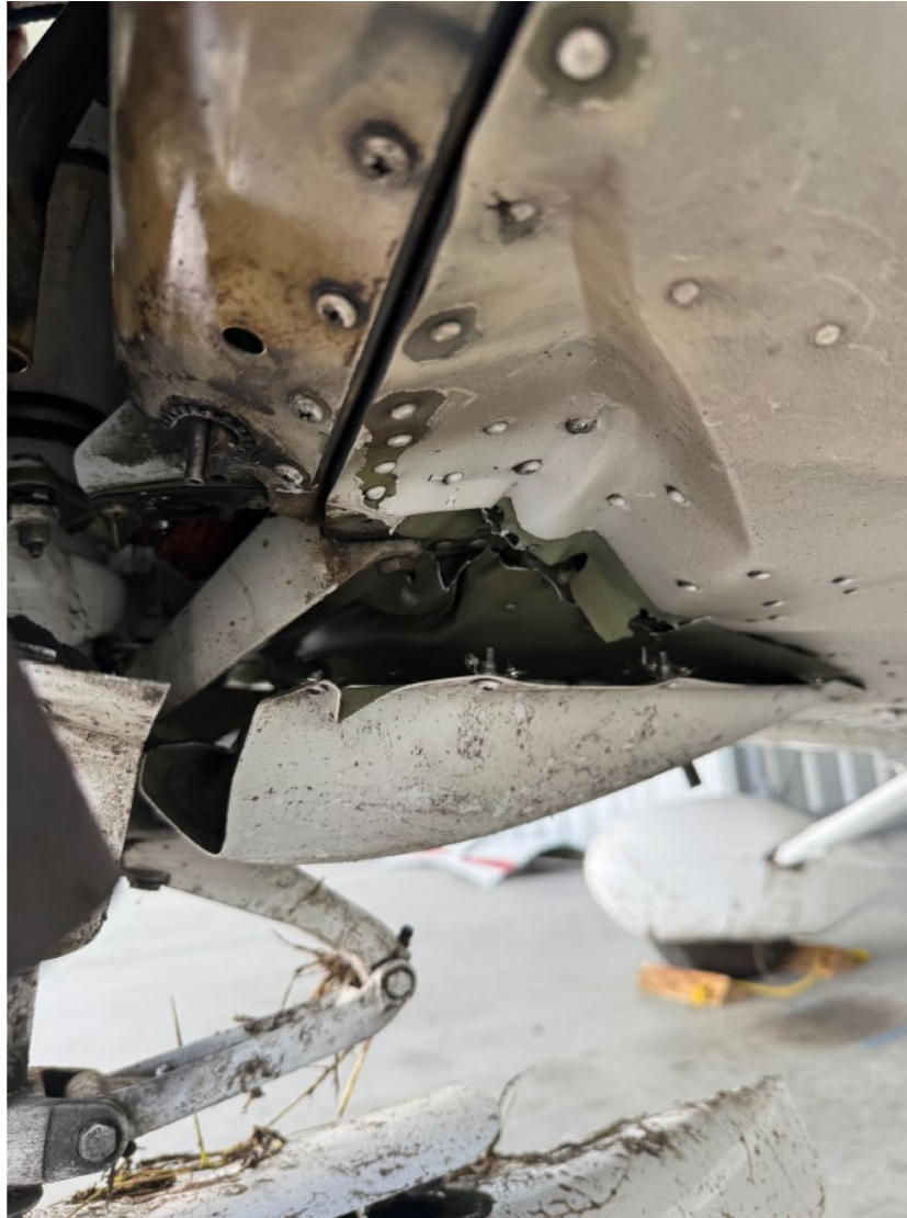
Photograph 2 - View of underside of fuselage behind firewall showing substantial damage (Courtesy of Maintenance Facility)
