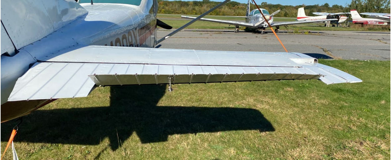
Trim tab with control wheel in the nose up position.
