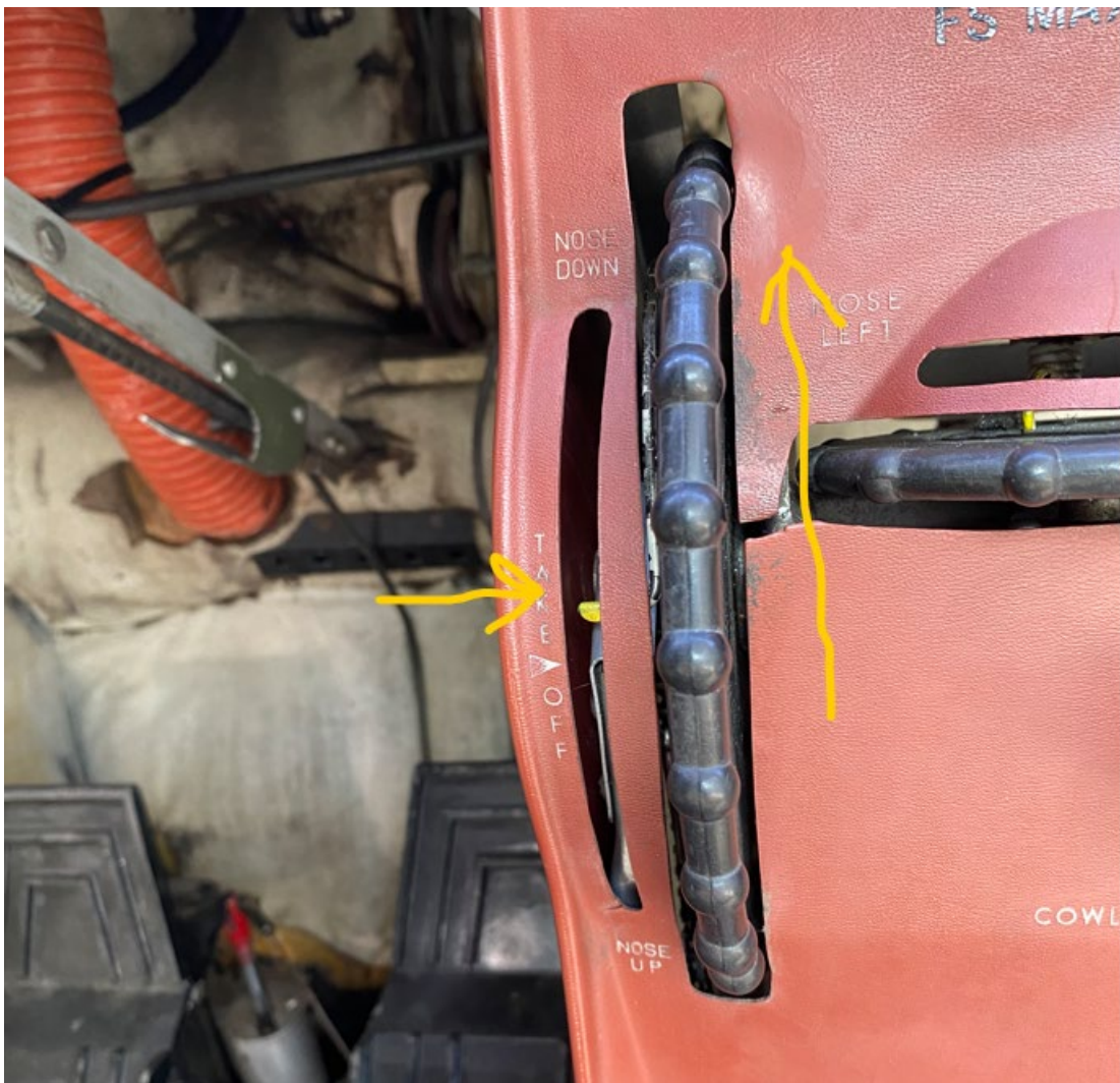
Trim tab with control wheel in the nose up position.
