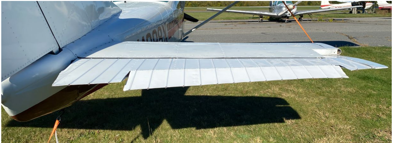
Trim tab with the control wheel in the nose down position.
