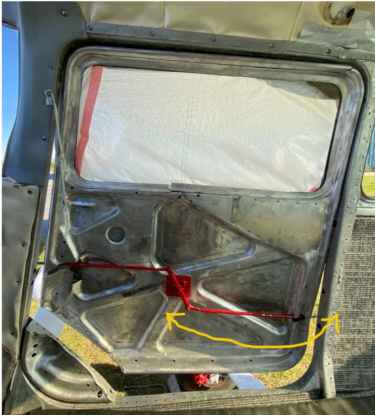
The locking rod is bowed as noted in these photographs.
