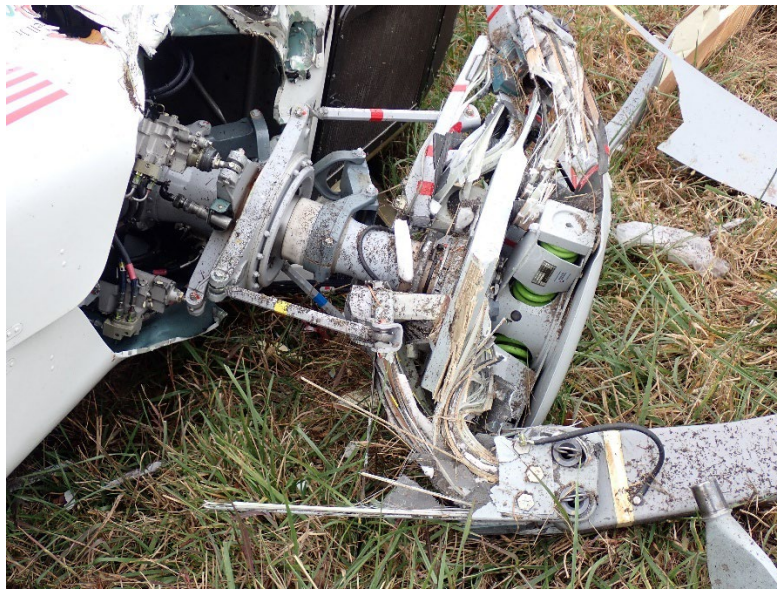
Figure 12. Main rotor Damage (Source: NTSB)
