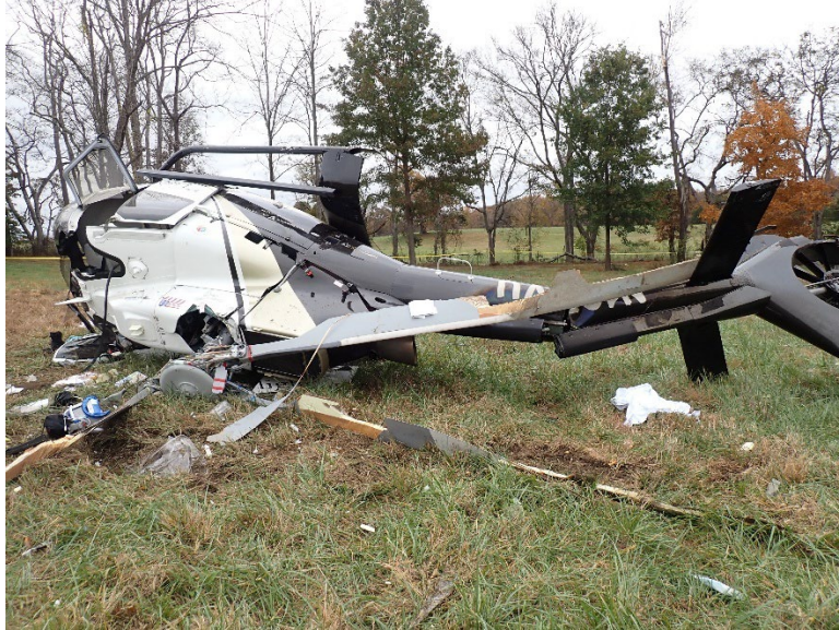
Figure 11. Main rotor Damage (Source: NTSB)
