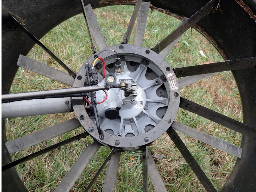
Figure 6. Gear Box (Source: NTSB)
