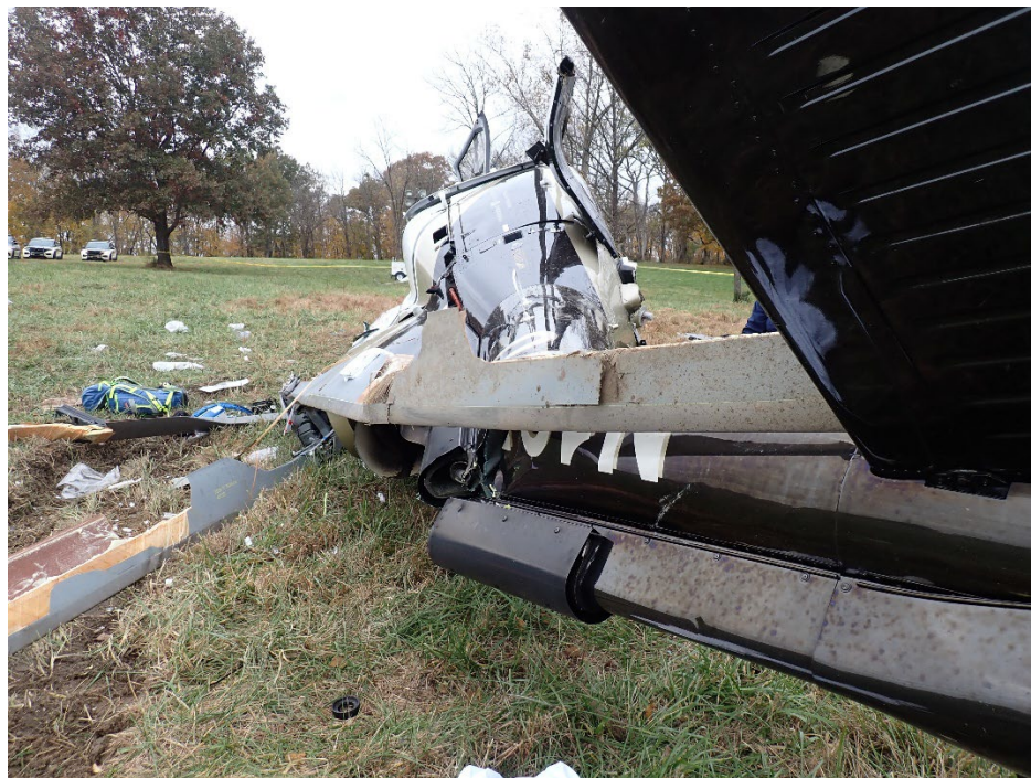
Figure 7. Empennage Damage (Source: NTSB)
