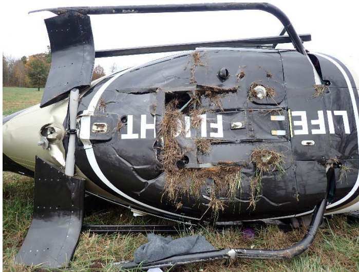
Figure 9. Damage to Skids and Underside (Source: NTSB)
