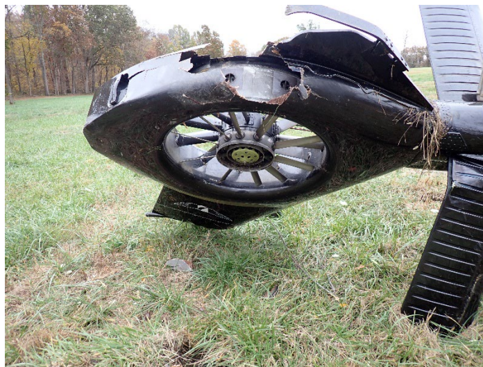
Figure 4. Fenestron Damage (Source: NTSB)
