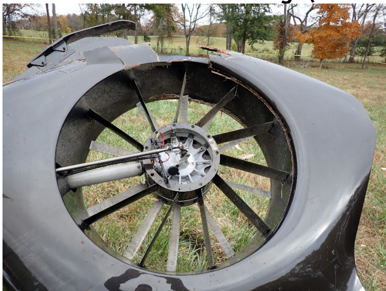
Figure 5. Fenestron Damage (Source: NTSB)
