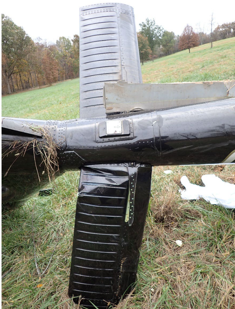
Figure 4. Horizontal Stabilizer Damage (Source: NTSB)
