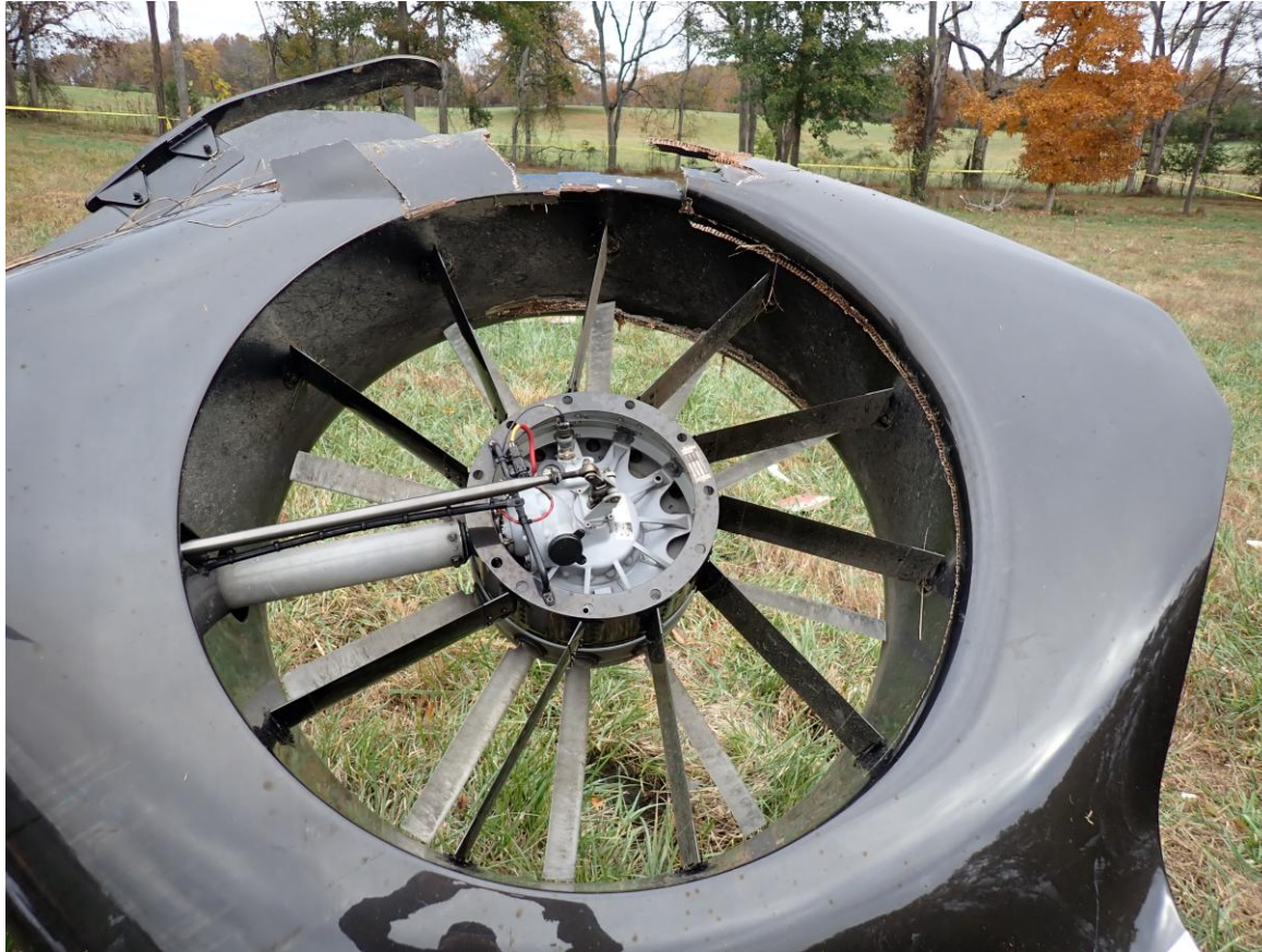
Photograph 3 - Fenestron Damage (Source: NTSB)
