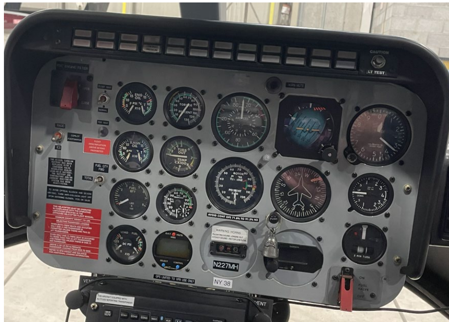
Figure 10. Exemplar (N227MH) instrument panel with caution and warning panel.
