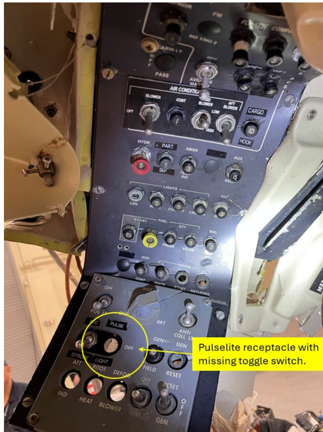
Figure 11. The accident helicopter overhead panel containing the circuit breakers and light switches, including the missing Pulselite switch on the lower left.
