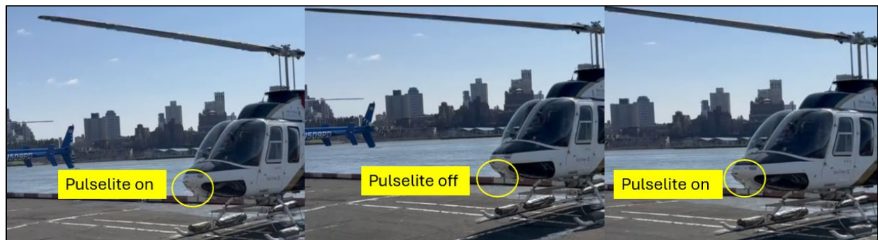
Figure 12. Sequential screen captures of video showing the Pulselite flashing. Full video in the docket shows the helicopter tail wag as reported by witnesses and pilots is listed as Attachment 10. 10
