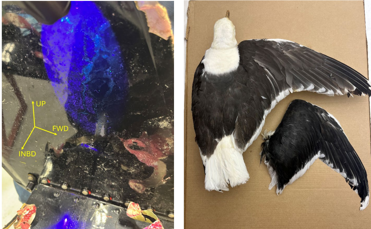
Figure 3. Snare observed on the left horizontal stabilizer and left finlet (left), recovered wing next to Smithsonian Institution's Feather Identification Lab's specimen of Great Black-backed Gull (right)
