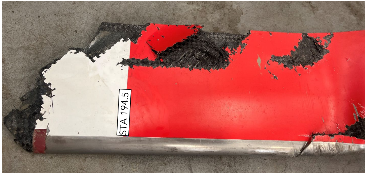
Figure 5. Red blade STA 202 damage
