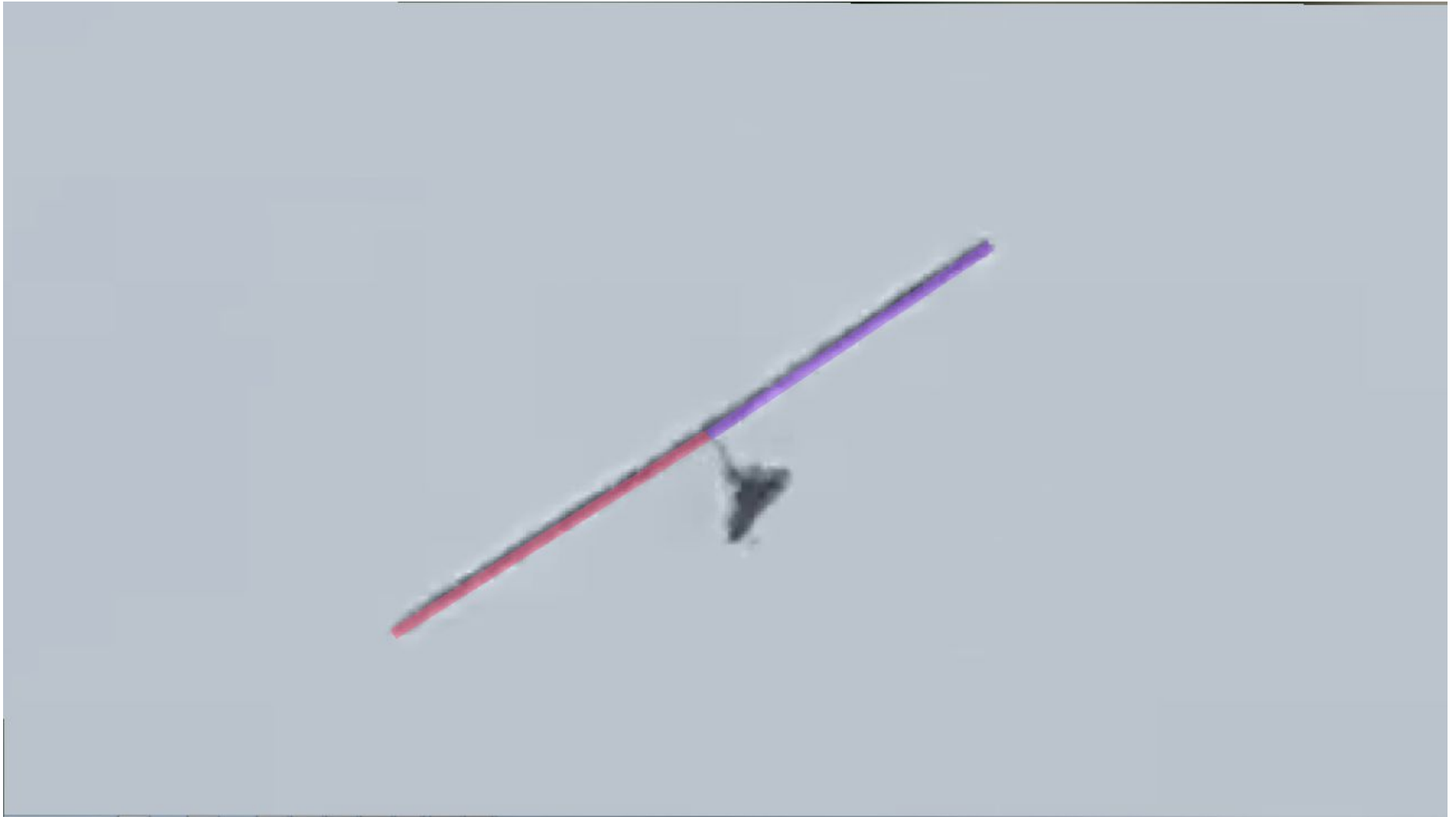
Figure 7: Exemplar frame 33 image subset showing N216MH main rotor blade (zoomed in and cropped from original 2160x3840 pixel image source) annotated with red and purple lines to estimate respective blade lengths.
