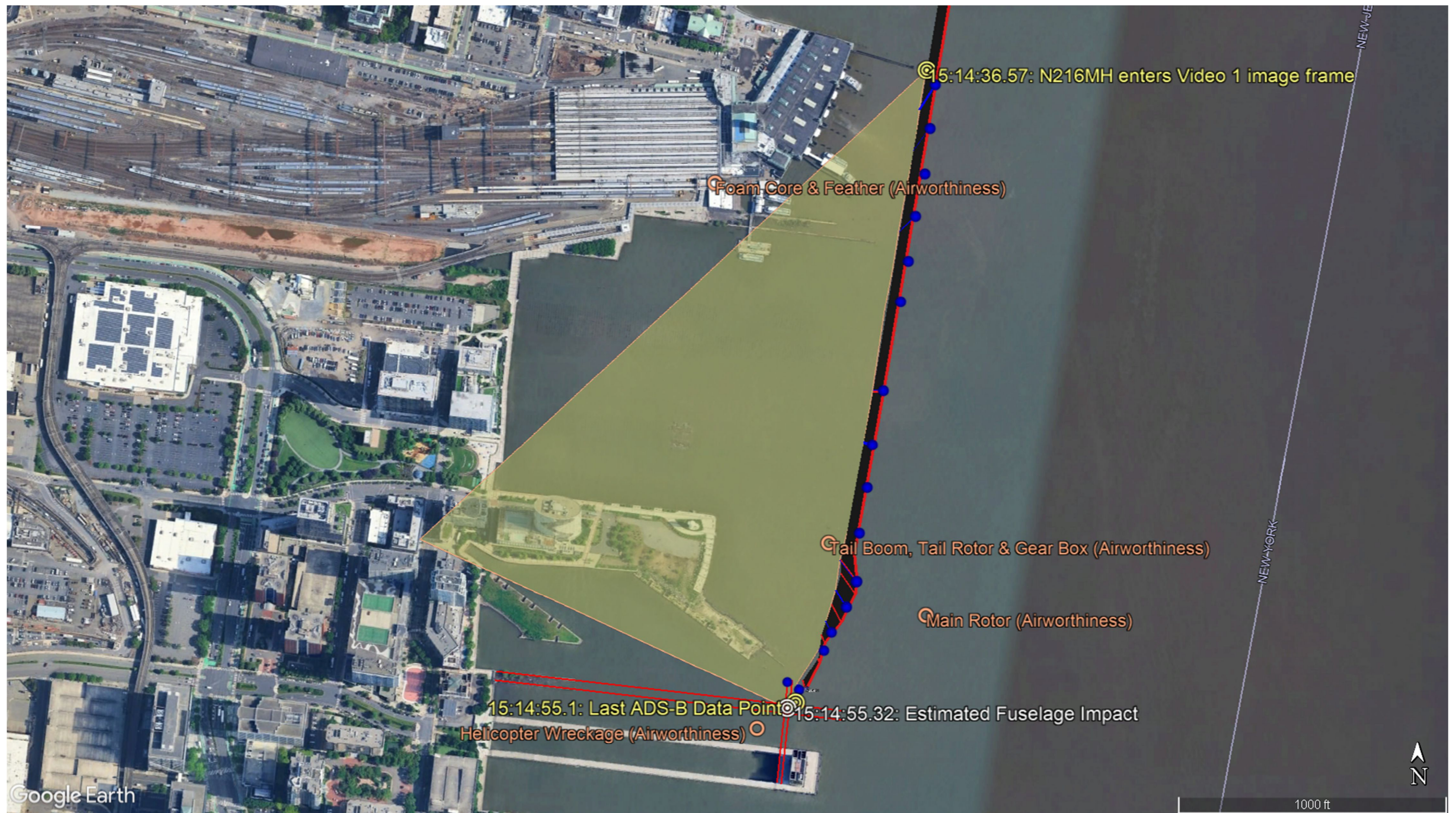
Figure 12: Planform view showing N216MH flight path, ground track, time alignment (with Video 1, Figure1, and Attachment 1-3 content), and helicopter fuselage, main rotor, and tail boom component recovery locations. The helicopter direction of travel was North (top of page) to South. The length of the yellow shaded region adjacent to the ground track corresponds to 18.75 seconds of flight time prior to fuselage water impact.
