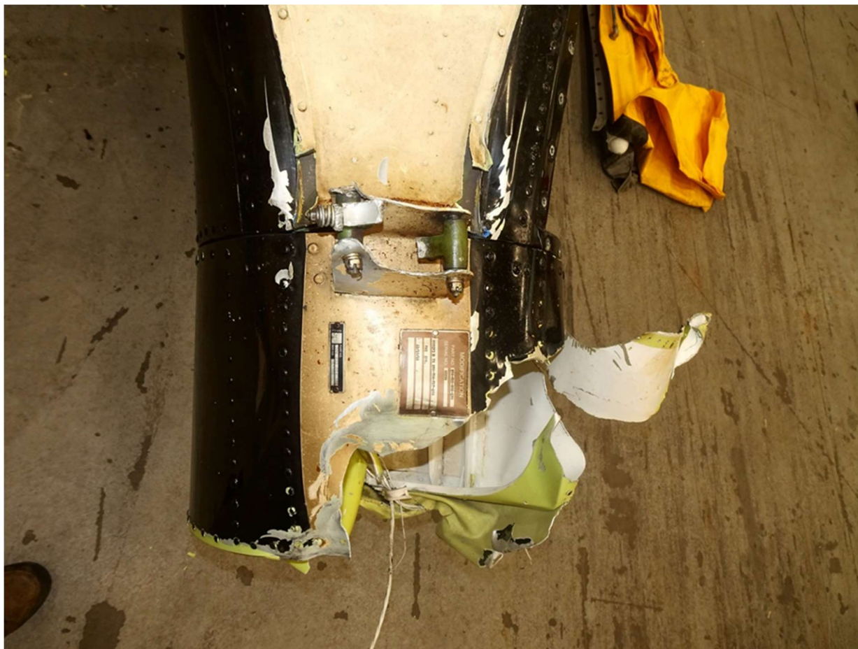
Figure 7. The fractured forward portion of the tail boom at its attachment point.
