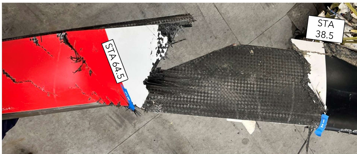
Figure 19. The separation of the red main rotor blade between STA 38.5 and STA 64.5.
