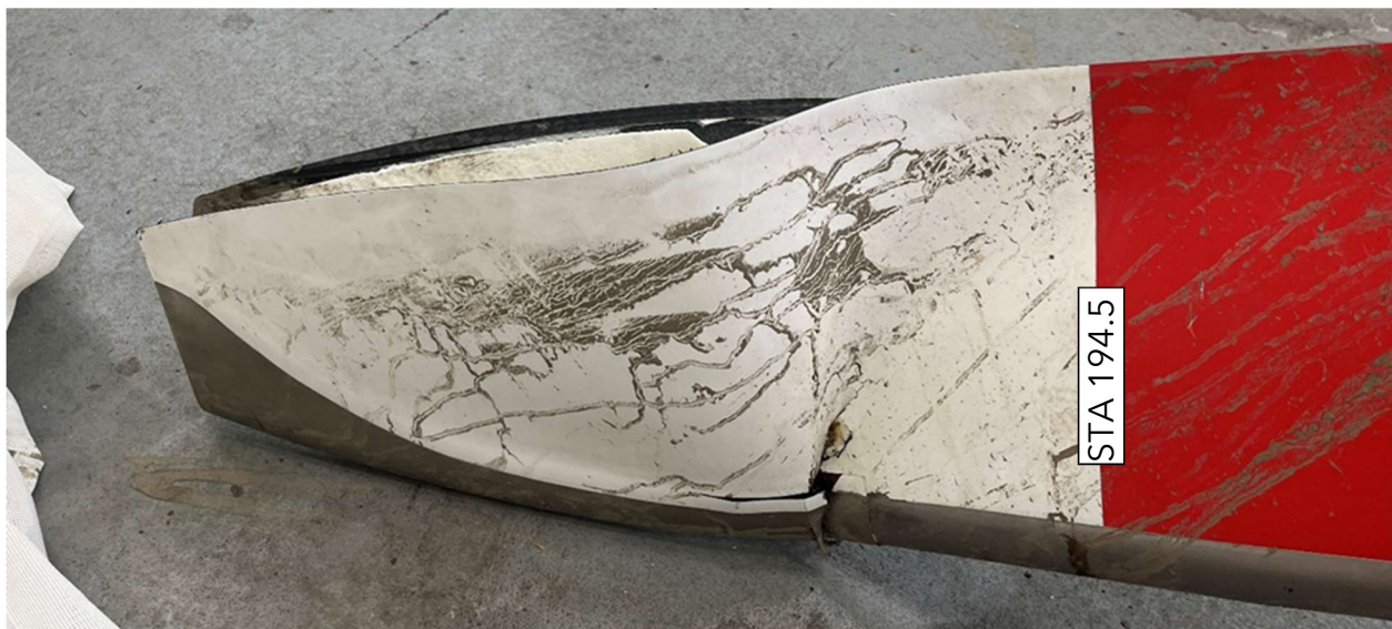
Figure 28. Damage at STA 202.5 on the blue main rotor blade.
