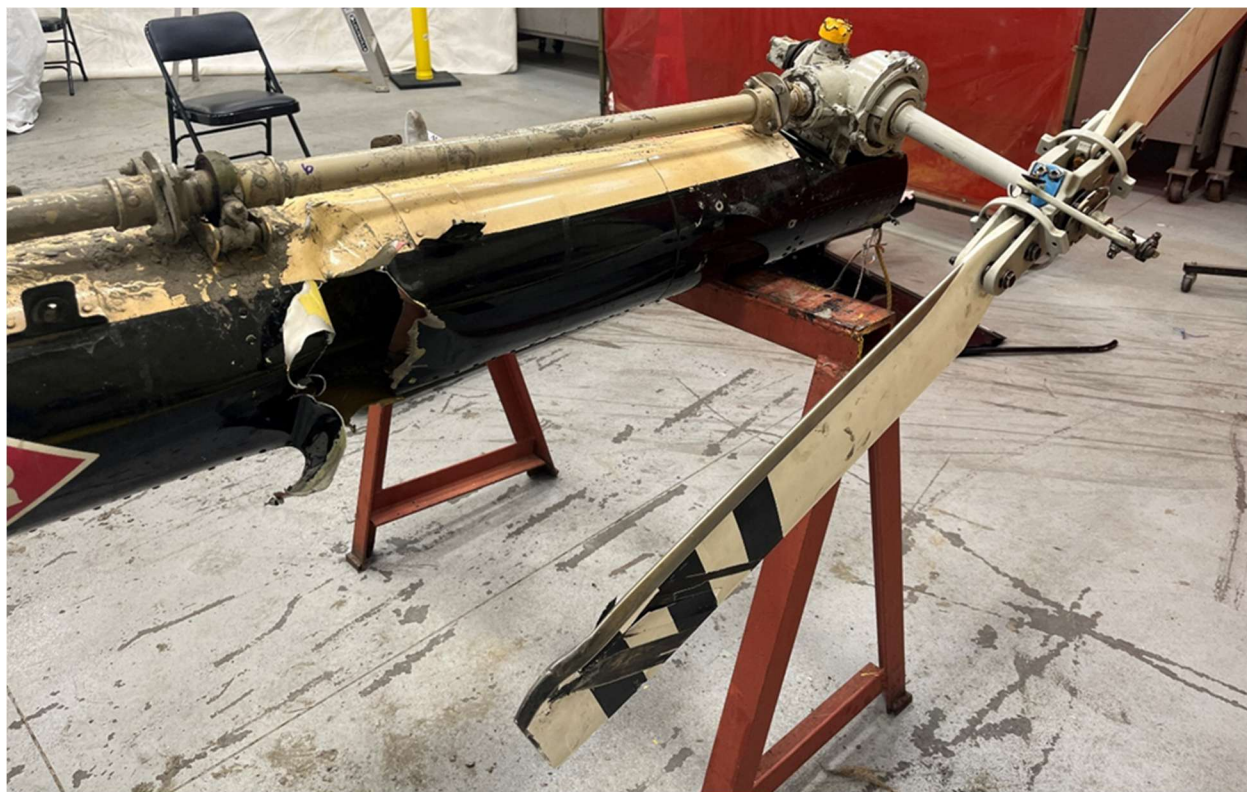
Figure 11. The opening observed at BS 146.088 consistent with tail rotor blade contact.
