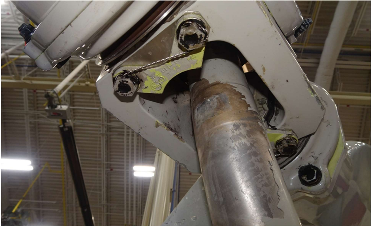
Figure 16. The main rotor mast showing contact with the bump stop adjacent to the red main rotor blade.
