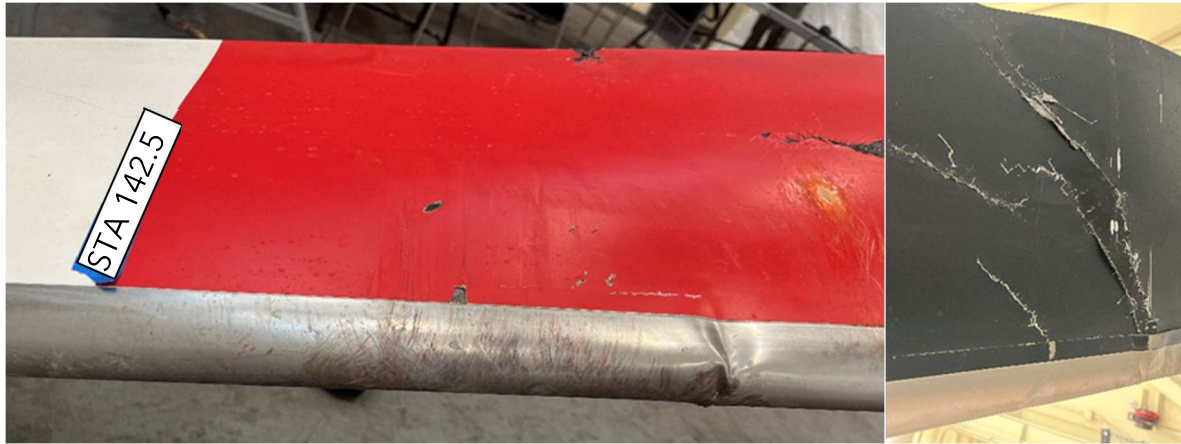
Figure 21. Damage at STA 128.5 on the red main rotor blade.
