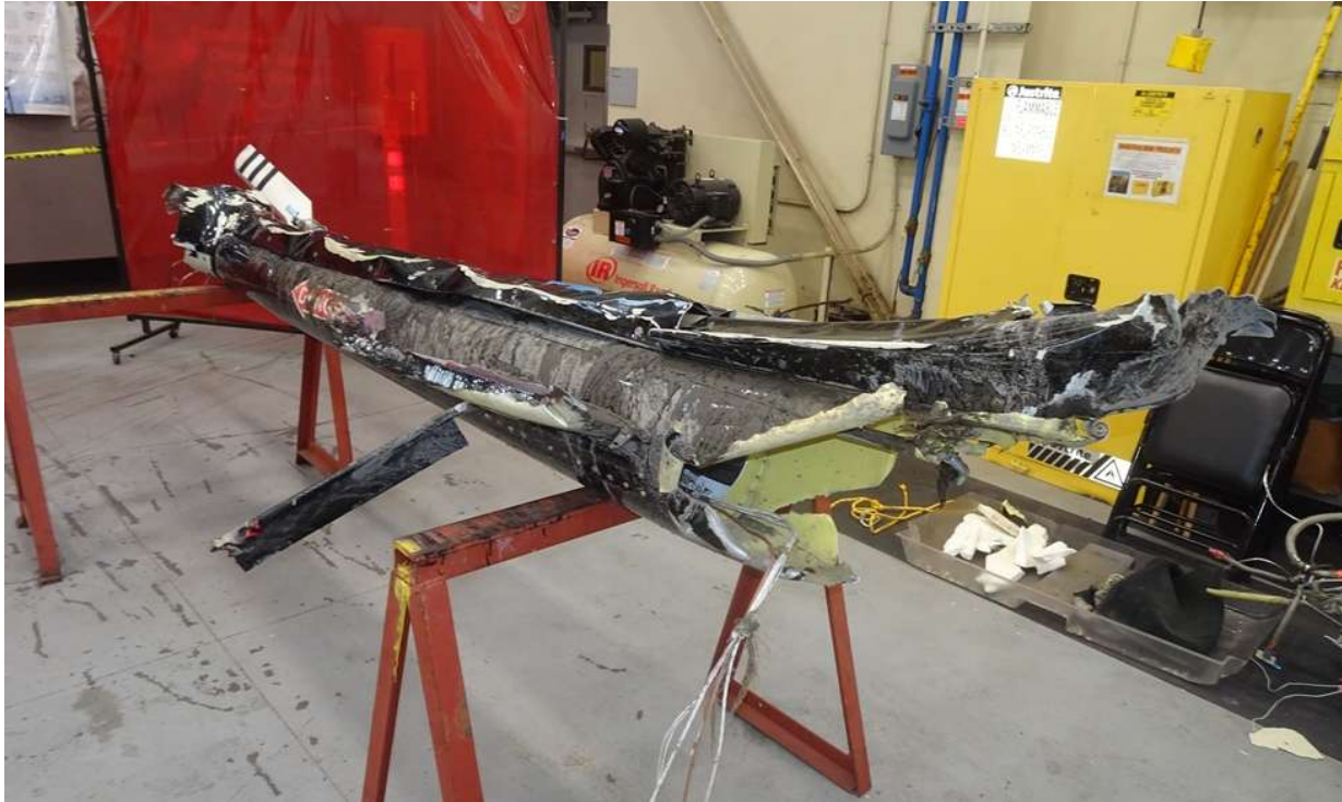
Figure 8. The recovered tail boom.
