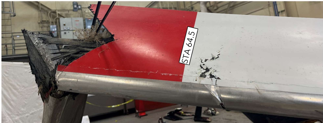
Figure 25. Damage on the blue main rotor blade at STA 61.5.
