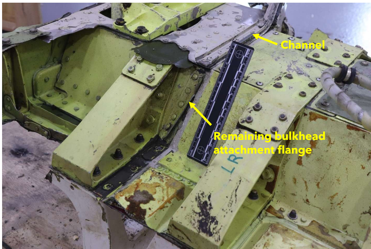
Figure 34. Roof beam structure left rear side.
