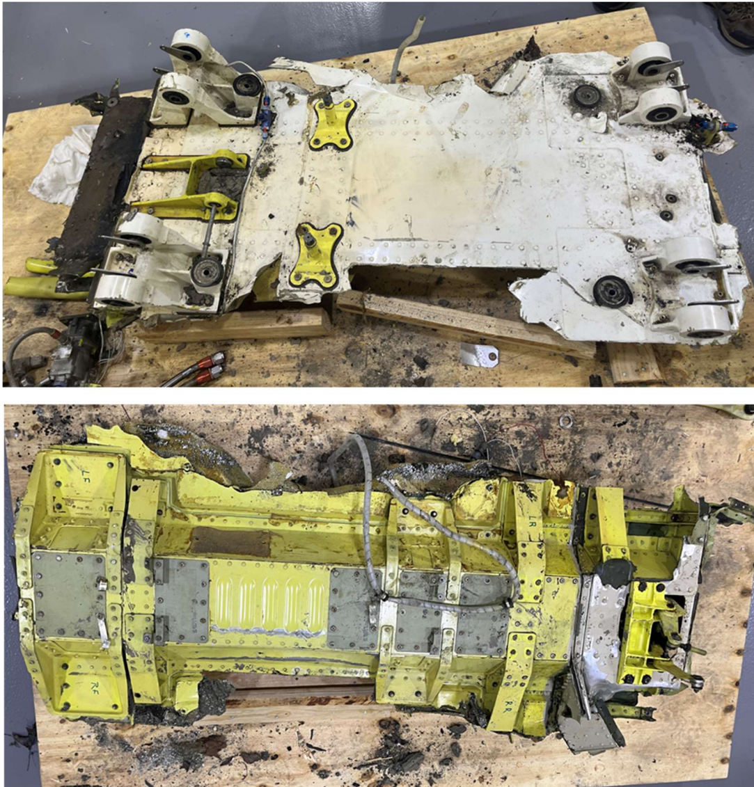
Figure 32. The upper and lower surfaces of the roof structure.
