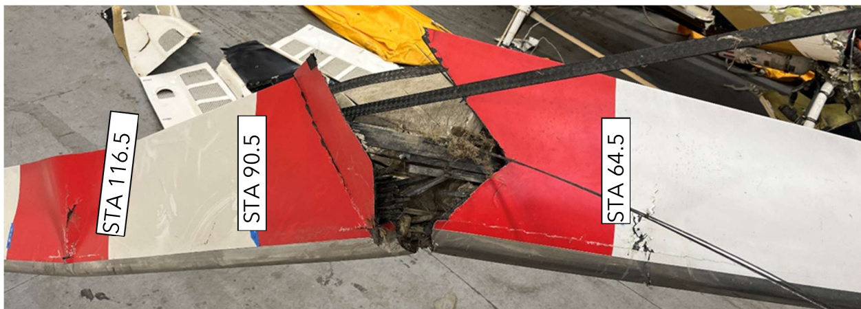
Figure 26. Damage at STA 76 on the blue main rotor blade.
