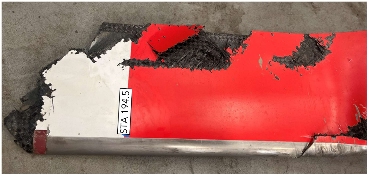
Figure 23. Damage at STA 194.5 on the red main rotor blade.
