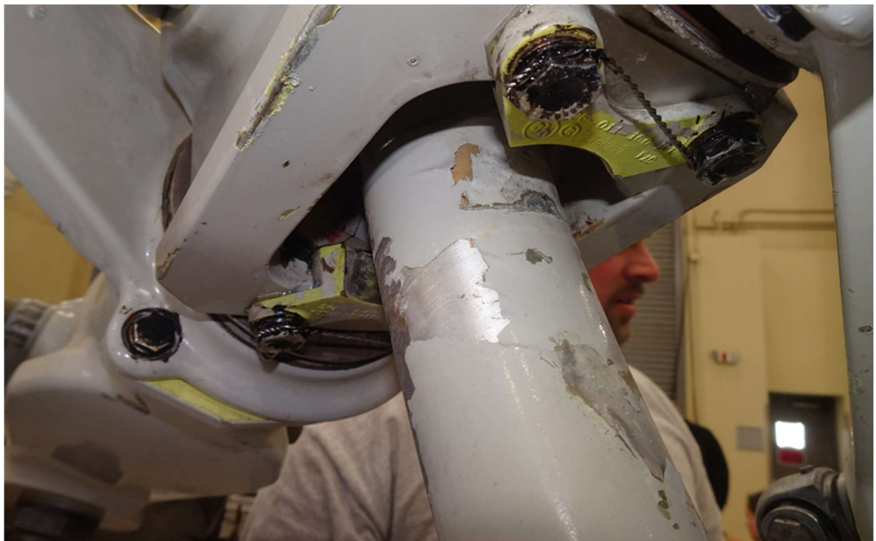
Figure 17. The main rotor mast showing contact with the bump stop adjacent to the blue main rotor blade.
