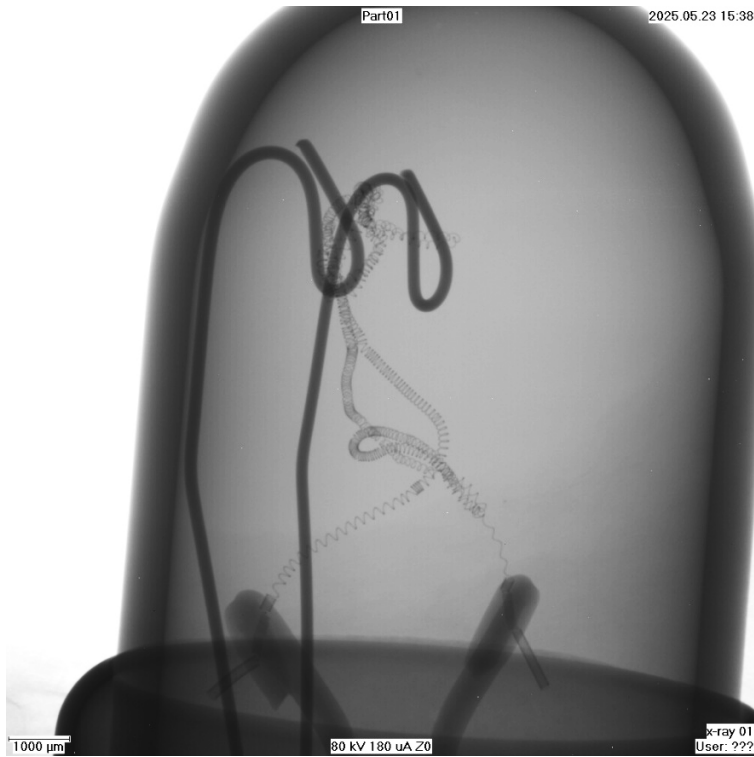
Figure 9. Radiograph of LF FUEL PUMP Bulb 2.
