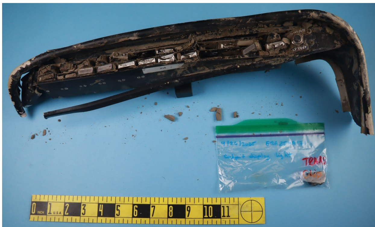
Figure 2. Photograph of as-received annunciator panel. The TRANS CHIP annunciator (in the plastic bag) was found separated from the panel.
