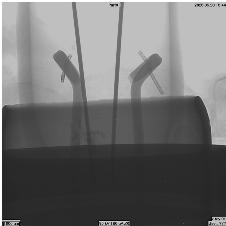
Figure 10. Radiograph of ROTOR LOW RPM Bulb 1.
