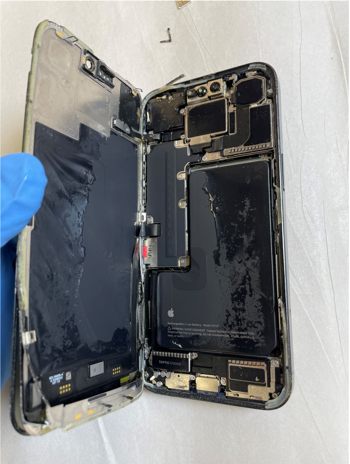
Figure 2. The interior of the Apple iPhone 15 Pro Max after being opened.
