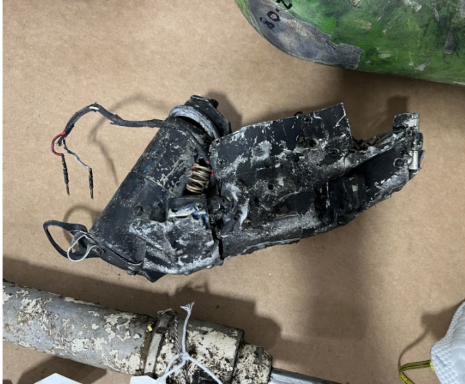
Figure 36: Secondary Pitch Trim Motor Found within the Debris
