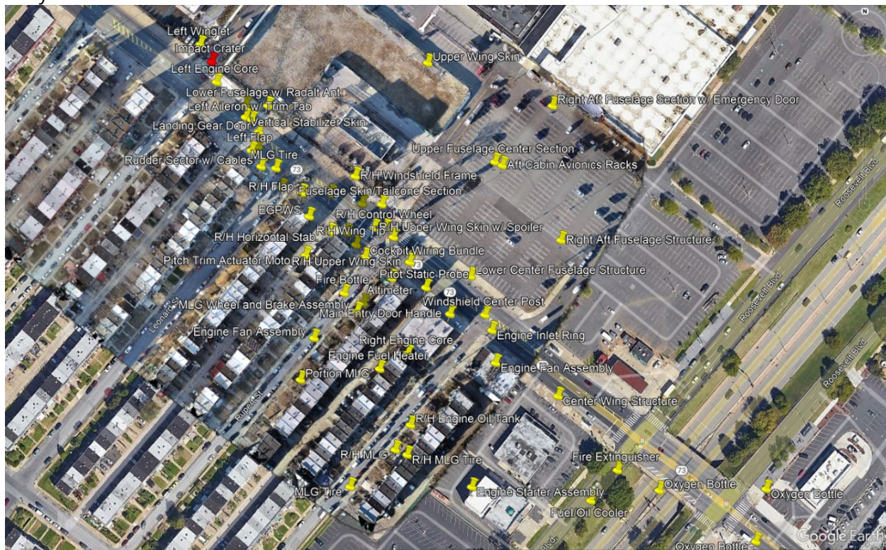
Figure 6: Impact Point and Debris Location with Aerial Photography Overlay. The Debris Path was 1410 ft in Length and 840 ft in Width
