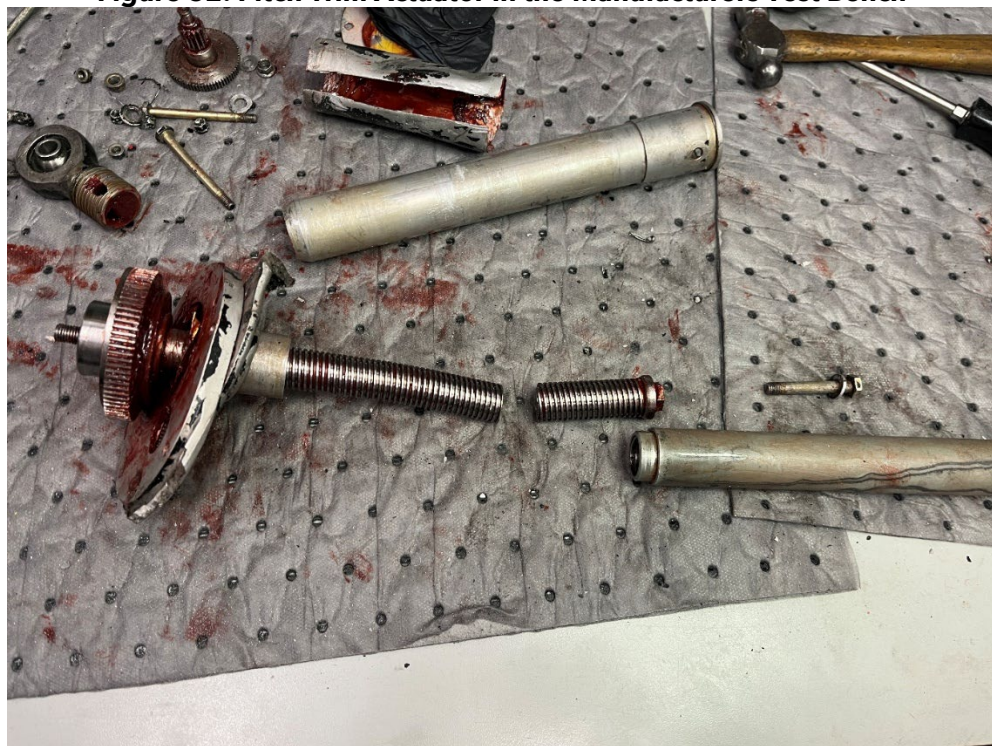
Figure 33: Pitch Trim Actuator Displaying Bending and Fracture to the Screw Assembly
