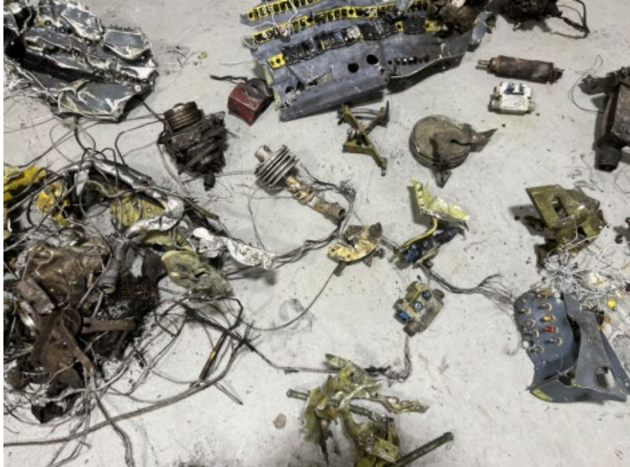
Figure 16: Cockpit Instrumentation, Circuit Breakers, and Controls
