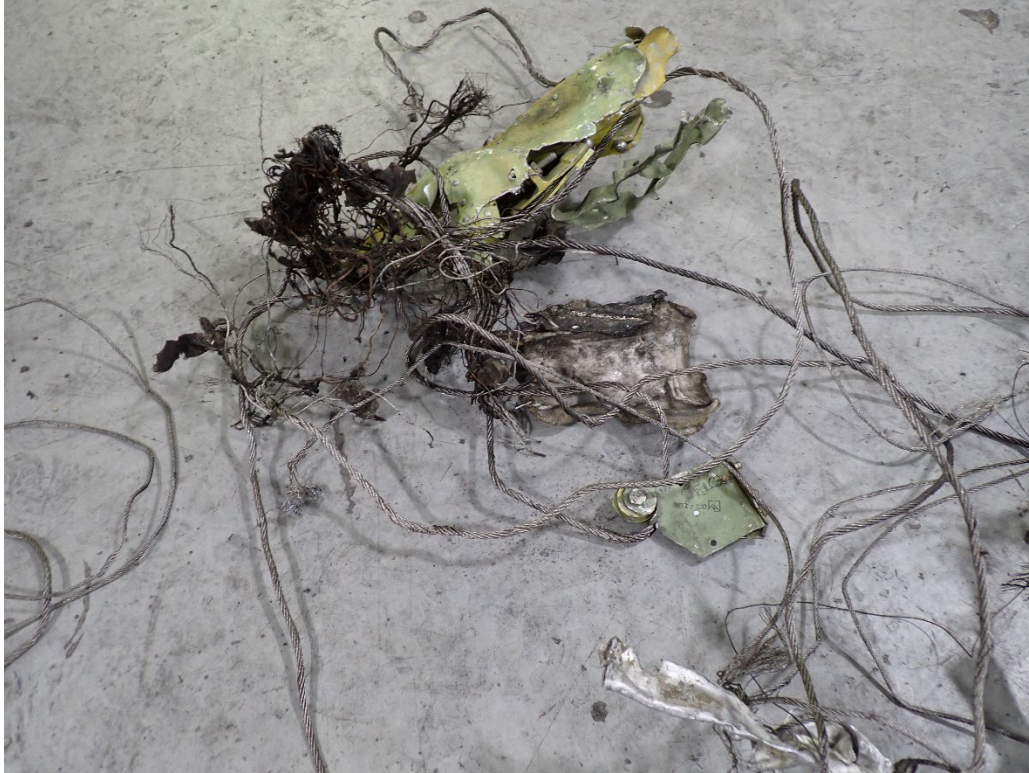
Figure 10: Control Cables Extending From the Cockpit Debris
