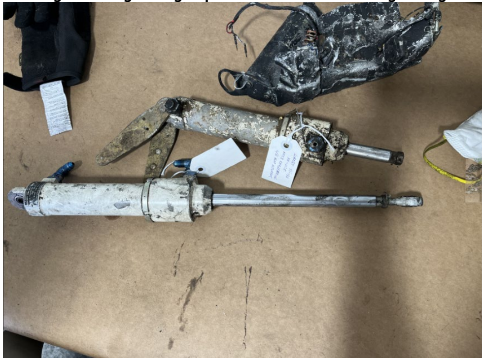
Figure 35: Left and Right Flap Actuators
