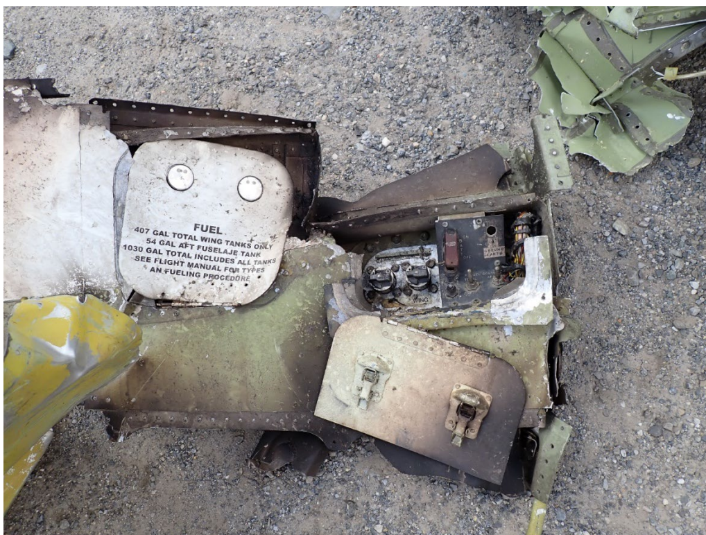
Figure 30: Exterior Fueling Control Panel
