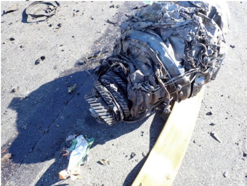
Figure 41: Left Engine Core as Found Adjacent to the Impact Crater
