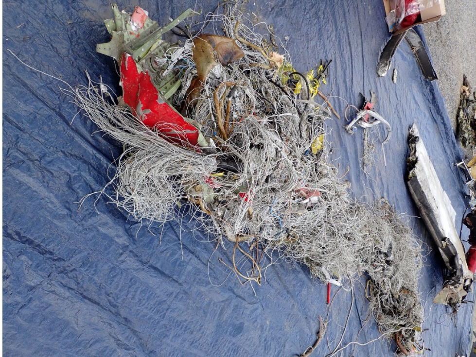
Figure 22: Large Wiring Harness and Bundles as Recovered
