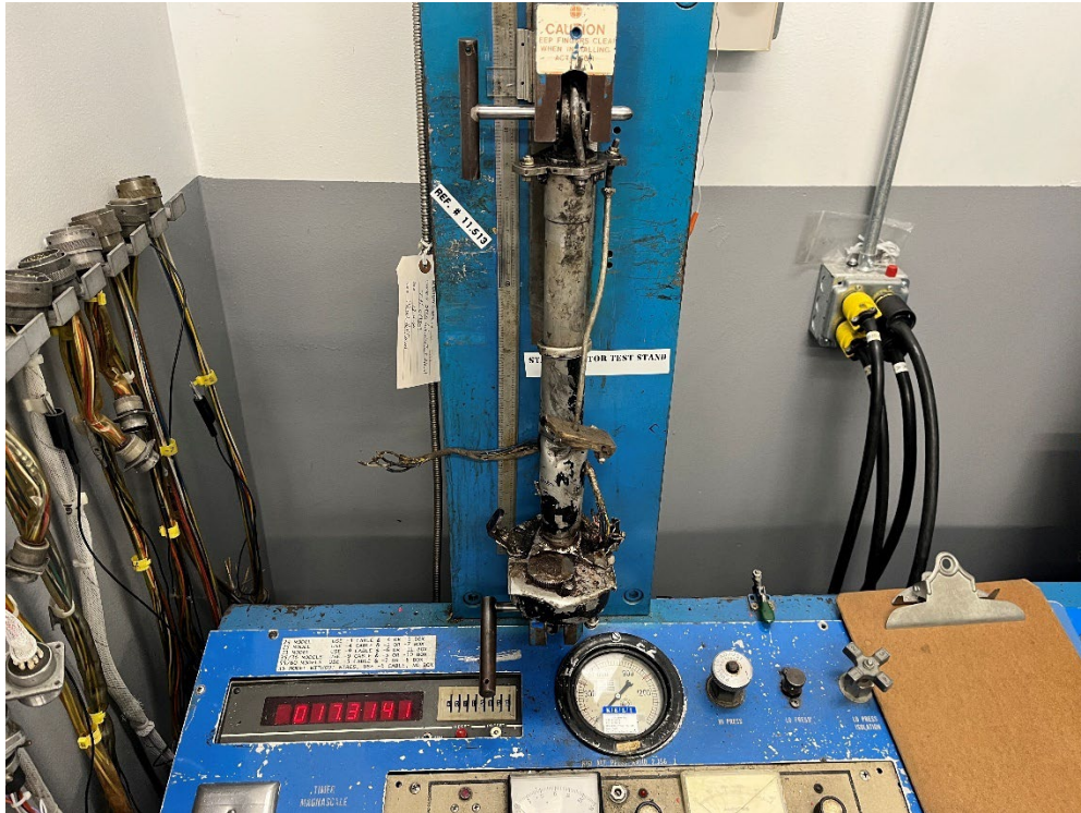
Figure 32: Pitch Trim Actuator in the Manufacturer's Test Bench
