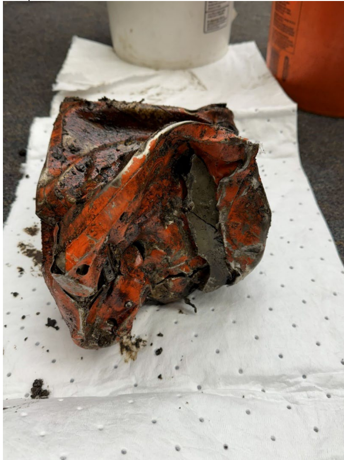
Figure 31: CVR Post Removal from the Impact Crater with Exterior Damage
