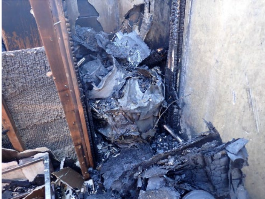
Figure 40: Right Engine Core as Found on the Second Floor of a Residential Structure
