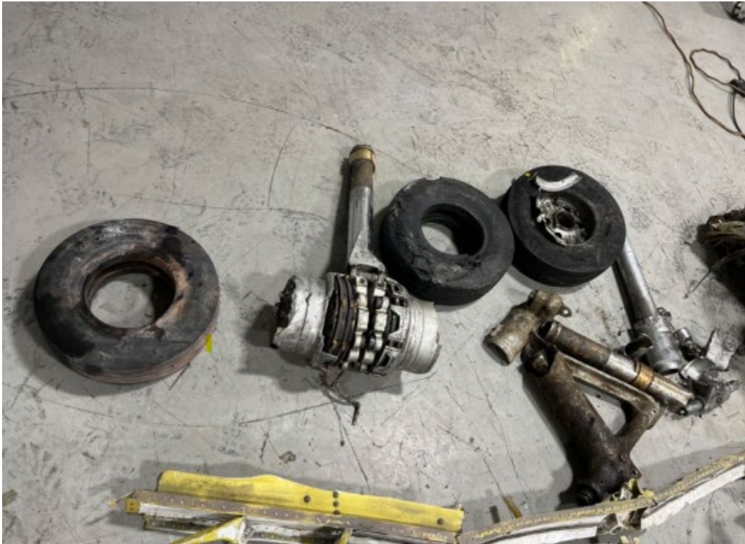
Figure 29: Pieces of the Landing Gear
