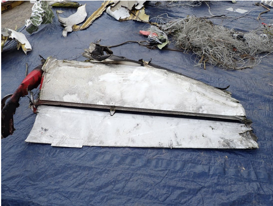
Figure 24: Portion of the Left Horizontal Stabilizer and Elevator
