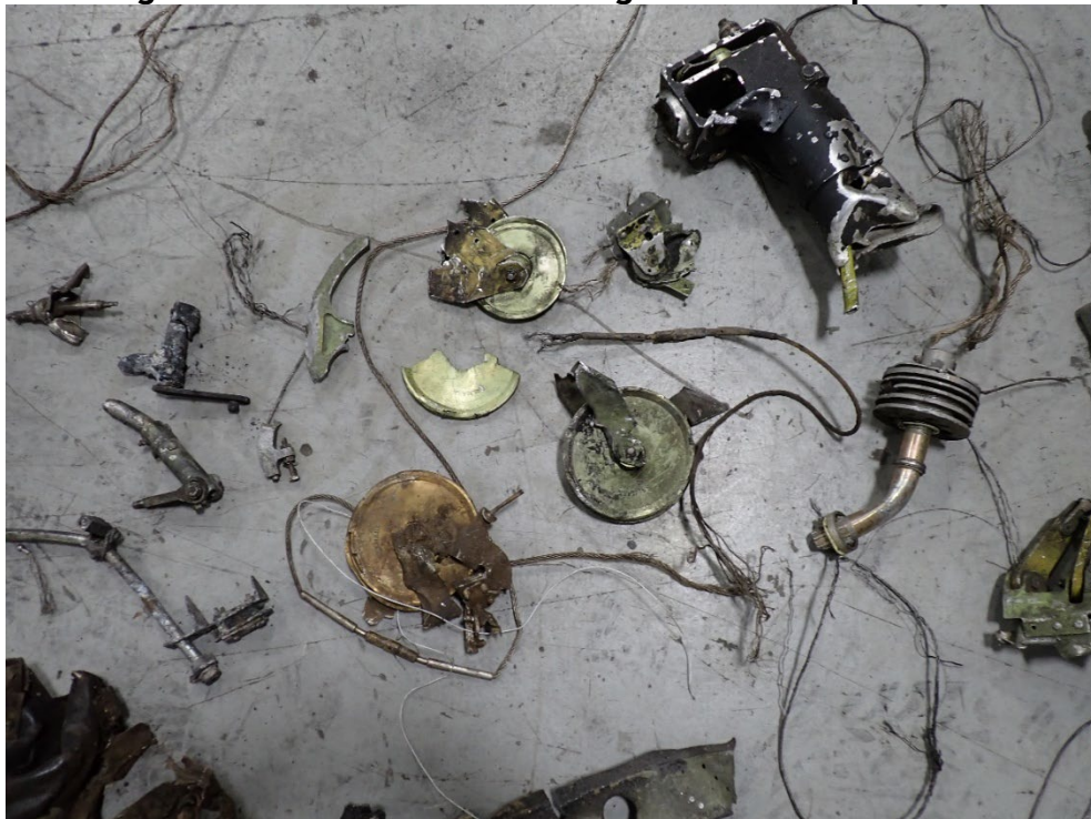
Figure 11: Miscellaneous Control Cables and Pulleys
