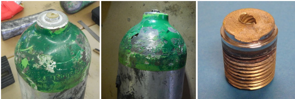
Figure 10: Photos of Cylinder #6 showing fractured valve stem remaining in cylinder neck (left), gouge observed in crown (center), and fractured valve stem removed from cylinder (right).
