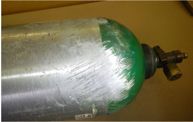
Figure 1: Cylinder #1, crown, scrape, and intact bent valve stem (March 26, 2025).
