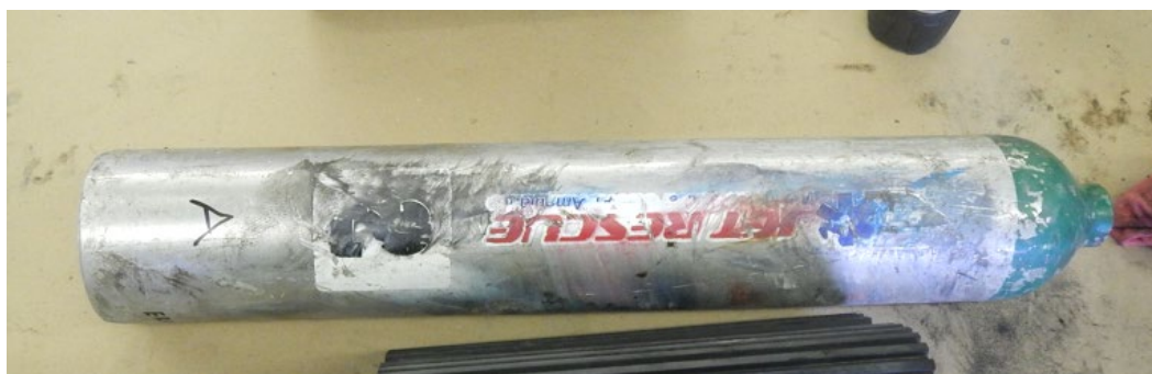
Figure 8: Photo of Cylinder #4 showing black, blue, and red impressions on cylinder wall (March 26, 2025).
