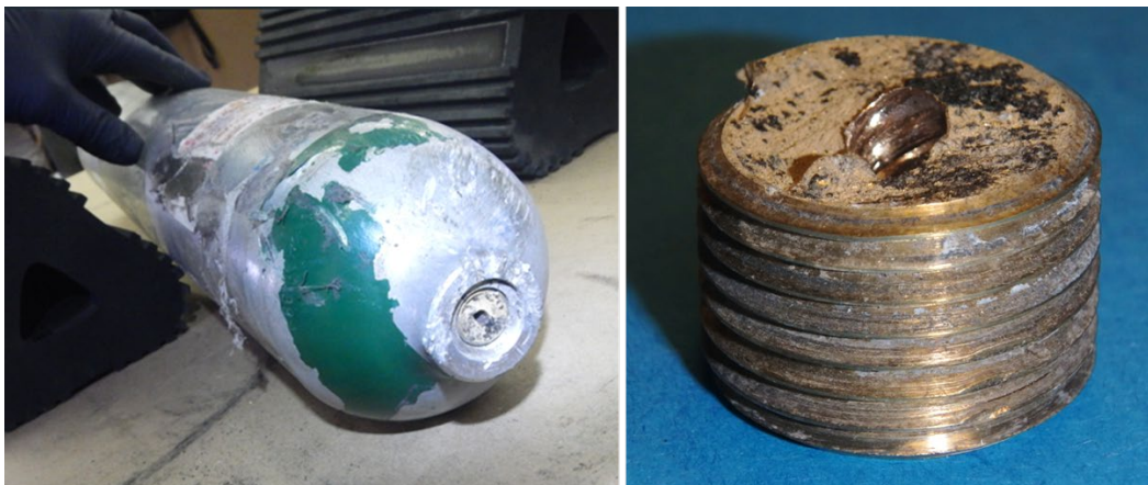
Figure 9: Photos of Cylinder #5 showing fractured valve stem and collar witness mark (left), and fractured valve stem removed (right).
