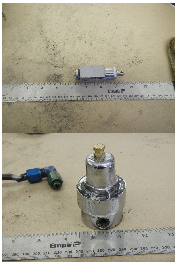
Figure 26: Photos of oxygen valve body stamped CGA870 (top) and an oxygen pressure regulator (bottom) (March 26, 2025).
