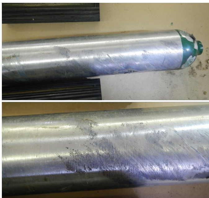
Figure 6: Photos of Cylinder #3 showing notable fabric impression on cylinder wall (March 26, 2025).
