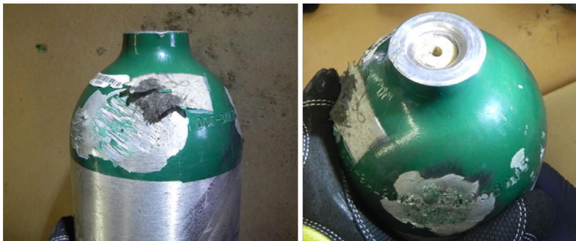
Figure 5: Photos of Cylinder #3 showing observed crown gouge (left) and fractured valve stem (right) (March 26, 2025).
