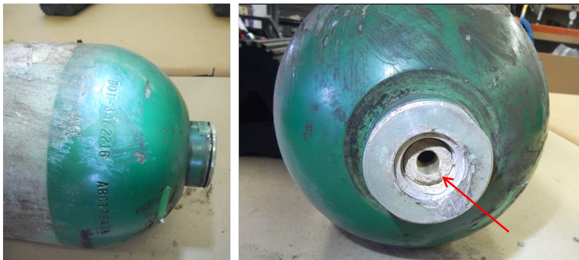
Figure 4: Photos of Cylinder #2 crown and bottom portion of fractured valve stem (red arrow) (March 26, 2025).
