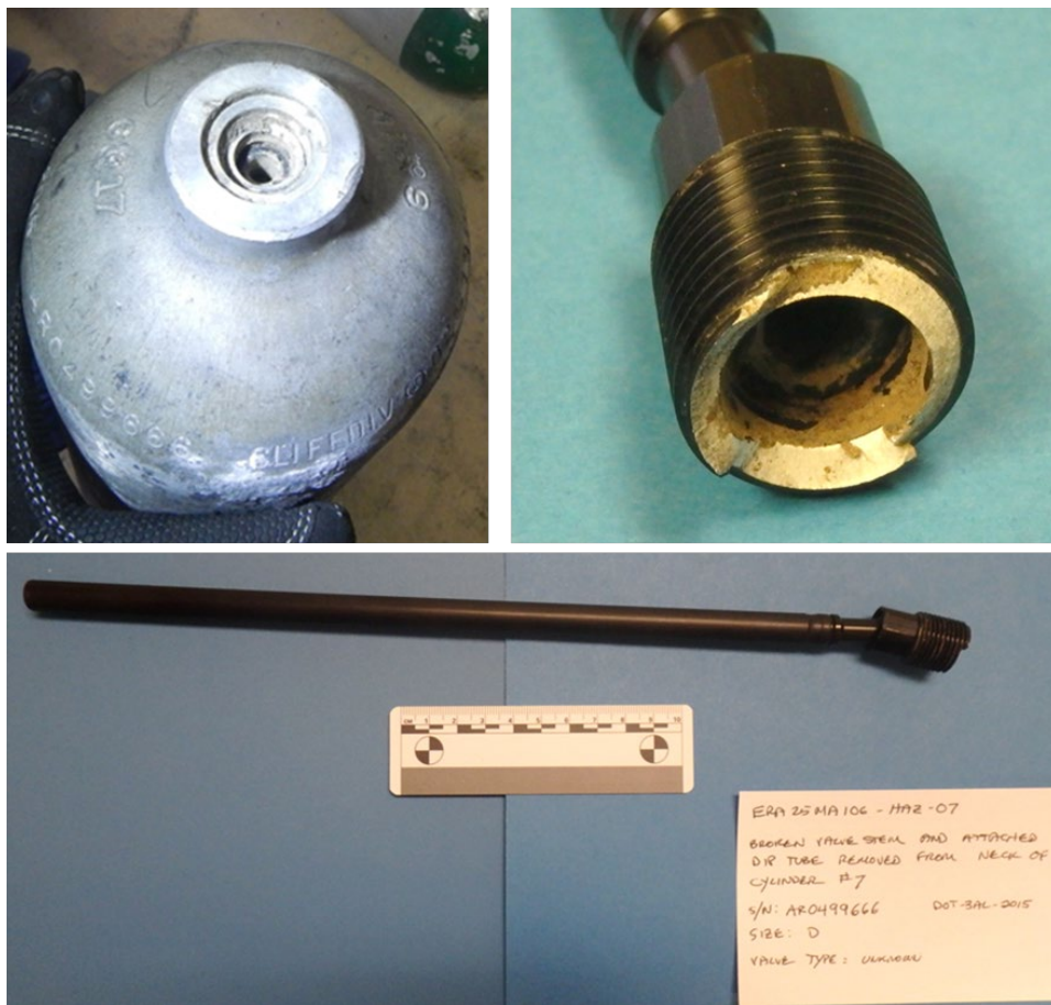
Figure 14: Photos of Cylinder #7 crown and collar (top left), fractured valve stem (top right), and dip tube (bottom) (March 26, 2025).
