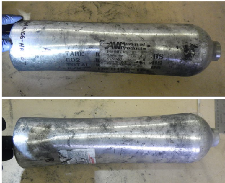
Figure 15: Photos of Cylinder #7 walls dented and bowed out (March 26, 2025).
