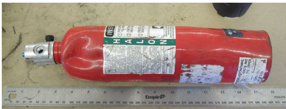
Figure 18: Photo of Halon Cylinder #3 (March 26, 2025).
