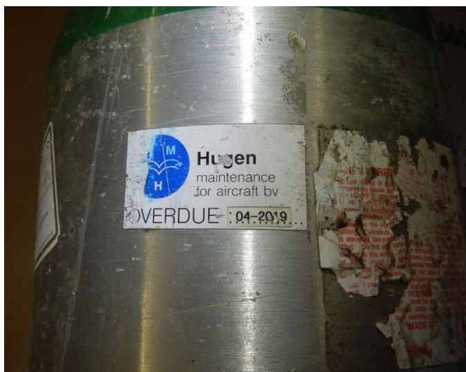
Figure 3: Cylinder #1, maintenance overdue sticker (March 26, 2025).
