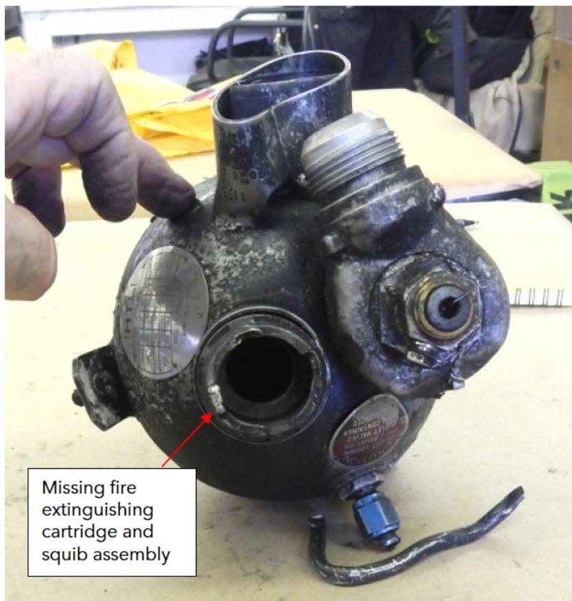
Figure 16: Photo of actuated Halon Cylinder #1 with one of its fire extinguisher cartridge and squib assembly missing (March 26, 2025).
