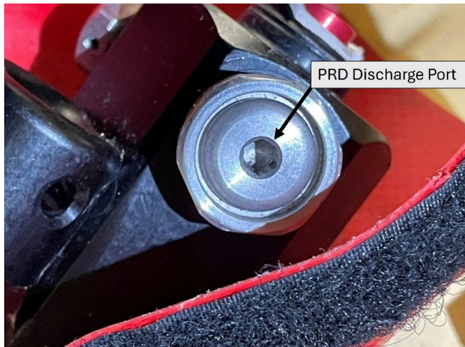
Figure 25: Close-up of pressure relief device discharge port with disc visibly in place (February 2, 2025, annotation by NTSB).
