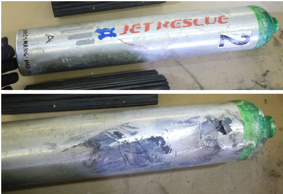
Figure 11: Photo of Cylinder #6 showing dents observed on the wall of the cylinder at the base of the crown and fabric adhered to tank wall.
