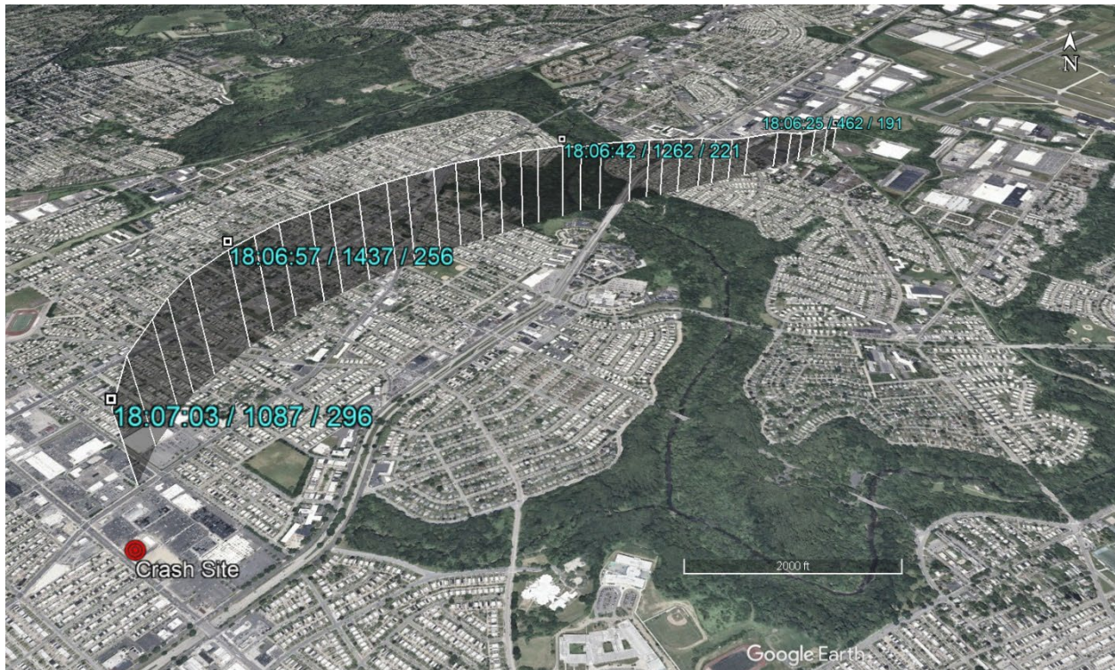
Figure 2. View of the flight path on a Google Earth background, with selected points annotated. Annotations indicate EST time, MSL altitude in ft and calibrated airspeed in kt. The airport is at upper right, and the crash site is marked with a red circle.
