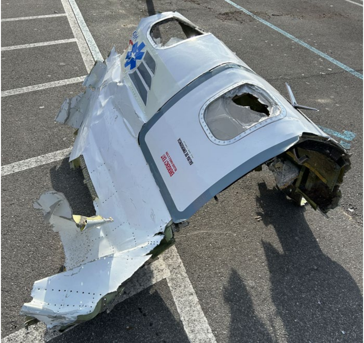
Figure 19: Emergency Egress Door
