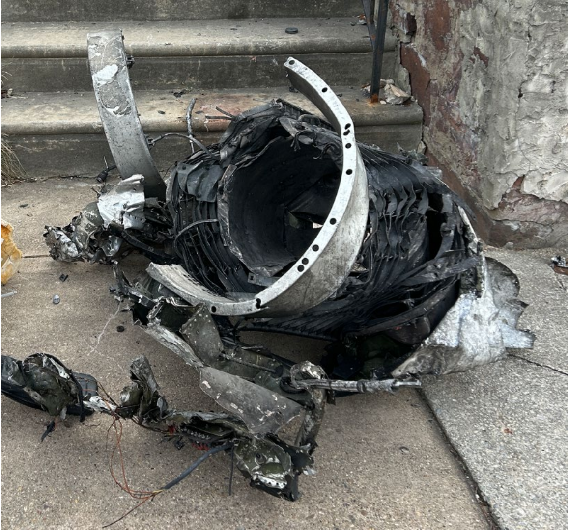
Figure 22: Portion of Right-hand Thrust Reverser
