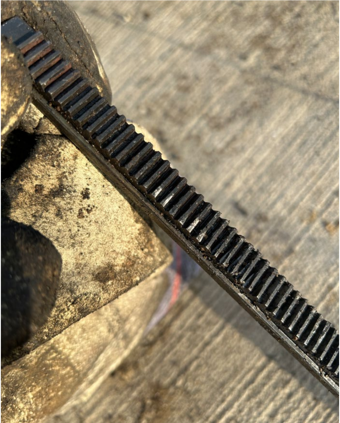
Figure 32: Possible Witness Marks on Thrust Reverser Rack
