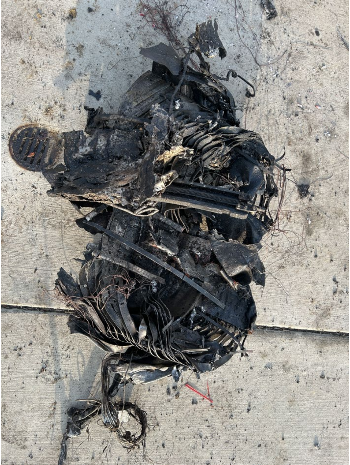
Figure 30: Thrust Reverser Assembly Recovered from Crater
