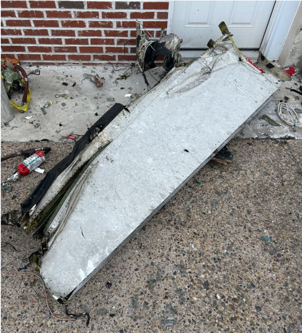
Figure 23: Portion of Right-hand Horizontal Stabilizer
