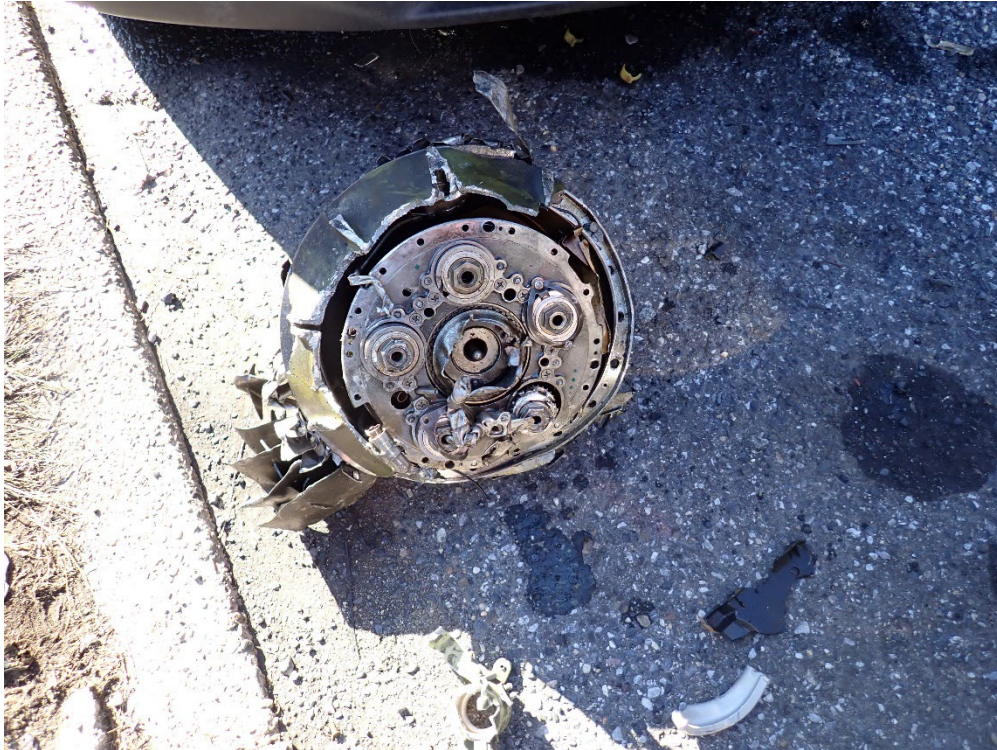
Figure 52: Fan Assembly 1 Located on Rupert St. (Courtesy of Honeywell)
