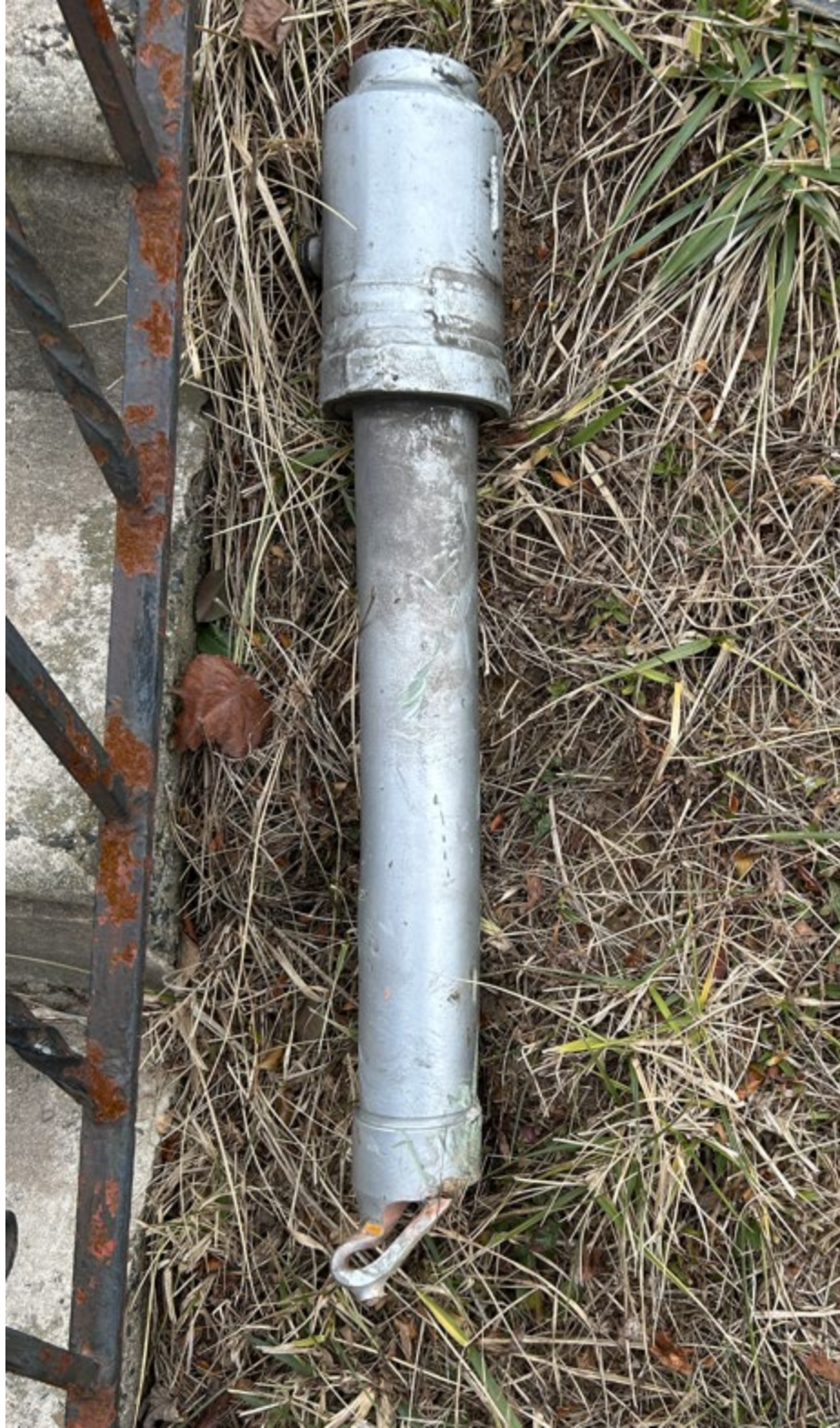
Figure 28: Main Landing Gear Actuator
