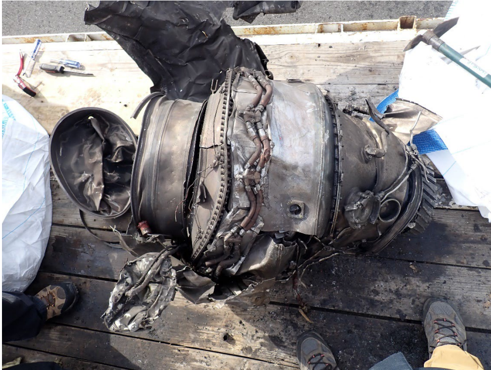
Figure 42: Engine Core 1 Fractured Plenum and T-Duct (Courtesy of Honeywell)
