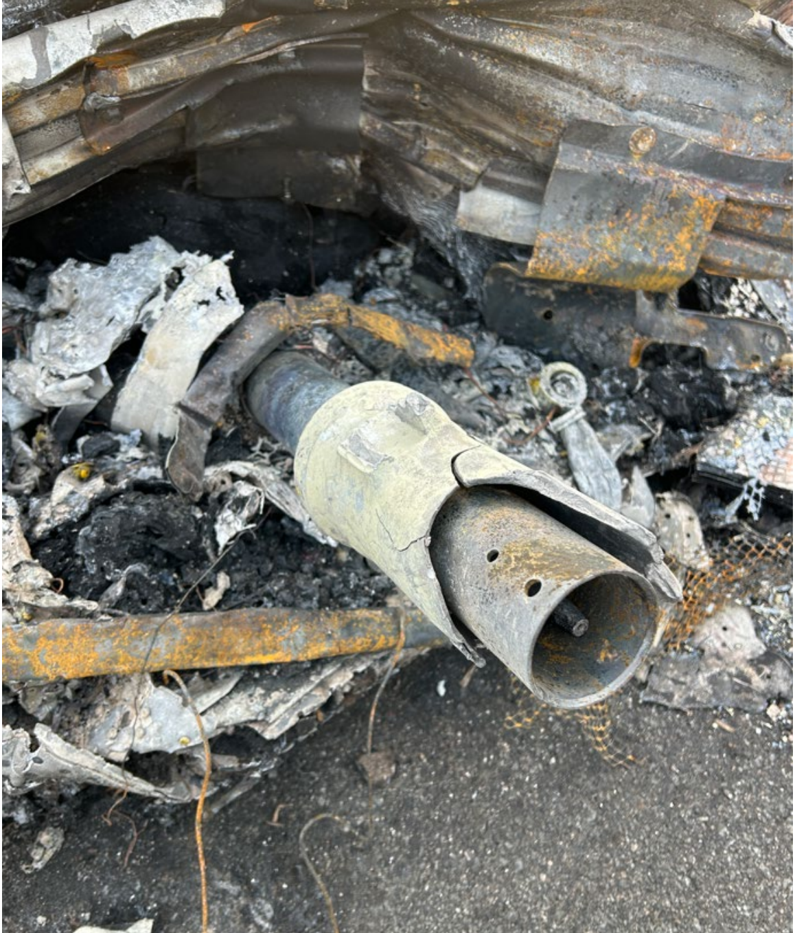
Figure 3: Nose Landing Gear Strut
