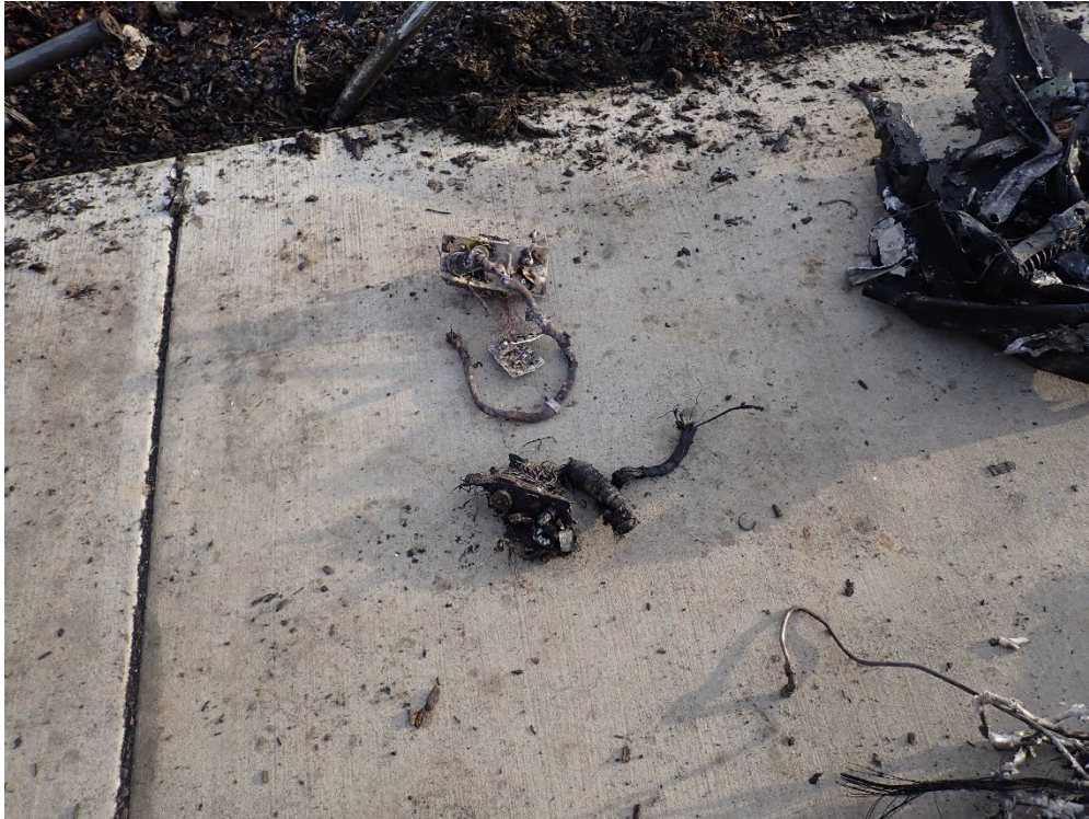
Figure 60: Remains of Engine EEC's (Courtesy of Honeywell)
