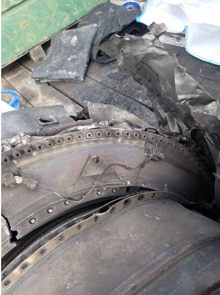
Figure 43: Engine Core 1 3 O'Clock Aft Engine Mount Bolt Hole Torn Outward (Courtesy of Honeywell)
