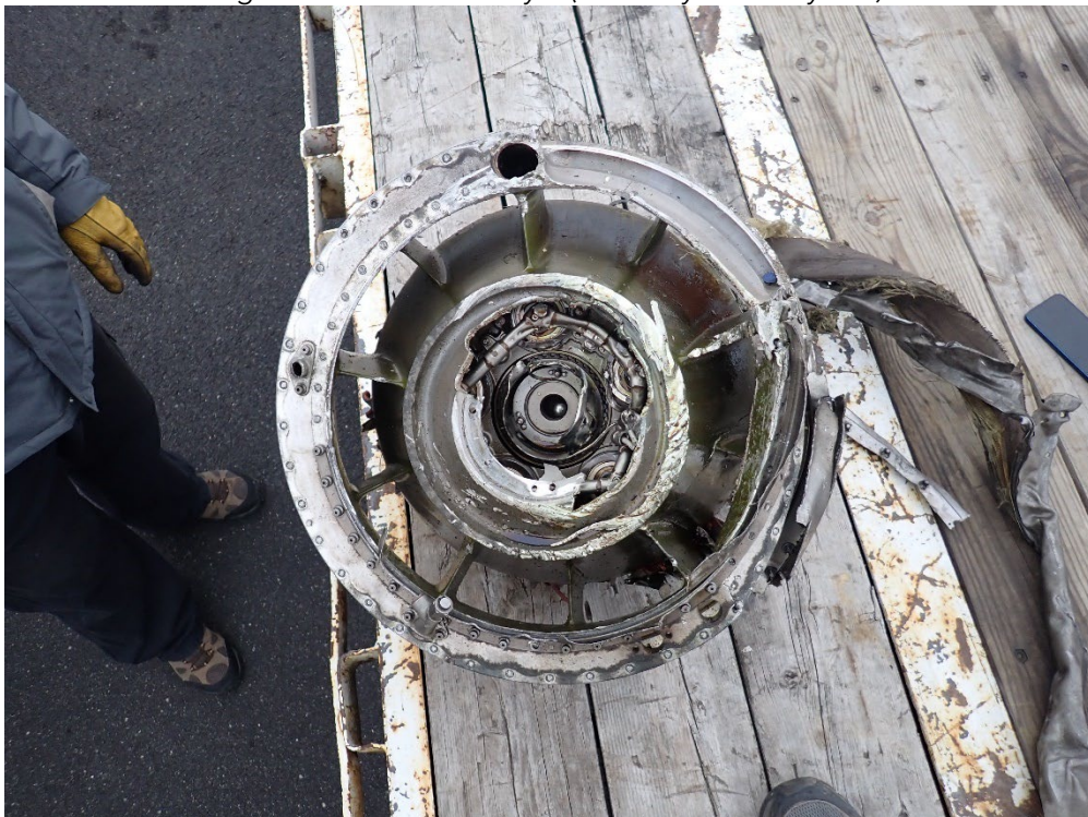
Figure 59: Fan Assembly 2 (Courtesy of Honeywell)
