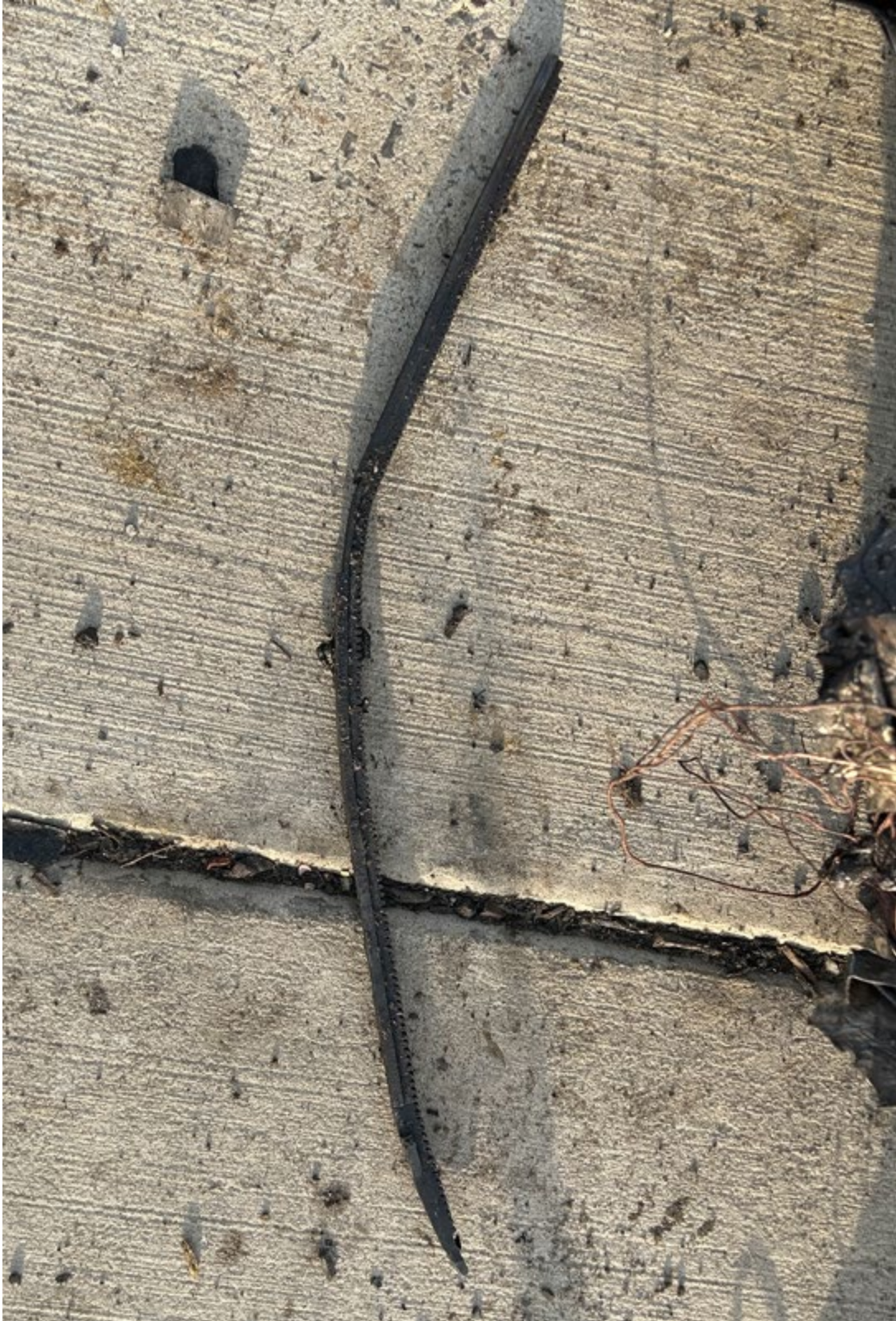
Figure 31: Thrust Reverser Rack Found in Crater
