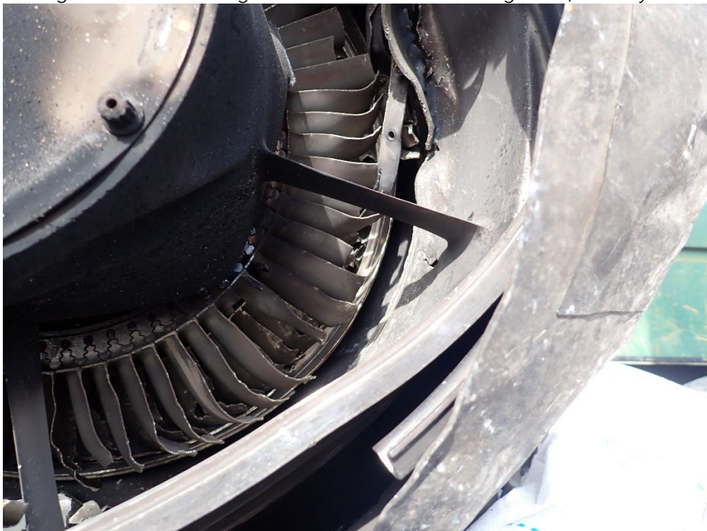
Figure 45: Engine Core 1 Third Stage LPT Blades with Rotational Bending Opposite Direction of Rotation (Courtesy of Honeywell)
