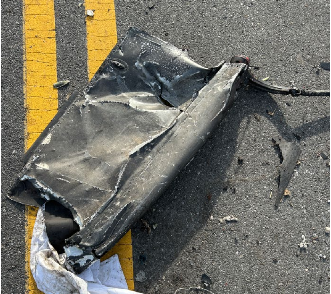
Figure 12: Inboard Portion of Left-hand Elevator
