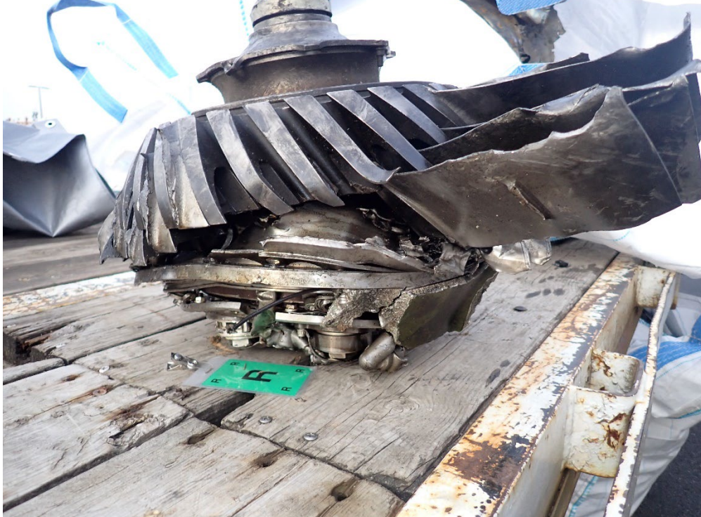
Figure 53: Fan Assembly 1 Side View of Disk and Blade (Courtesy of Honeywell)
