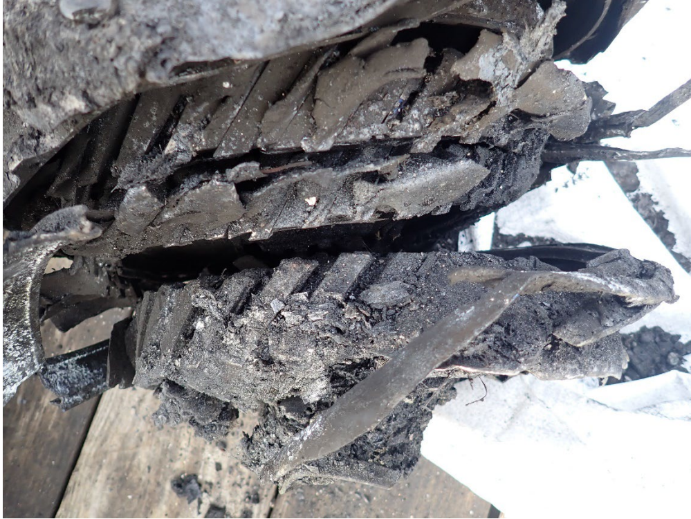
Figure 48: Engine Core 2 Compressor Section (Courtesy of Honeywell)
