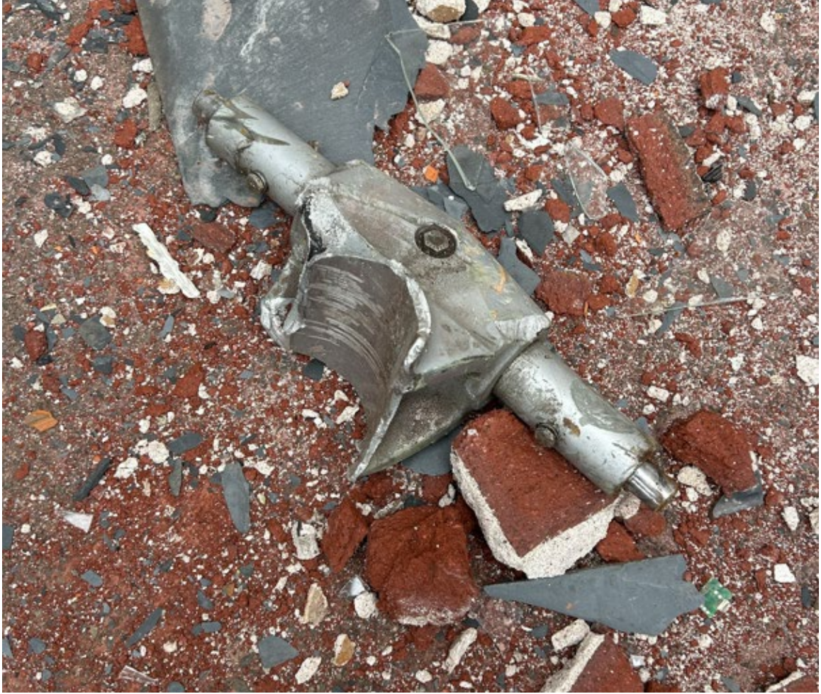
Figure 27: Top Piece of Nose Landing Gear Strut
