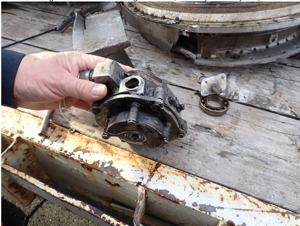
Figure 61: A Portion of an Engine Fuel Control (Courtesy of Honeywell)
