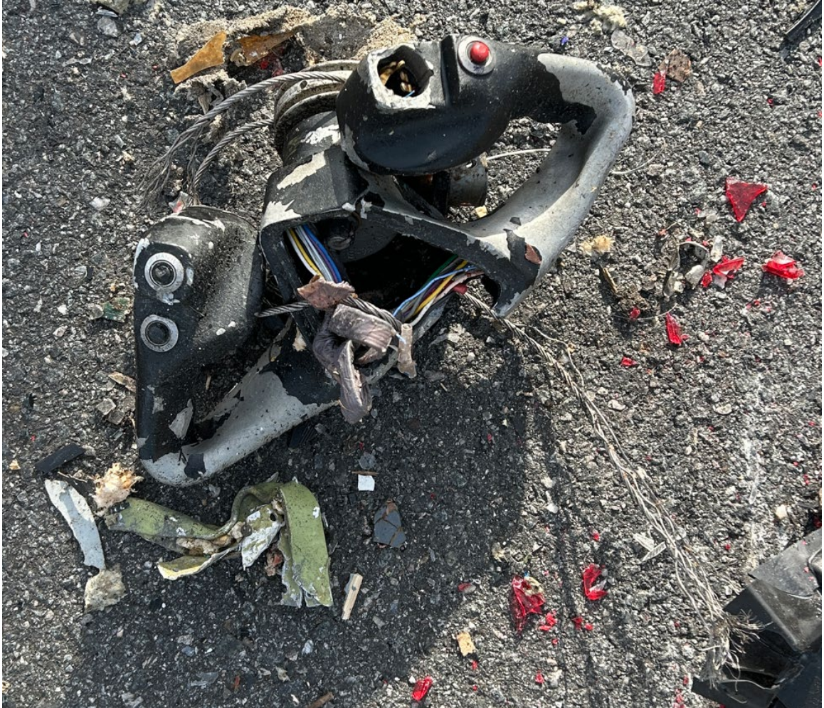
Figure 15: Co-pilot Control Wheel
