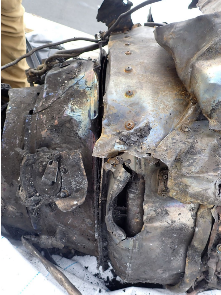
Figure 49: Engine Core 2 Compressor Plenum and Exposed Diffuser and Combustor Liner (Courtesy of Honeywell)
