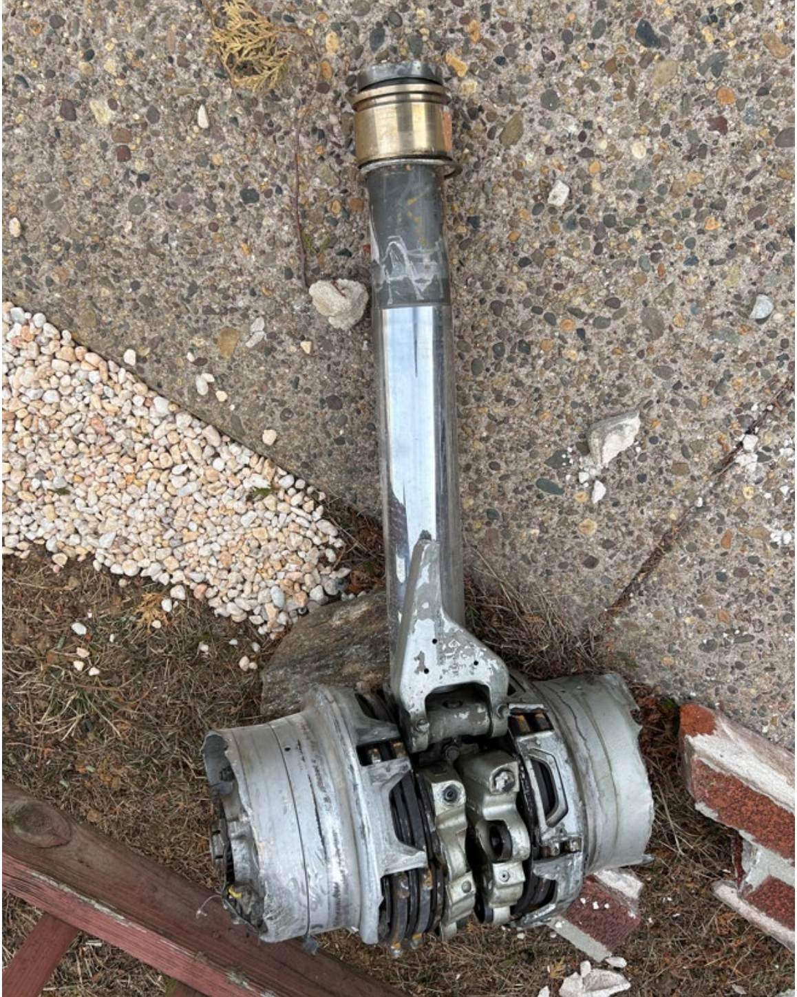
Figure 20: Right-hand Main Landing Gear Strut Piston
