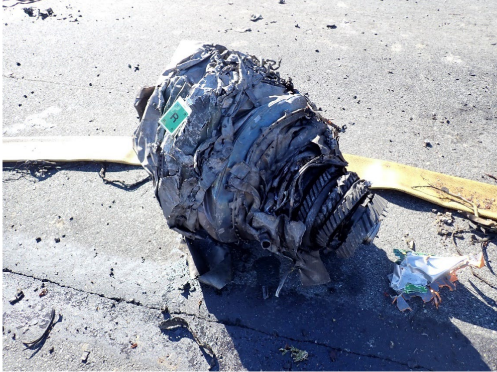
Figure 39: Engine Core 1 Near the Impact Crater and Later Identified as the Left Engine (Courtesy of Honeywell)
