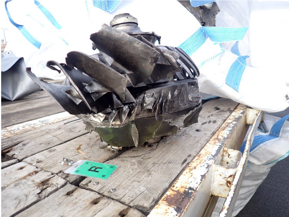
Figure 56: Fan Assembly 1 Side View of Blades and Some Stator Vanes (Courtesy of Honeywell)
