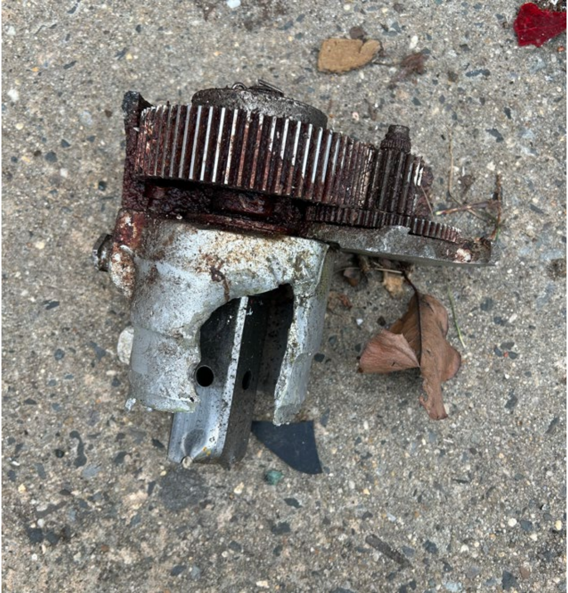
Figure 29: Nose Wheel Steering Servo
