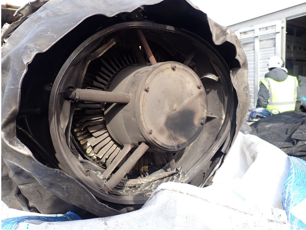
Figure 44: Engine Core 1 Third Stage LPT with View of Second Stage LPT (Courtesy of Honeywell)
