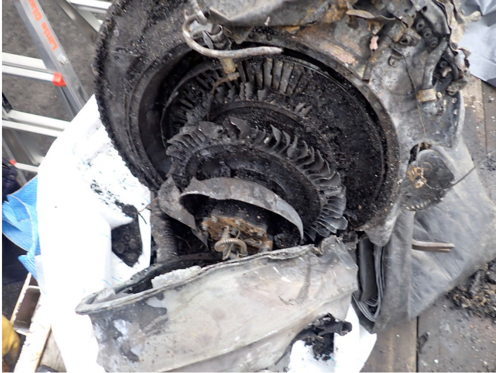
Figure 50: Engine Core 2 LPT Section and Displaced Rear Bearing Support Housing (Courtesy of Honeywell)
