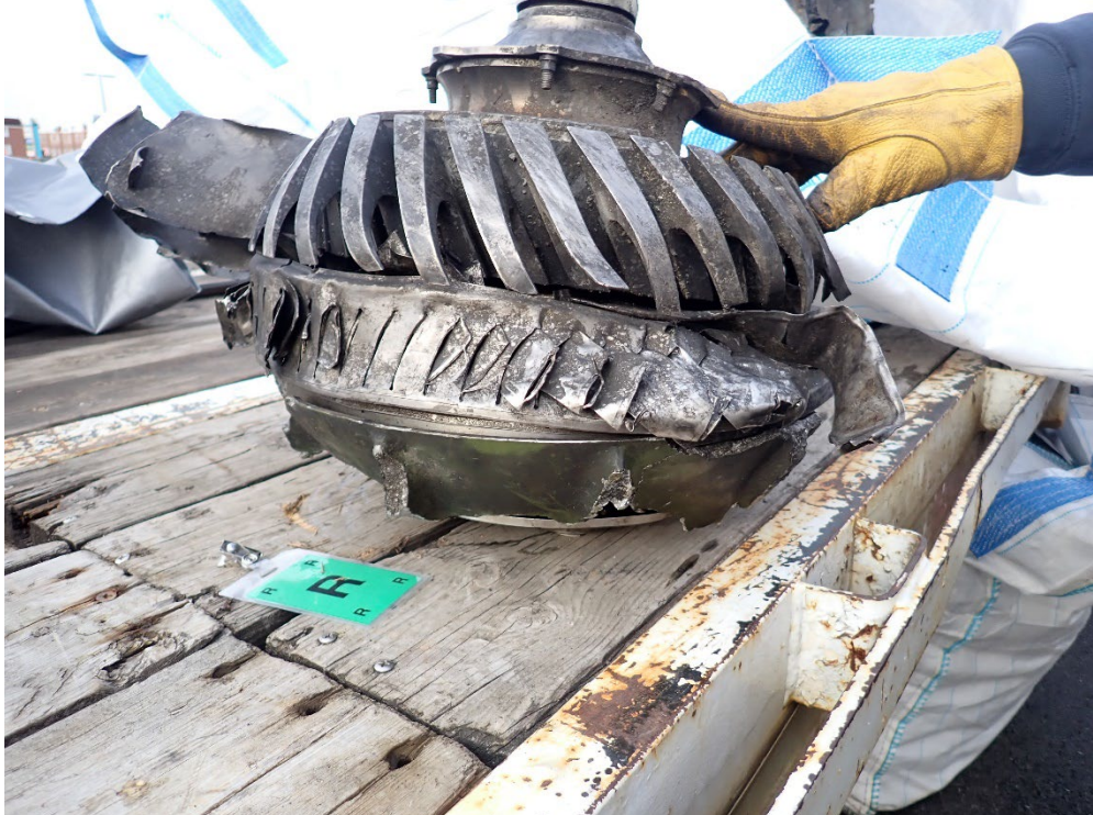
Figure 55: Fan Assembly 1 Damaged Disk and Portion of Compressor Inlet Stator Ring (Courtesy of Honeywell)
