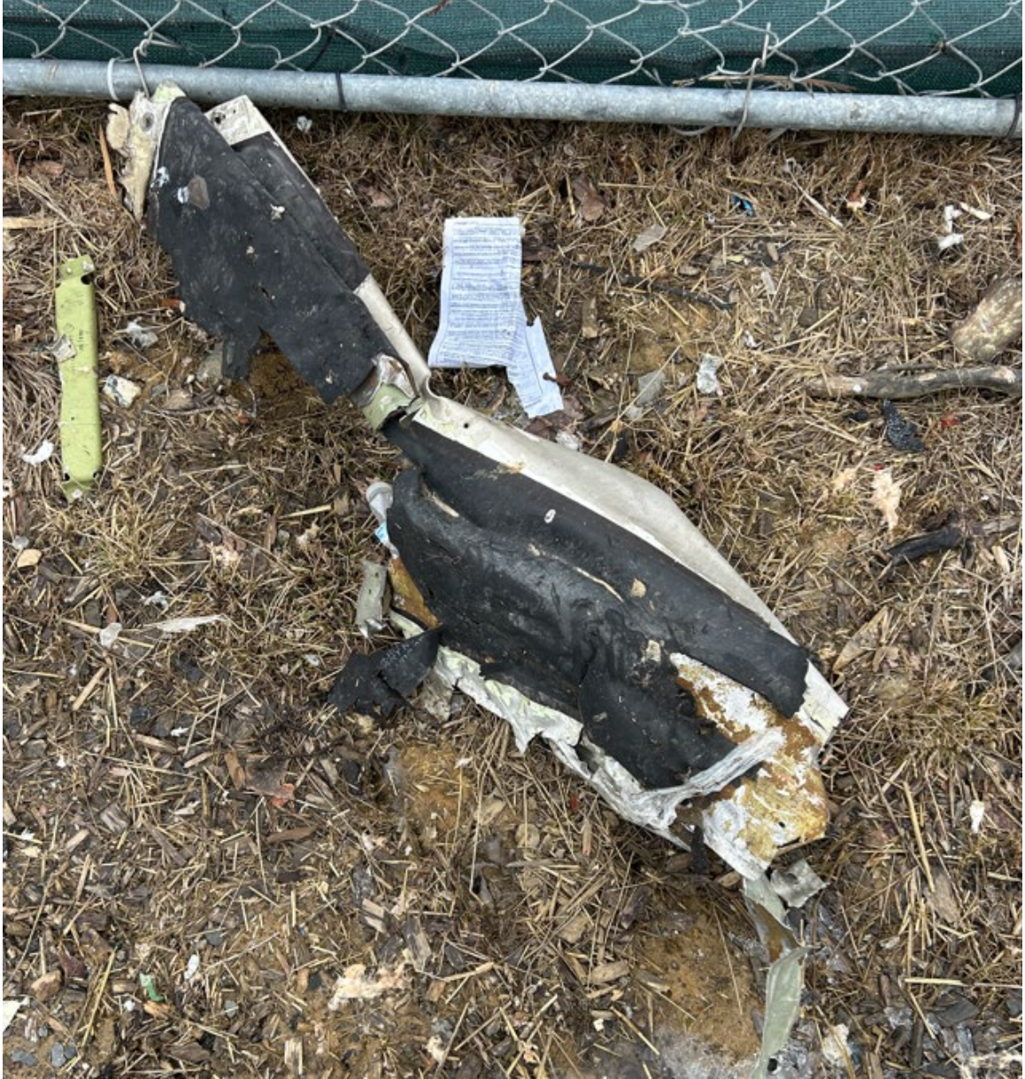
Figure 18: Portion of Horizontal Stabilizer Leading Edge
