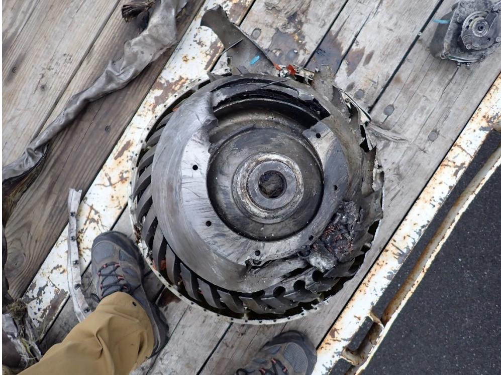
Figure 58: Fan Assembly 2 (Courtesy of Honeywell)
