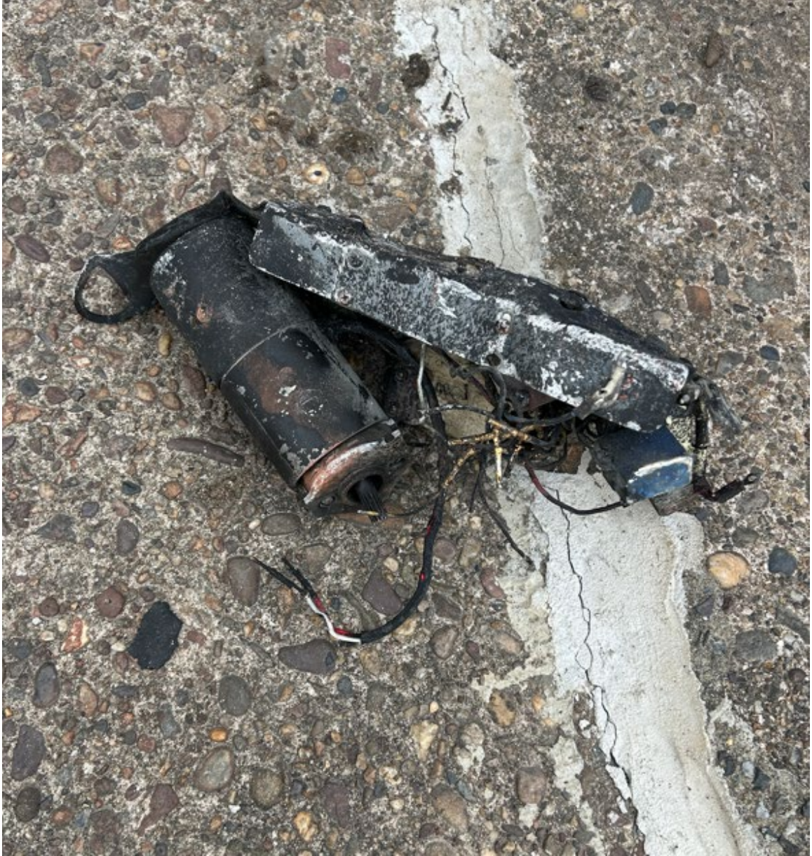
Figure 26: Pitch Trim Actuator Motor
