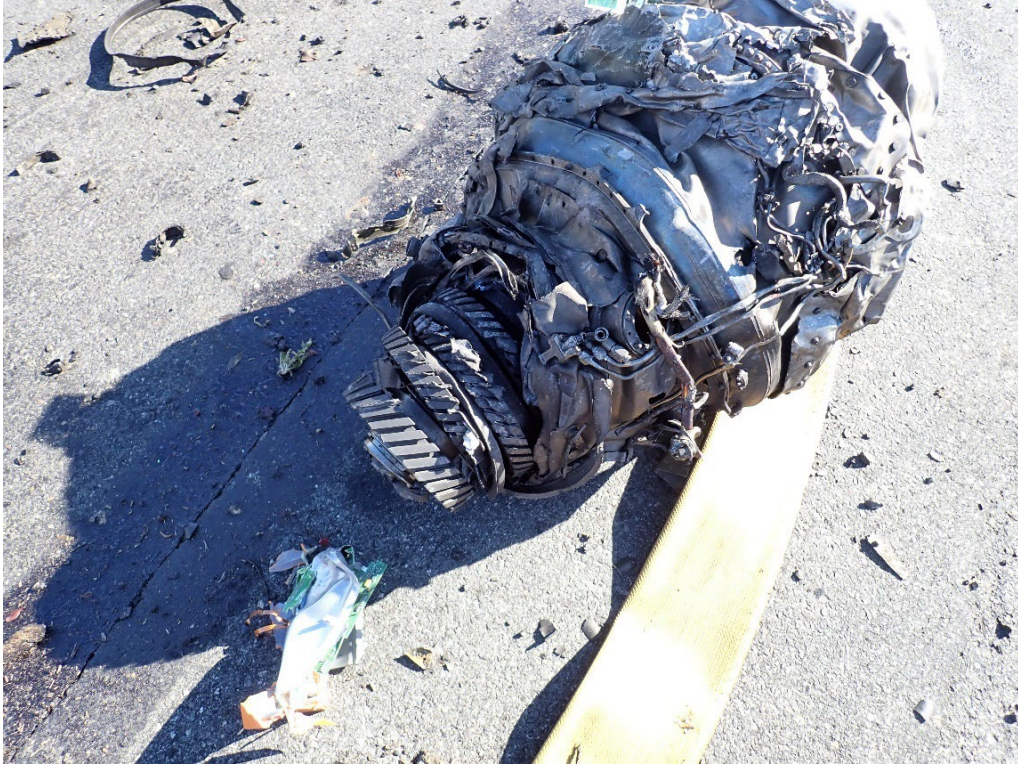
Figure 40: Engine Core 1 Near the Impact Crater and Later Identified as the Left Engine (Courtesy of Honeywell)
