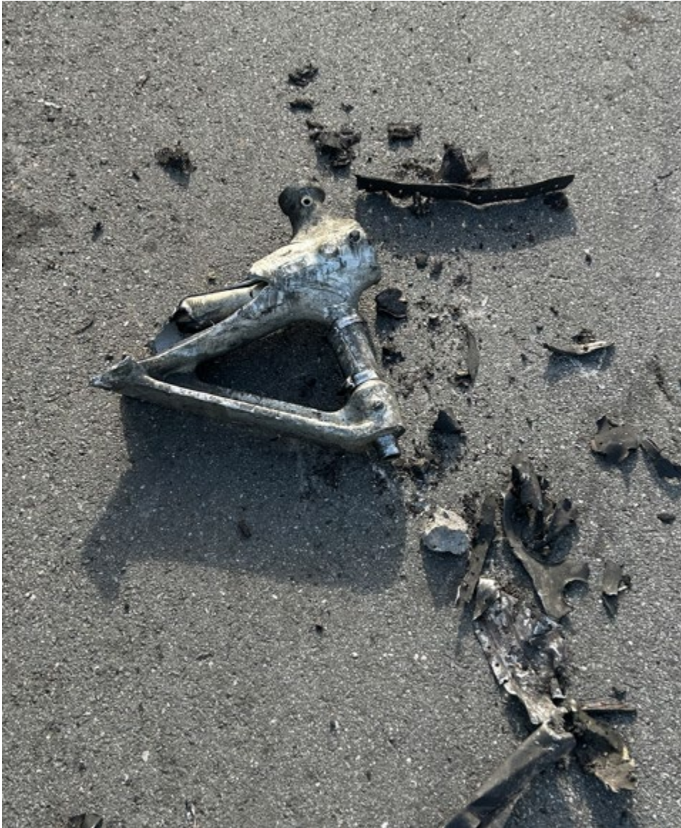
Figure 2: Right-hand Main Landing Gear Fitting
