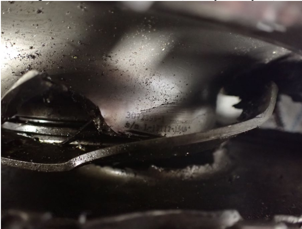
Figure 63: Left Engine First Stage Compressor Disc Part Number and Serial Number (Courtesy of Honeywell)
