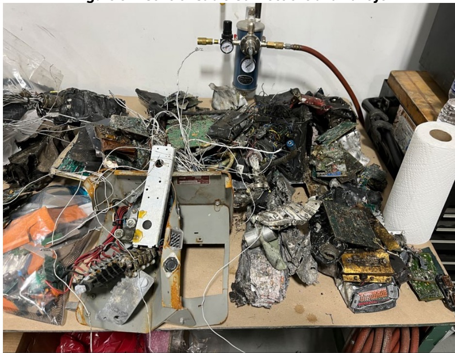
Figure 52: Circuit Breaker Panels and Miscellaneous Electronic Equipment
