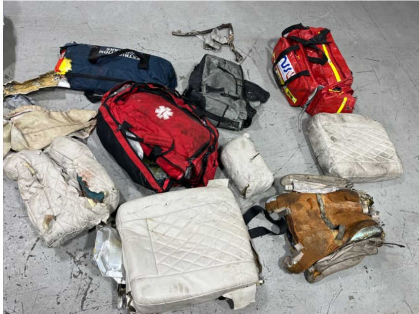
Figure 47: Interior Seating and Medical Equipment Absent of Soot
