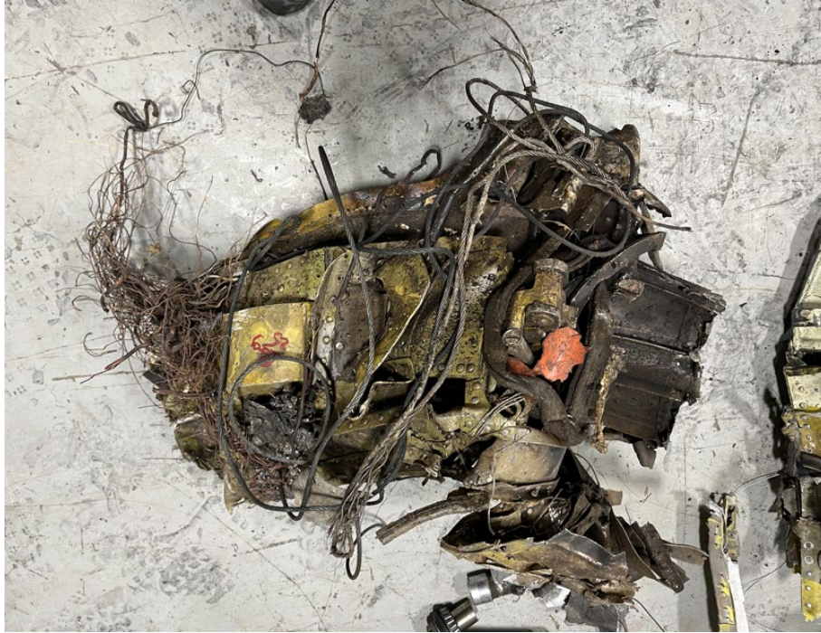
Figure 55: Lower Tail Section with Attached Control Cables
