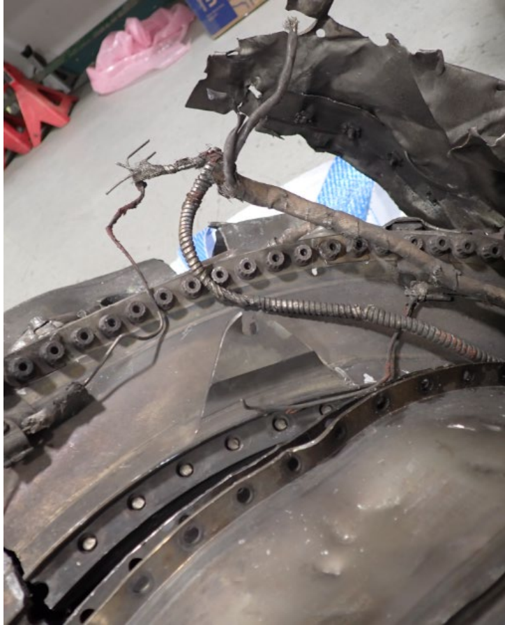
Figure 64: Left Aft Engine Mount(Courtesy of Honeywell)
