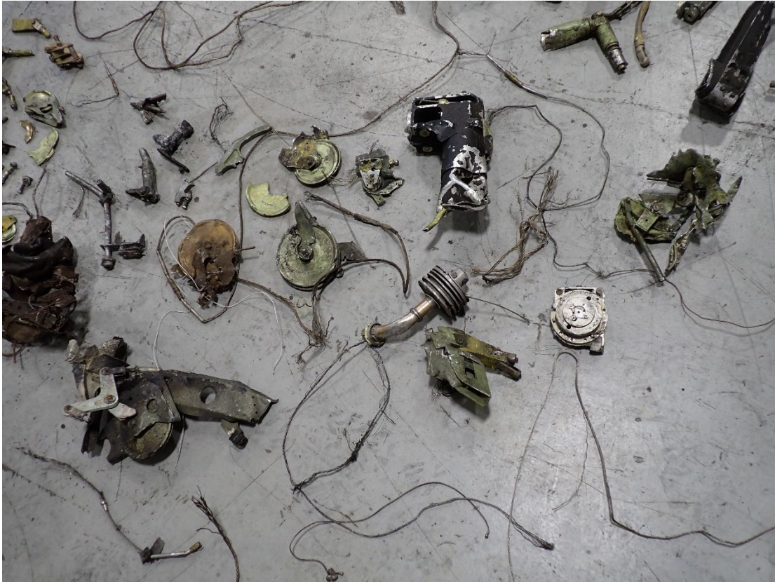
Figure 51: Control Cable Connections and Pulleys
