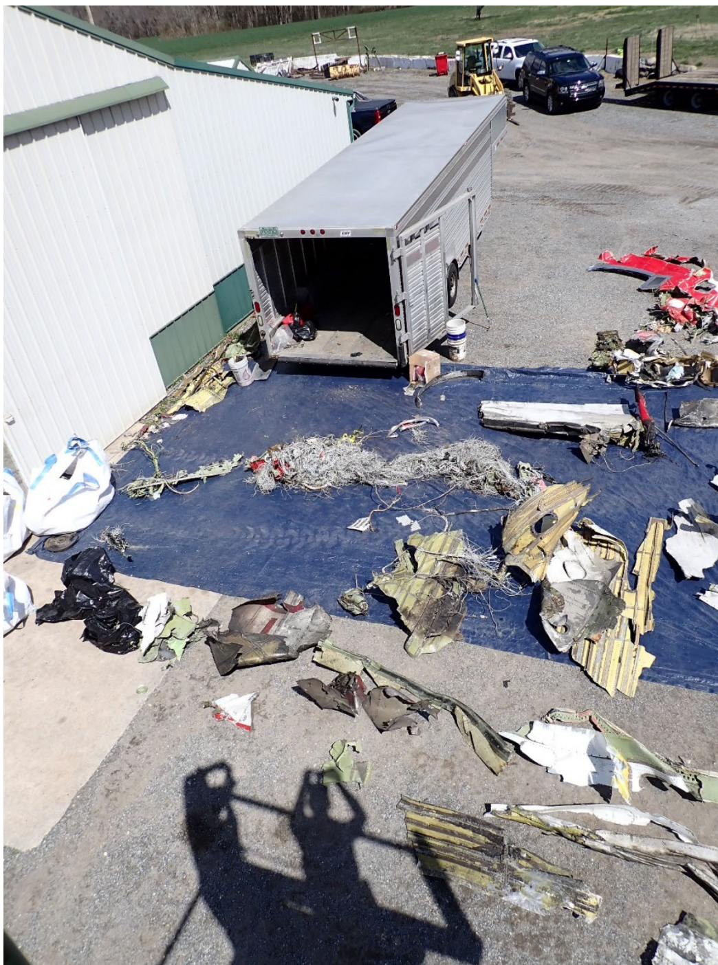
Figure 61: Layout of Trailer Components and Large Wiring Bundle
