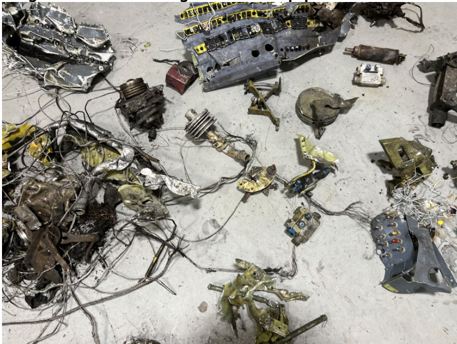
Figure 48: Control Pulleys, Circuit Breakers, and Miscellaneous Switch Panel
