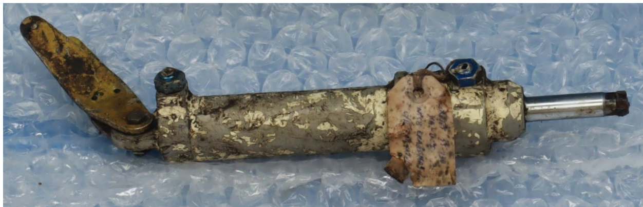
Figure 1. LH flap actuator as received at the NTSB Materials Laboratory.
