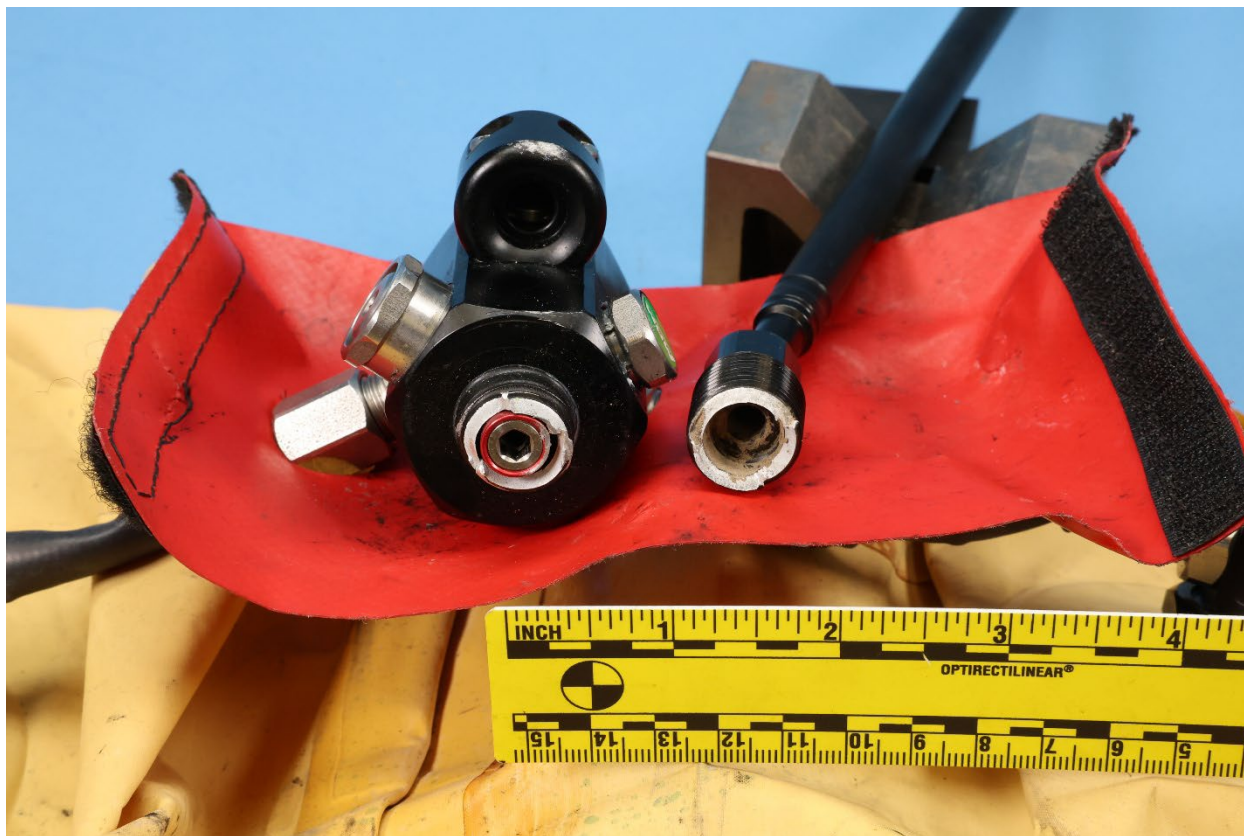
Figure 18. Emergency life raft inflation valve as received at the NTSB Materials Laboratory.
