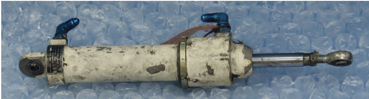
Figure 7. RH flap actuator as received at the NTSB Materials Laboratory.
