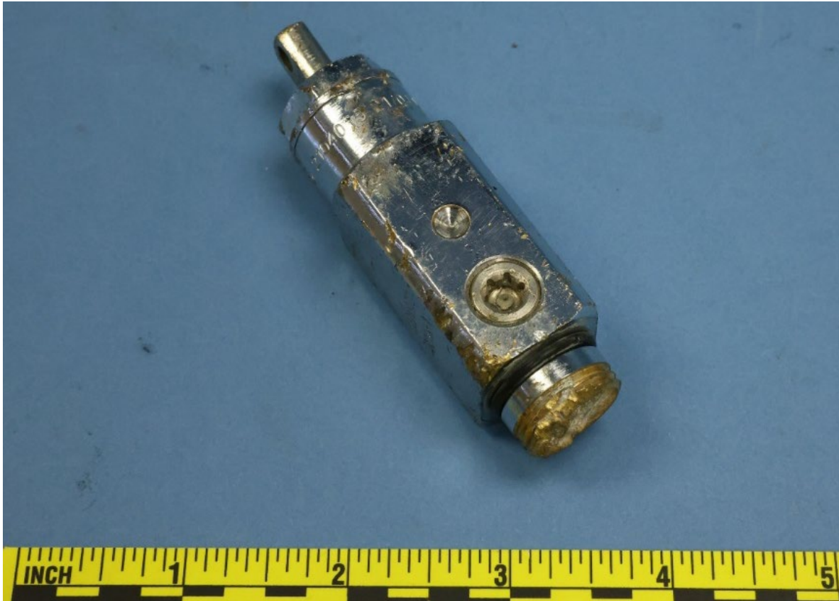
Figure 14. Oxygen medical pin index valve as received at the NTSB Materials Laboratory.
