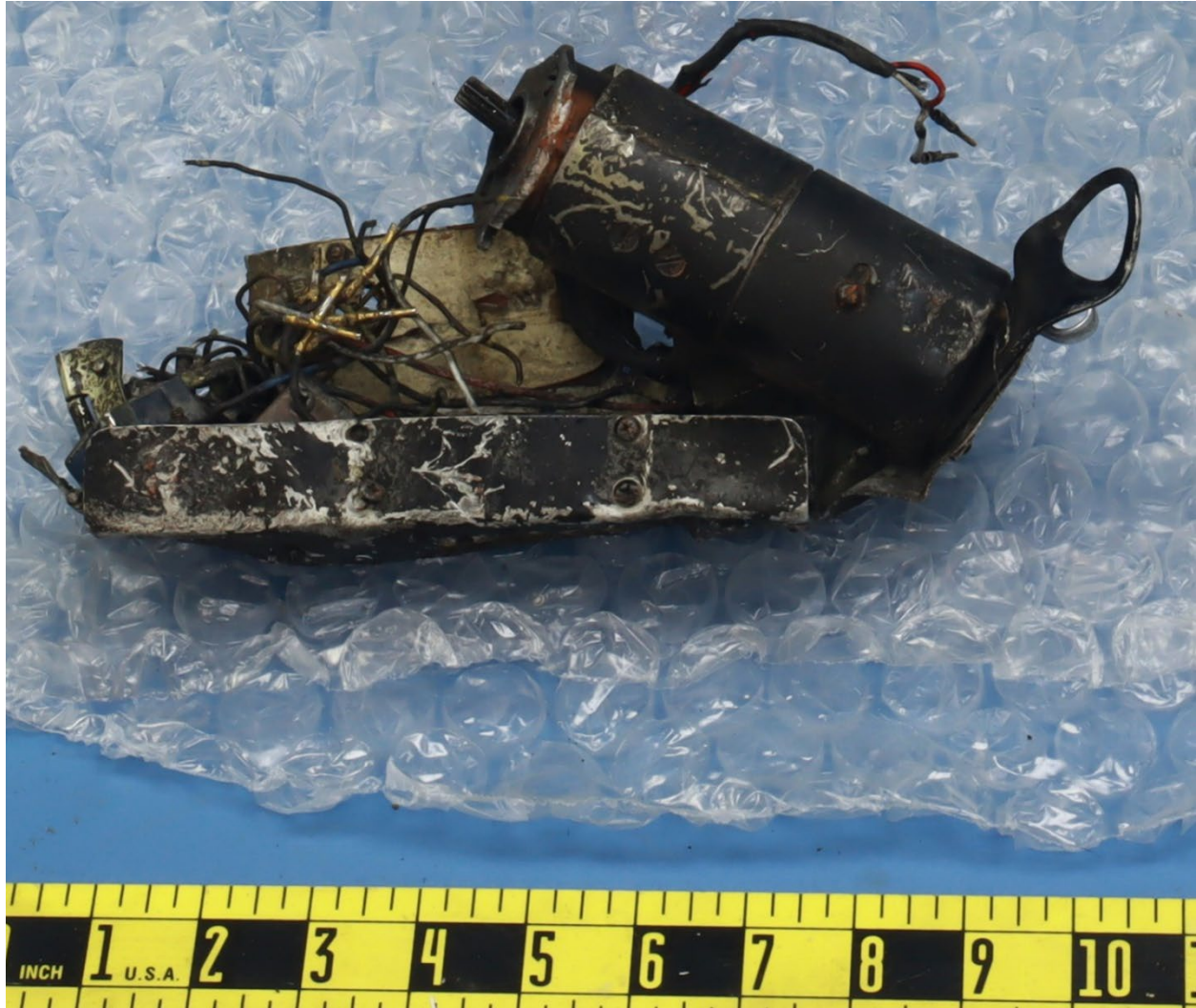
Figure 11. Pitch trim motor as received at the NTSB Materials Laboratory.
