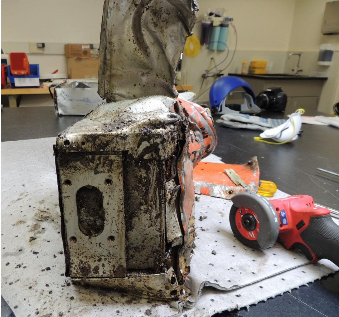
Figure 5. Damaged exterior of CVR being removed using cutting tools.
