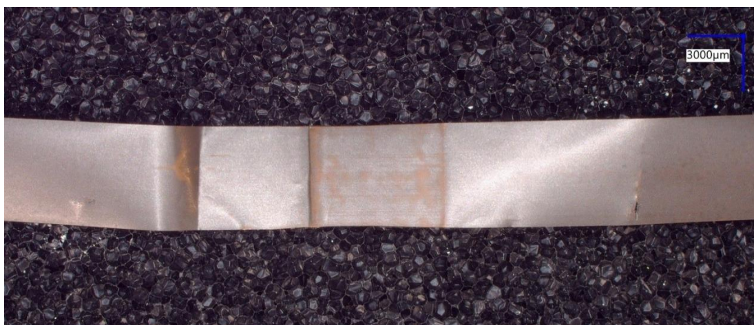
Figure 19. First pre-existing splice viewed from the non-data side of the tape.
