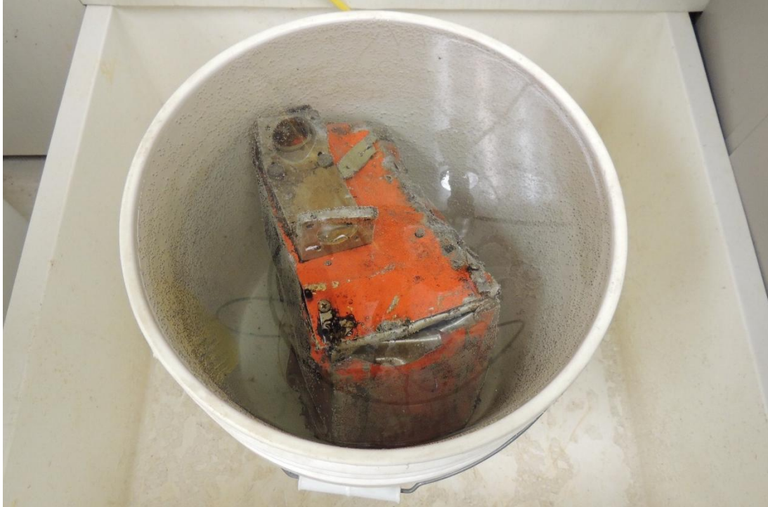
Figure 2. Damaged exterior of CVR during initial soaking.
