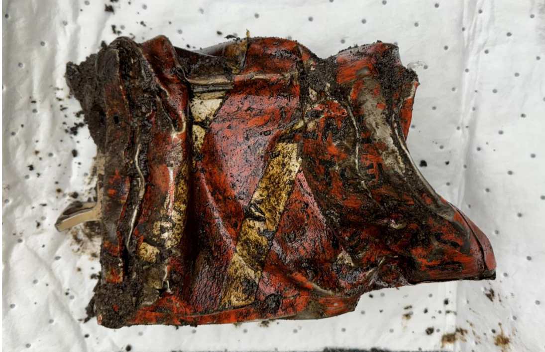
Figure 1. Damaged exterior view of CVR prior to initial soaking.
