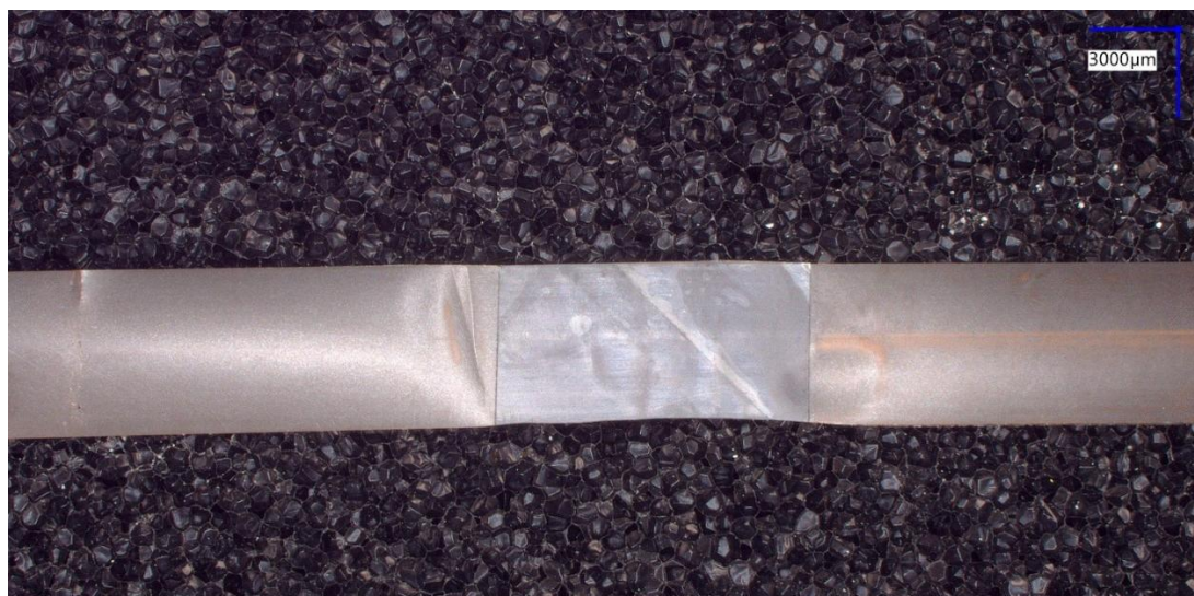
Figure 22. Second pre-existing splice viewed from the non-data side of the tape.
