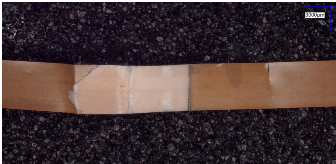
Figure 18. First pre-existing splice viewed from the data side of the tape.
