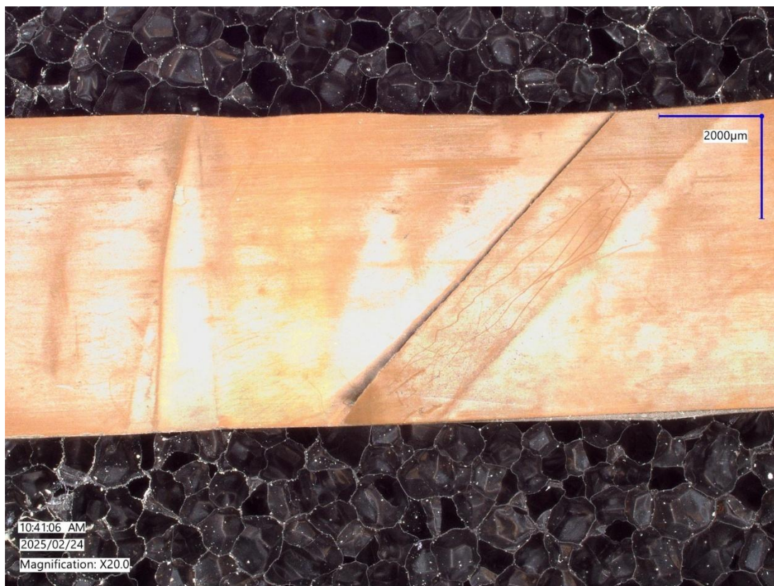
Figure 21. Second pre-existing splice viewed from the data side of the tape (closeup).
