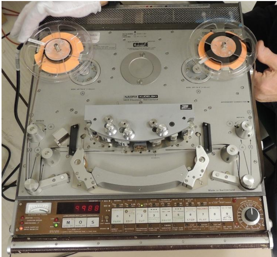
Figure 17. Tape being hand-wound in free-spooling mode after drying to take up slack.
