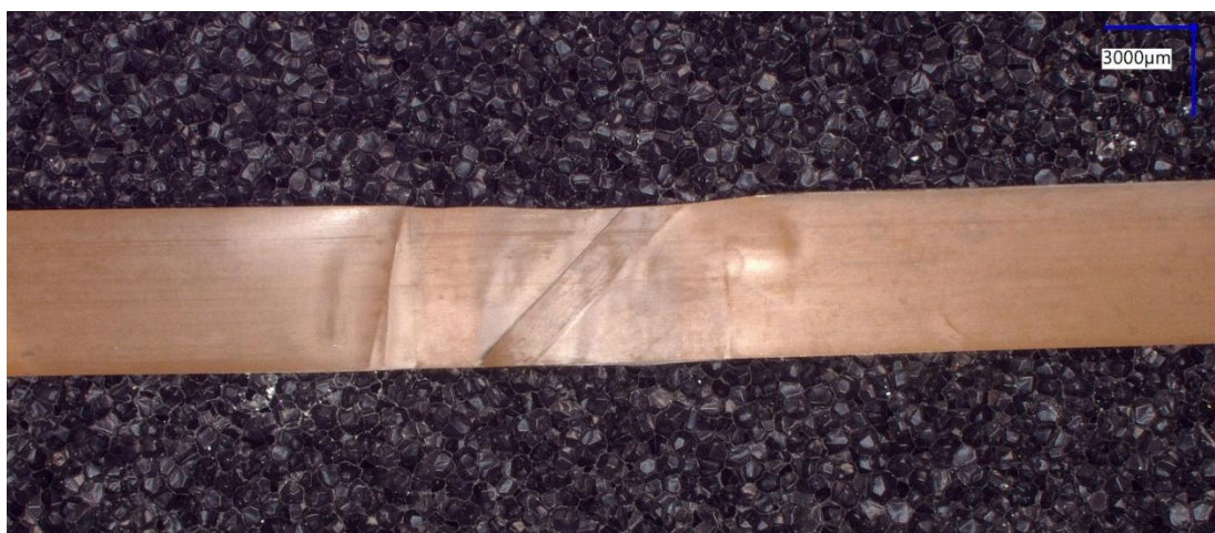
Figure 20. Second pre-existing splice viewed from the data side of the tape.
