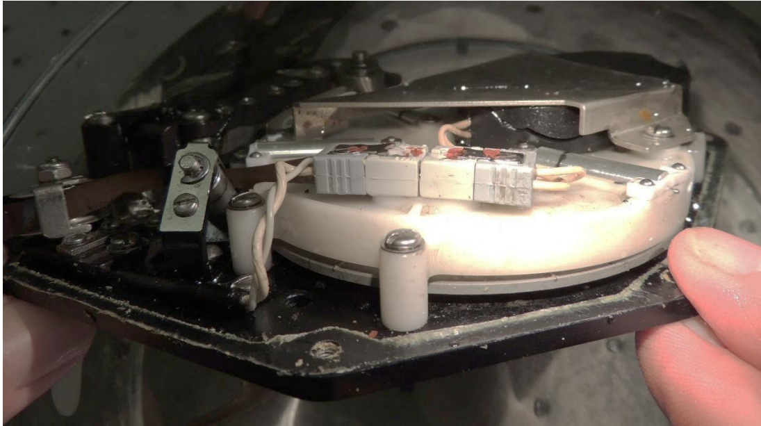
Figure 8. Transport mechanism showing internal damage due to impact forces.
