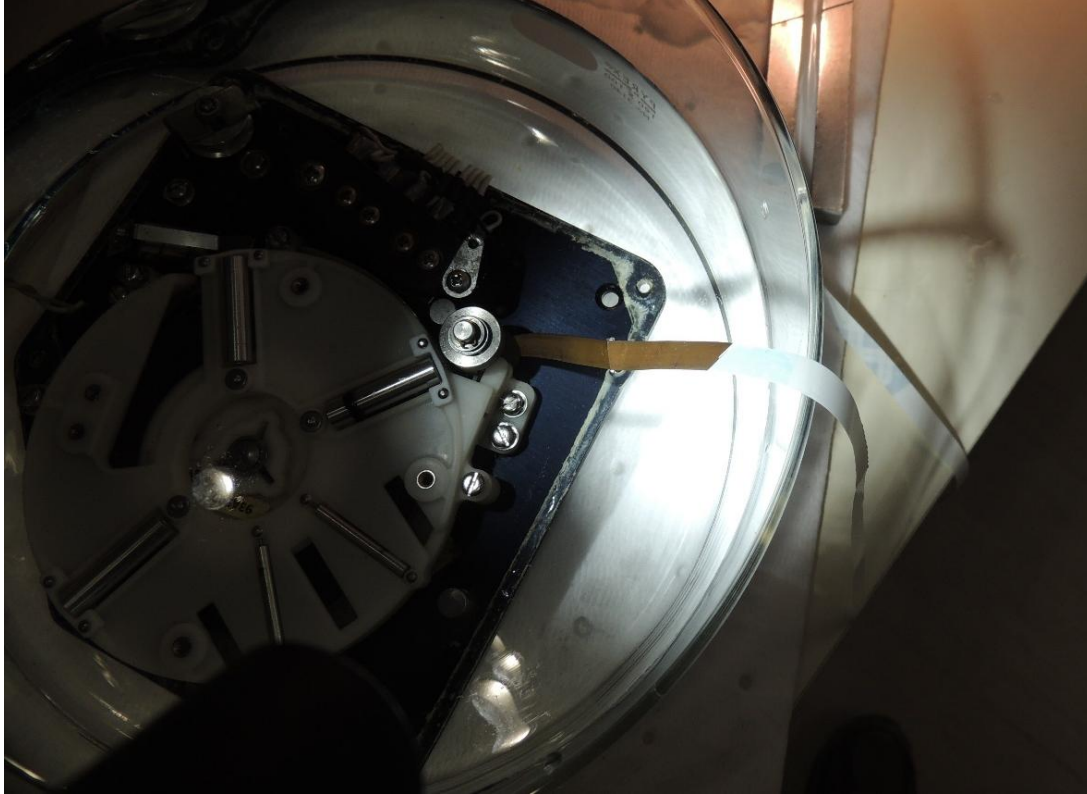
Figure 12. Leader tape spliced to outer end CVR tape after initial cutting and splicing.
