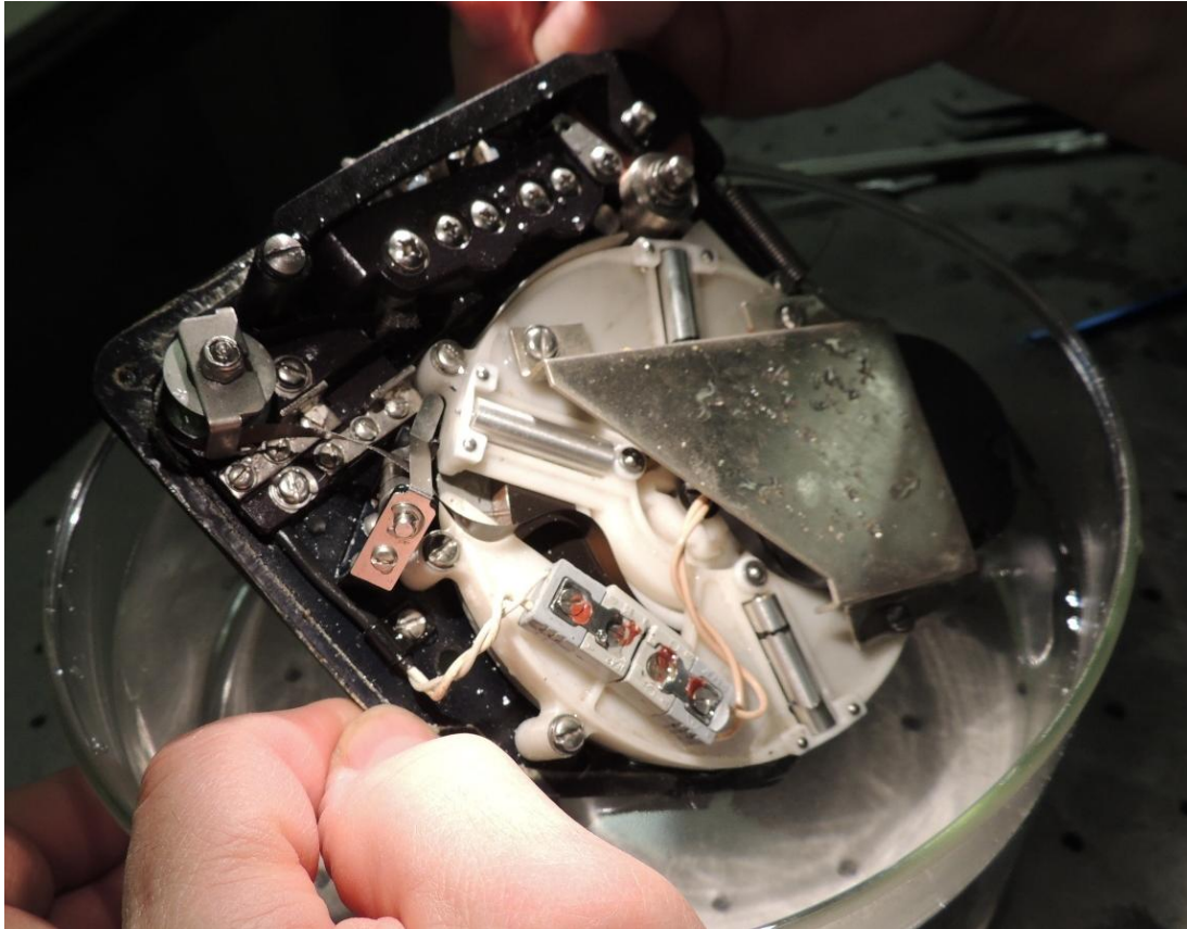
Figure 6. Transport mechanism removed from the damaged A-100A (s/n 25033).
