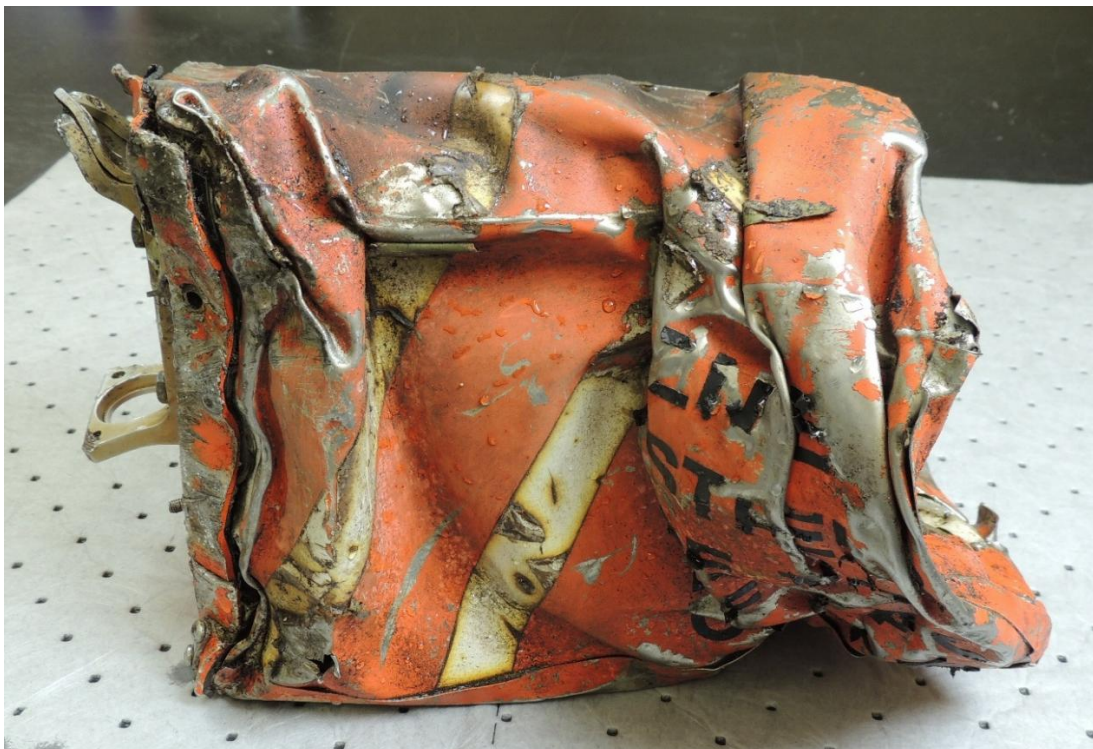
Figure 3. Damaged exterior view of CVR after initial soaking.
