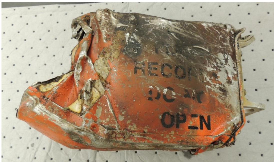
Figure 4. Damaged exterior of CVR after initial soaking.
