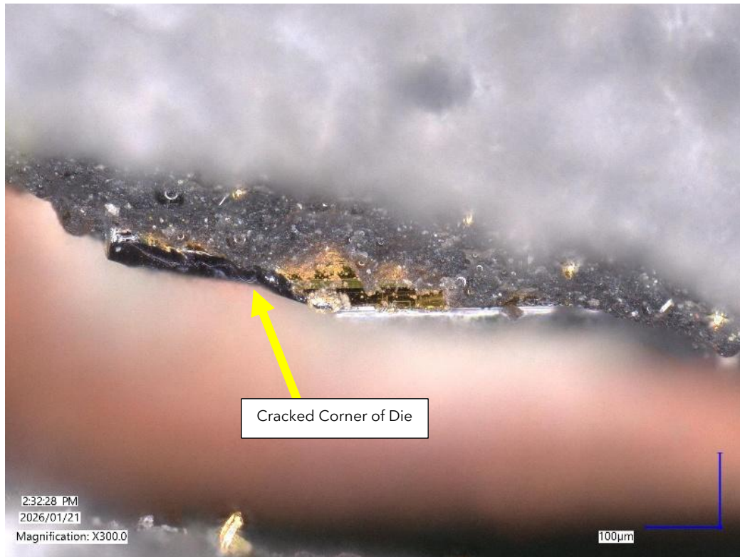
Figure 5. A 300x magnification image of the area circled in yellow in Figure 4. The yellow arrow annotates a cracked corner of the chip's die.
