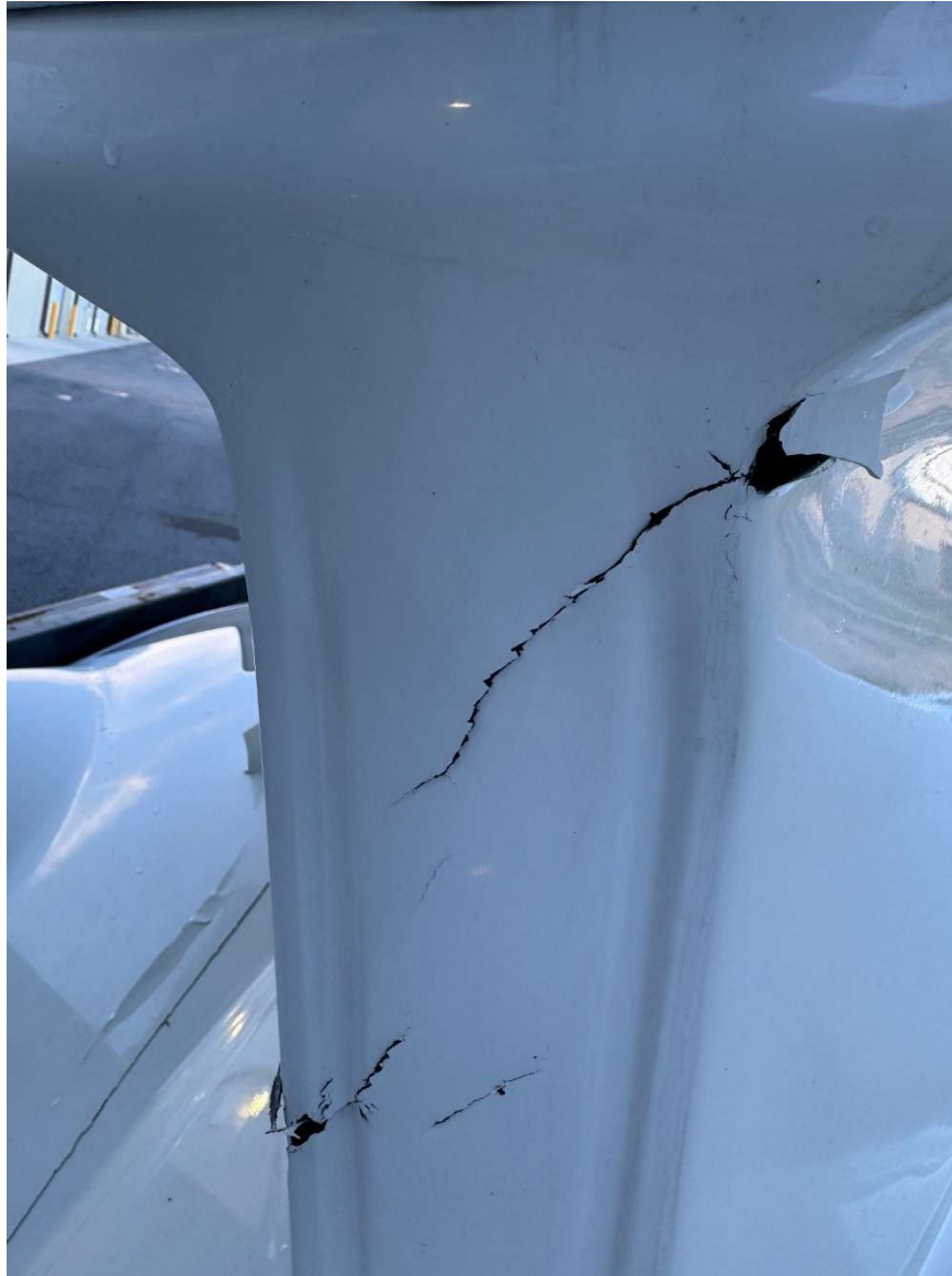
Photograph 4 - Close up of Damage to Engine Pylon (Courtesy of Owner)
