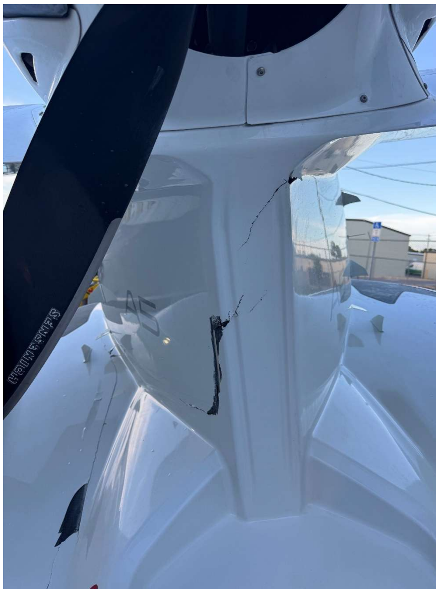
Photograph 3 - Cracking Damage to Engine Pylon (Courtesy of Owner)
