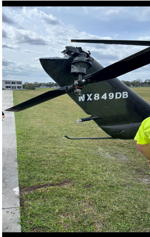
Photograph 1 - View of damaged tail rotor. (Courtesy of FAA)
