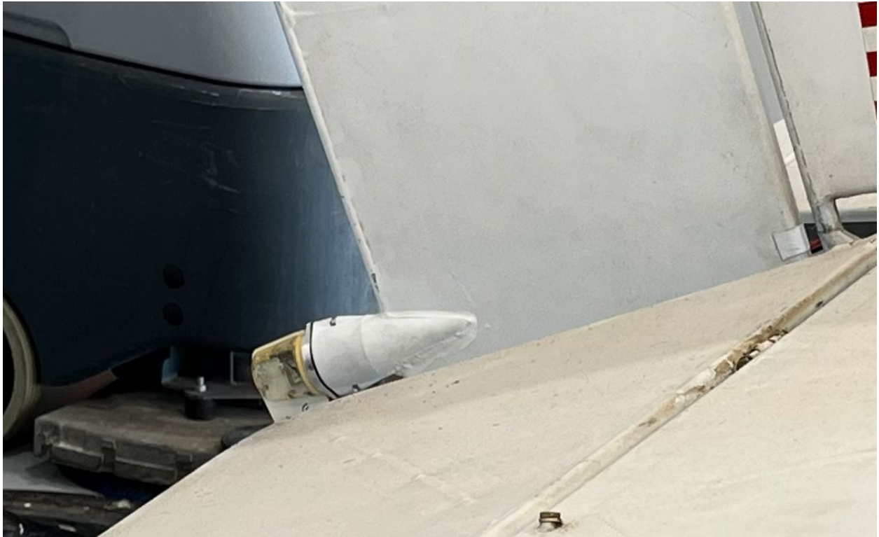
Figure 11: UA Avionics ADSB System and Fixture/Fairing (Photo Courtesy of FAA)
