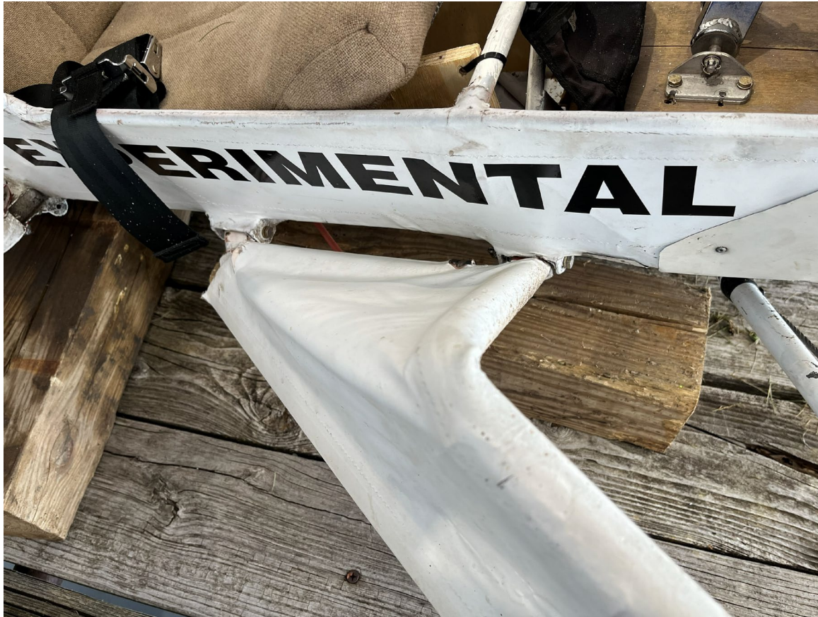
Photograph 4 - Right Landing Gear Collapse, Brackets Still Attached (Courtesy of FAA)
