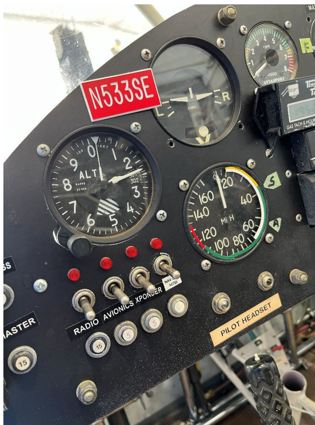
Photograph 5 - N533SE Interior Showing ADS-B and Airspeed Markings (Courtesy of FAA)
