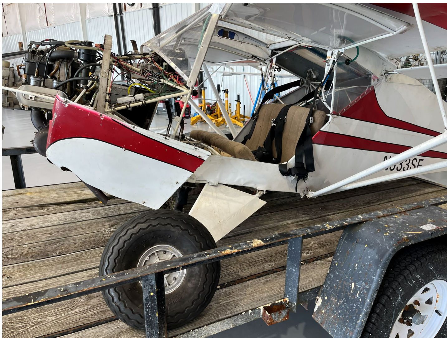
Photograph 2 - Left Forward Landing Gear Bracket Torn from Frame (Courtesy of FAA)
