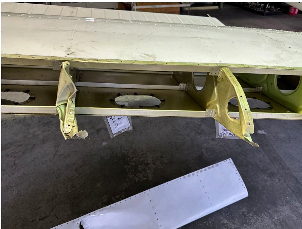
Photograph 2 - Right Wing Rib Damage (Courtesy of Operator)
