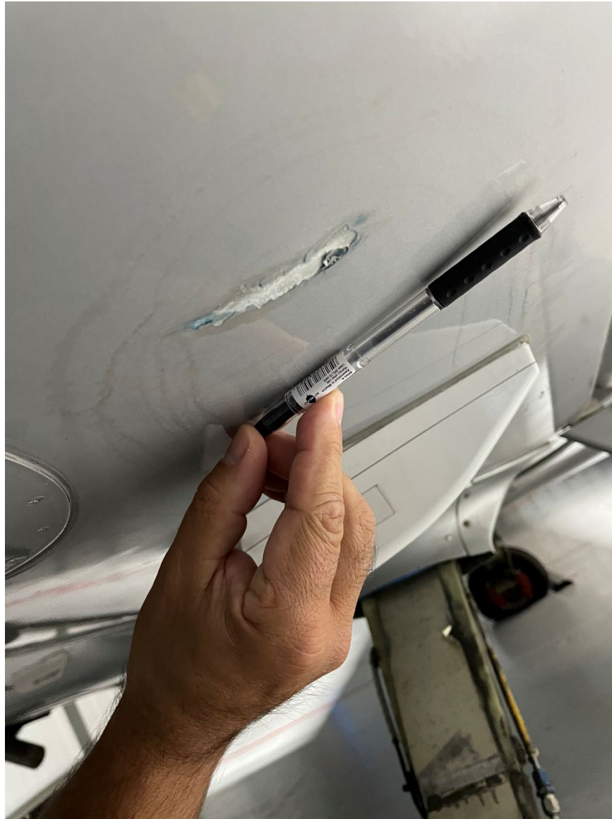
Photograph 2 - Left Fuel Cell Breach (Courtesy of FAA)
