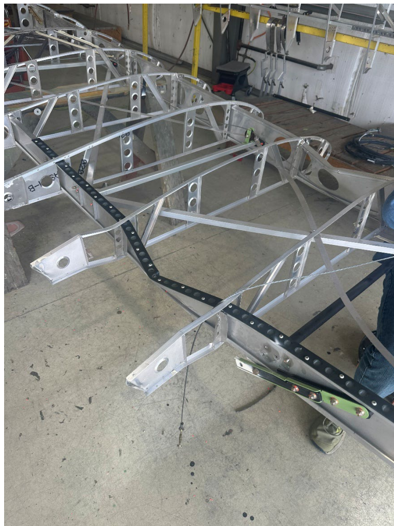
Photograph 3 - Damage to Aircraft Right Wing Spars (Courtesy of FAA/Legend Aircraft)
