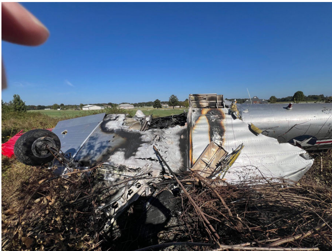
Photograph 3 - Bottom surface of wings showing fire damage (Courtesy of FAA)
