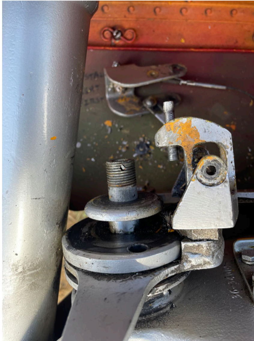
Photograph 5 - Upper half of locking pin frozen in place in upper casting (Courtesy of FAA)
