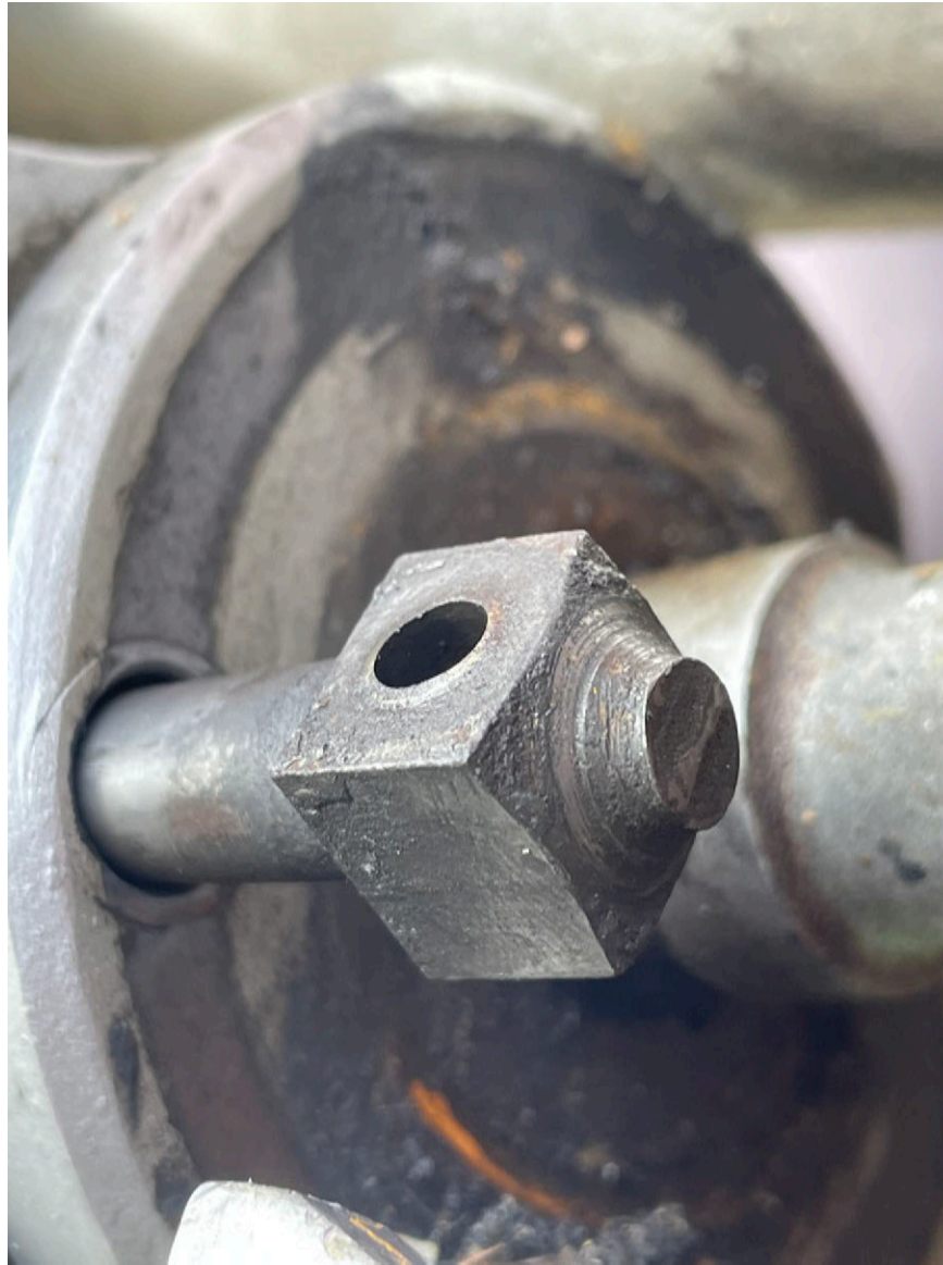
Photograph 4 - Lower half of tailwheel locking pin showing fracture surface (Courtesy of FAA)
