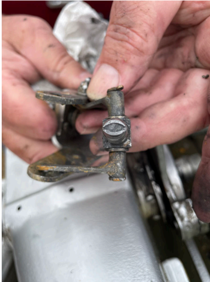
Photograph 6 - Bottom of lower locking pin showing wear (Courtesy of FAA)
