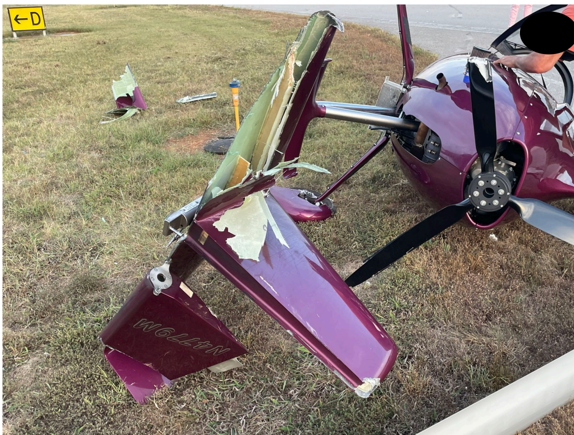
Photograph 3 - Rudder/Horizontal Stabilizer Damage (Courtesy of FAA)
