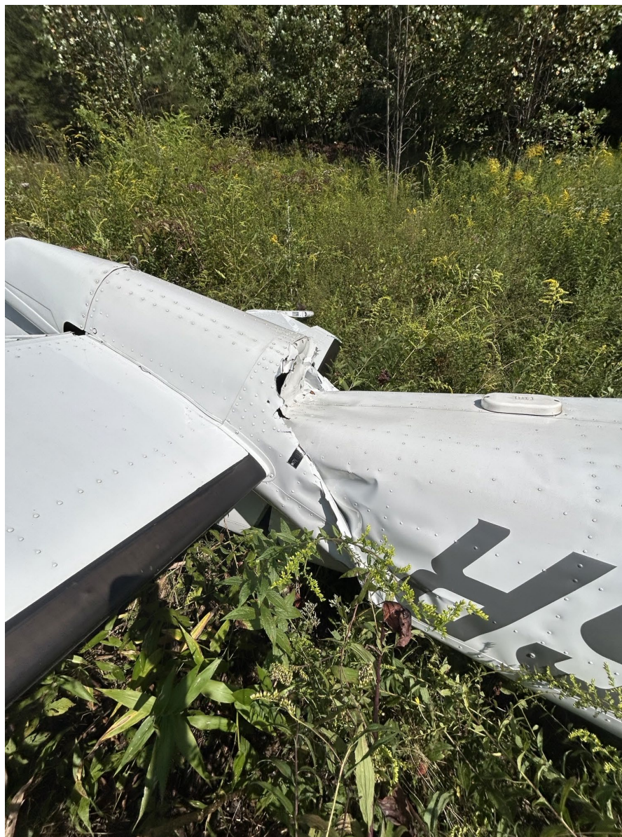
Photograph 3 - damaged tail section (Courtesy of Fire Department)
