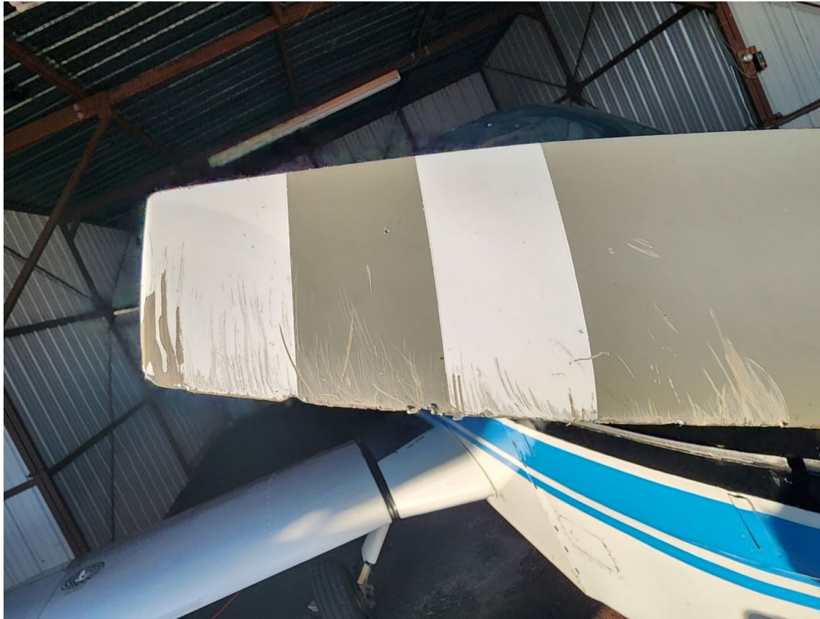
Photograph 1 - View Showing Damage to 1 Propeller Blade of N81317 (Courtesy of Pilot)
