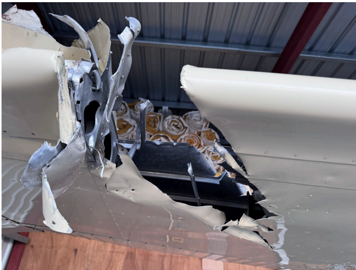
Photograph 3 - View of Damage to Outer Right Wing of N2383X (Courtesy of Pilot)
