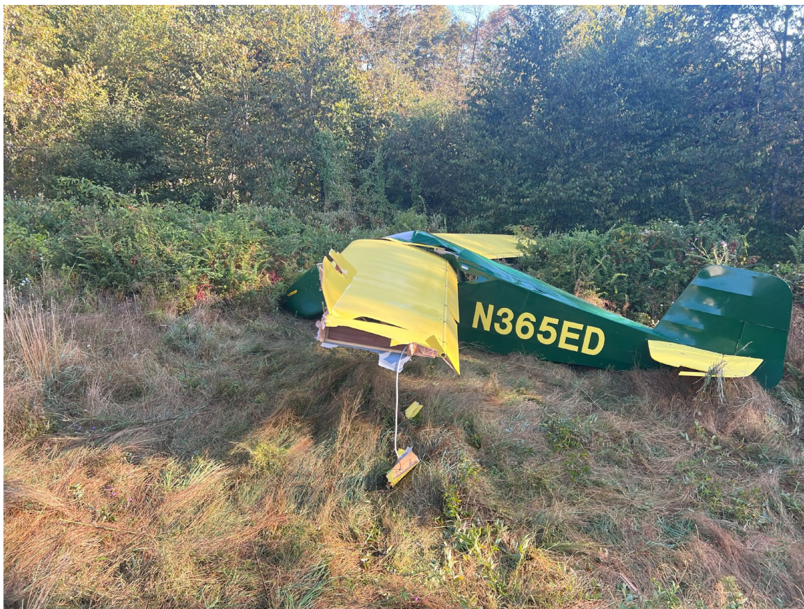
Photograph 2 - Skin separations and spar fractures noted to left wing (Courtesy of FAA)
